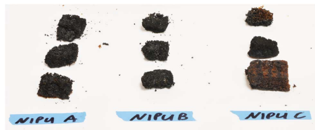
Fig. 7 Remnants of NIPU foam samples after burn testing.
