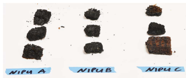
Fig. 7 Remnants of NIPU foam samples after burn testing.
