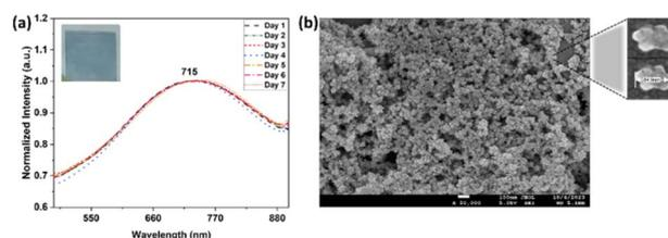
Fig. 2 (a) UV-absorption spectra of APTES-associated gold nanostar substrate on seven different days with a photograph of the fabricated substrate (inset), (b) FESEM image of the nanostar substrate.
