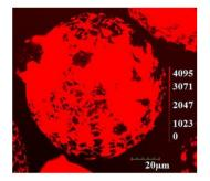
Fig. 7 3D reconstruction picture of a single FCC catalyst particle with adsorbed rhodamine B.
