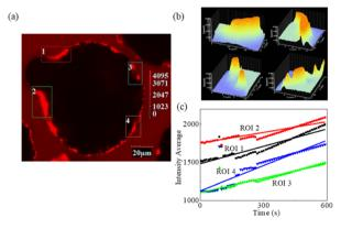
Fig. 5 Changes in the fluorescence distribution catalyst particles upon the adsorption of rhodamine B at  $10^{-4}$  mol L<sup>-1</sup> with time: (a) different regions of the catalyst particles; (b) fluorescence intensity of each pixel in the corresponding region of the catalyst particle after adsorbing rhodamine B; and (c) average fluorescence intensity variations in regions 1-4 with time.
