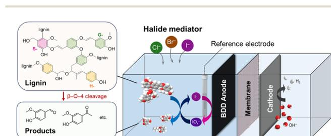
**Scheme 1** Schematic representation of the halide-mediated electrochemical depolymerization of lignin. The left panel illustrates the representative lignin structure comprising typical monolignol units (G, H, and S) and aromatic products formed *via*  $\beta$ -O-4 bond cleavage.
