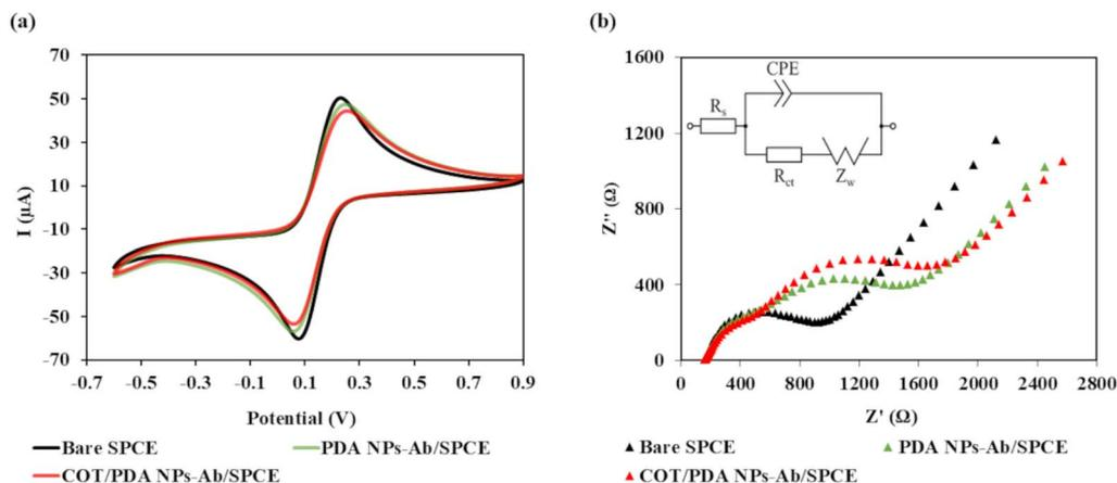
Fig. 2 Electrochemical characterization of the cotinine immunosensor: (a) CV and (b) EIS of bare SPCE, PDA NPs-Ab/SPCE, and COT/PDA NPs-Ab/SPCE in 5 mM  $[\text{Fe}(\text{CN})_6]^{3-/4-}$  with 0.1 M KCl.
