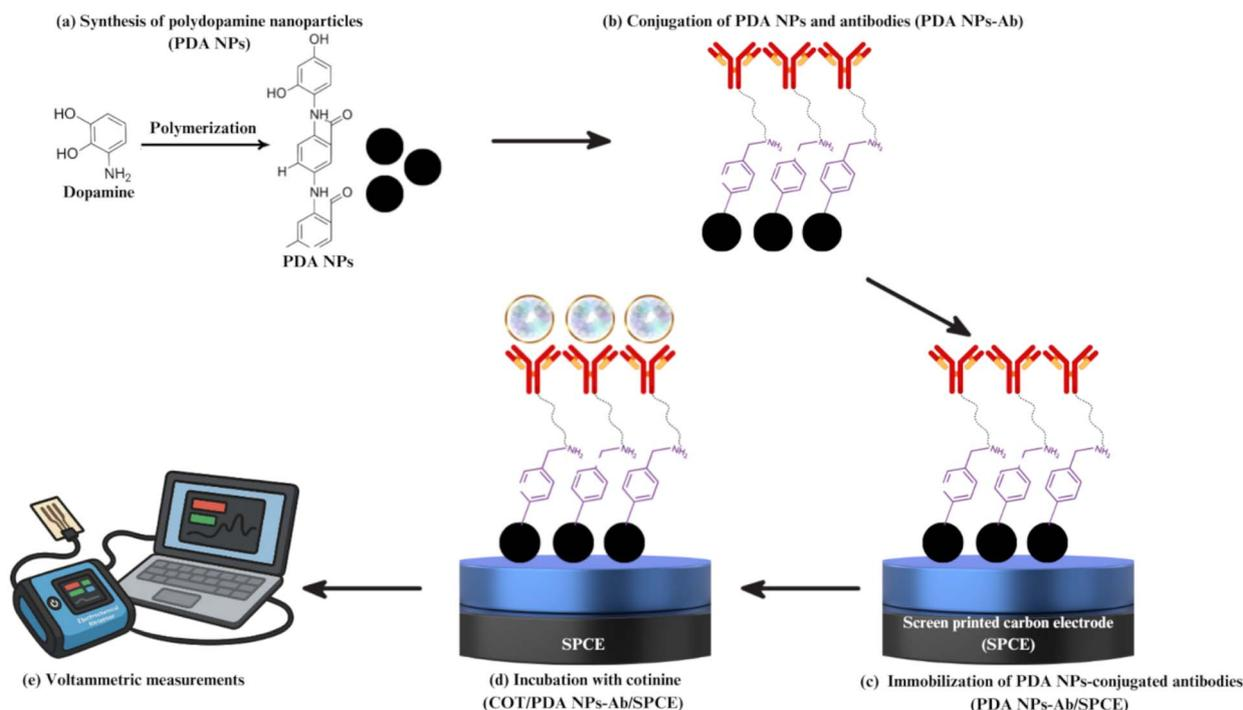
**Scheme 1** Schematic illustration of the fabrication and detection process of the PDA NP-based cotinine immunosensor. (a) Synthesis of PDA NPs via dopamine polymerization, (b) covalent conjugation of PDA NPs with anti-COT Ab using EDC–NHS chemistry, (c) immobilization of PDA NPs–Ab conjugates on SPCE, (d) specific binding of cotinine to PDA NPs–Ab/SPCE, (e) electrochemical detection of cotinine using voltammetric measurements.
