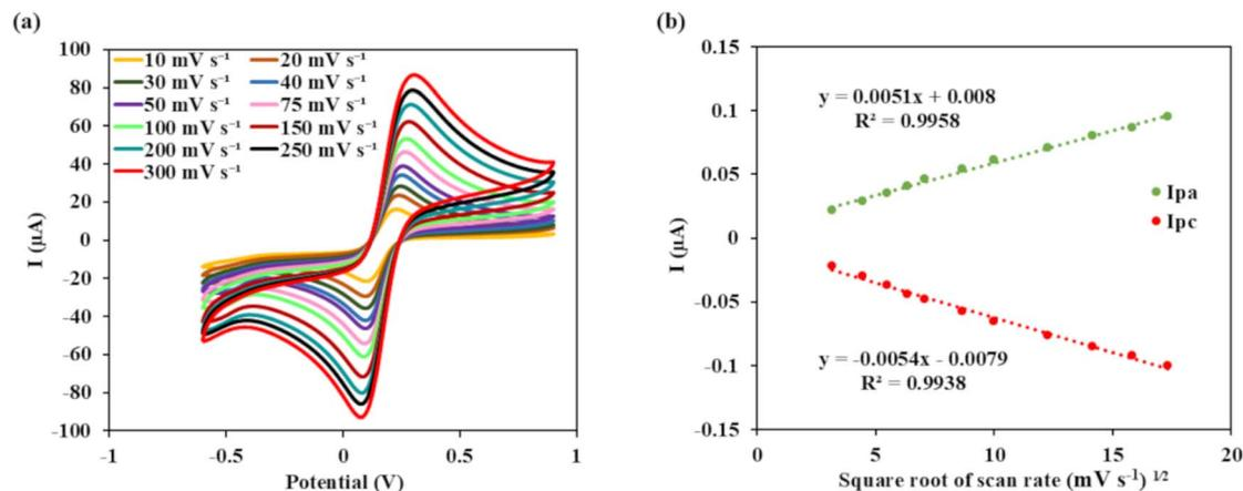
Fig. 3 Scan rate study of the PDA NPs-modified cotinine immunosensor: (a) CV at different scan rates ( $10\text{--}300 \text{ mV s}^{-1}$ ) and (b) Randles-Sevcik plot of anodic and cathodic peak current vs. square root of scan rate.
