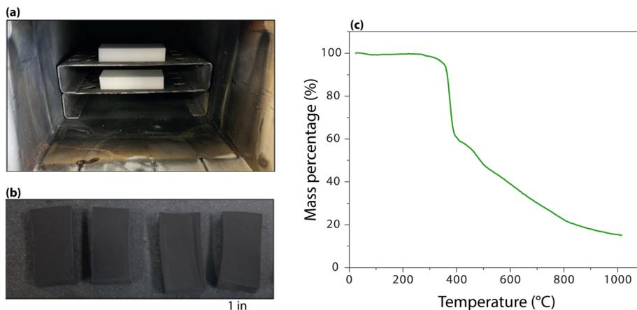
Fig. 3 (a) Picture of MeF loaded in the furnace, (b) picture of CF formed from carbonization, and (c) TGA of MeF showing mass loss with temperature in N<sub>2</sub>.
