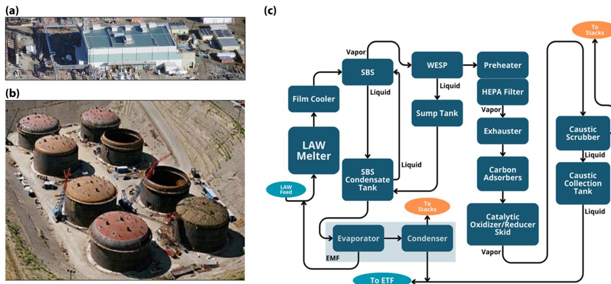
Fig. 1 Image of the (a) WTP facility (b) tank farm (with permission from Marcial *et al.*<sup>7</sup>) and (c) the flow diagram illustrates the treatment process the vitrification effluent is expected to undergo (recreated with permission from Fountain *et al.*<sup>10</sup>).
