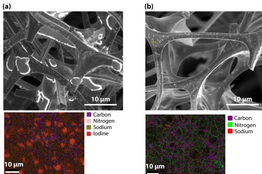
Fig. 7 SEM/EDS of (a) CF-I<sub>2</sub> and (b) CF-NO<sub>2</sub>-I<sub>2</sub>.
