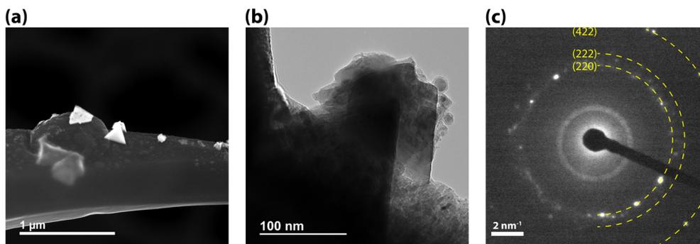
Fig. 8 (a) TEM image of CF-I<sub>2</sub>, (b) HR-TEM image of CF-I<sub>2</sub>, and (c) SAED pattern matching NaI from ICDD 00-006-0302.
