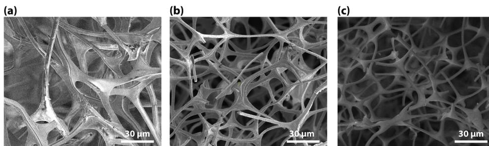
Fig. 4 SEM micrographs of (a) melamine foam (MeF), (b) carbon foam (CF), and (c) carbon foam after NO<sub>2</sub> treatment (CF-NO<sub>2</sub>).
