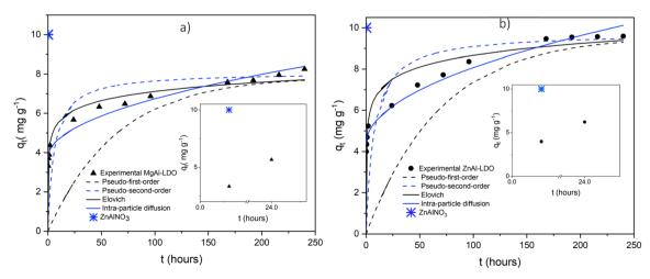
Fig. 2 Effect of contact time on the phosphorus sorption by (a) MgAl-LDO and (b) ZnAl-LDO. Symbols represent experimental data (D = 10 g L<sup>-1</sup>,  $C_i = 100$  mg L<sup>-1</sup>) while the curves correspond to the preditions through pseudo-first-order, pseudo-second-order, Elovich, and intra-particle diffusion models. The insets in each figure provide an enlarged view, highlighting the experimental point for ZnAlNO<sub>3</sub> measured at t = 0.2 h.
