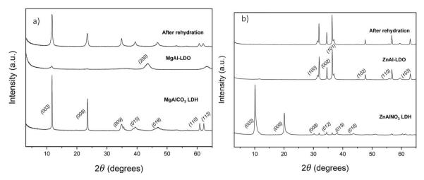
Fig. 1 XRD of (a) MgAlCO<sub>3</sub> and (b) ZnAlNO<sub>3</sub> before and after calcination, and after the rehydration process.
