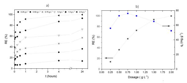
Fig. 4 Phosphorus removal using ZnAlNO<sub>3</sub> and initial solution concentration  $C_i = 100$  mg L<sup>-1</sup>: (a) Removal efficiency over time for different sorbent dosages. (b) Removal efficiency (left axis) and solid concentration (right axis) as a function of sorbent dosages at t = 24 hours.
