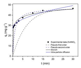
Fig. 3 Kinetic study of P removal using ZnAlNO<sub>3</sub>. Symbols are experimental data (D = 10 g L<sup>-1</sup>,  $C_i$  = 500 mg L<sup>-1</sup>), and the curves correspond to the pseudo-first, pseudo-second, Elovich, and intraparticle diffusion models.
