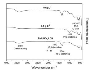
Fig. 8 FTIR analysis of ZnAlNO<sub>3</sub> powder before and after sorption of phosphorus at two different dosages (0.5 and 10 g  $L^{-1}$ ).
