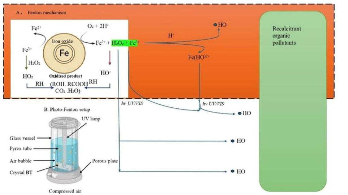
Fig. 2 Schematic representation of (A) the Fenton process (outlined in blue) and (B) the photo-Fenton process (outlined in red).
