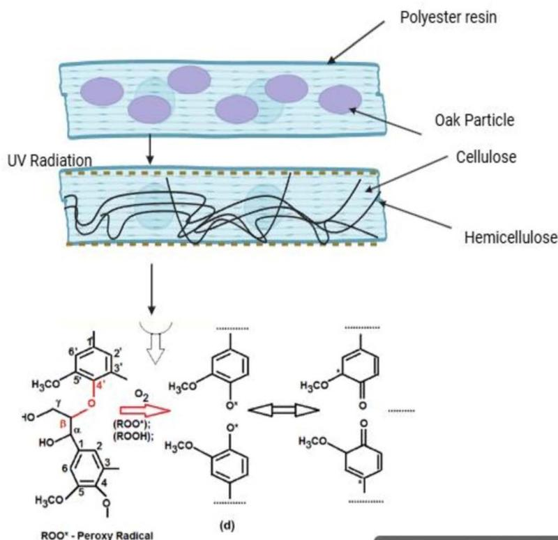
Fig. 5 Schematic representation of degradation induced by UV radiation on specimens composed of oak particles and resin.
