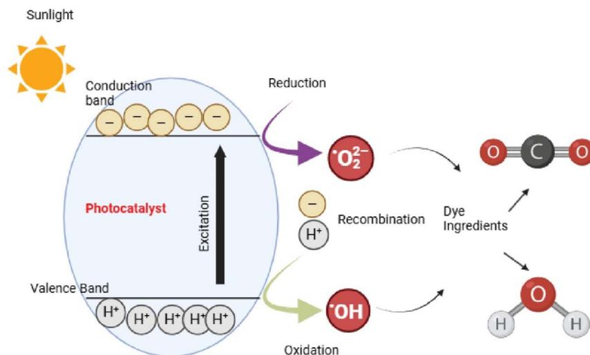
Fig. 3 The photocatalytic degradation mechanism of microplastics.
