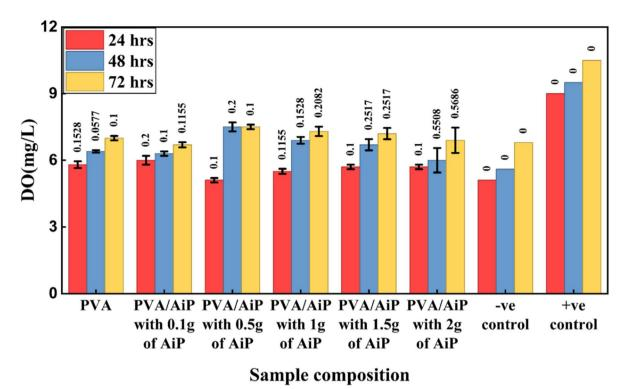
Results of oxygen permeability test for matrix PVA film and PVA/AiP hybrid films.
