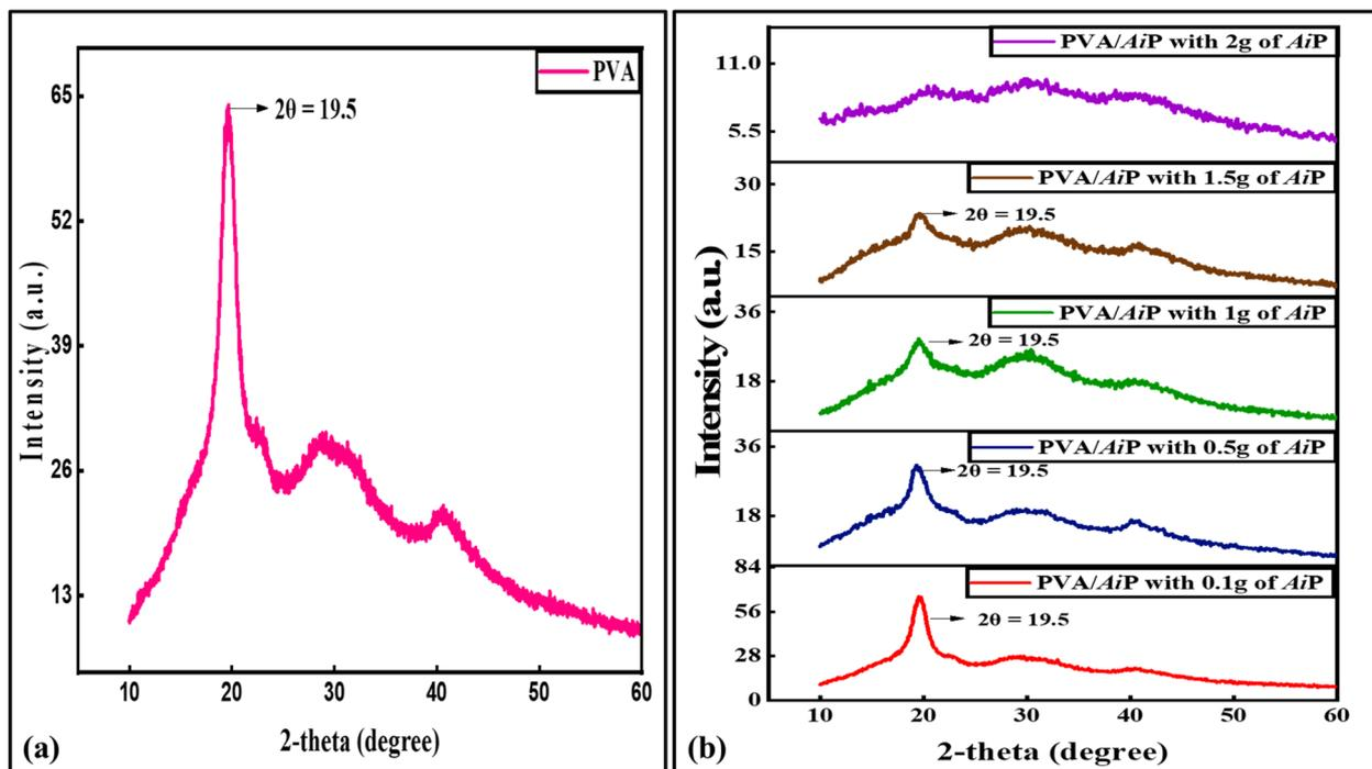
Fig. 3 X-ray diffractogram of matrix PVA (a) and PVA/AiP hybrid films (b).
