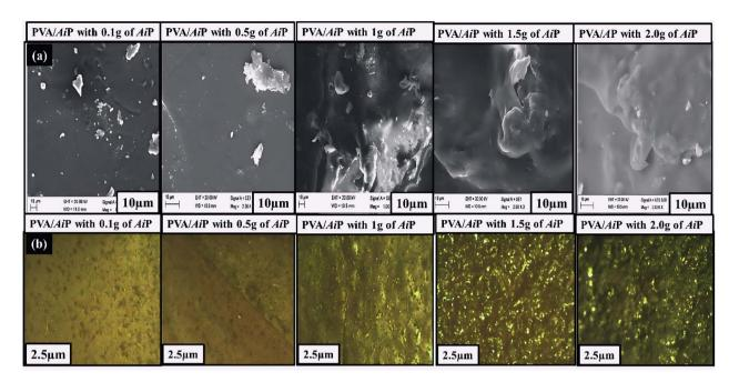
Fig. 4 SEM images (a) and optical microscopy images (b) of PVA/AiP hybrid films
