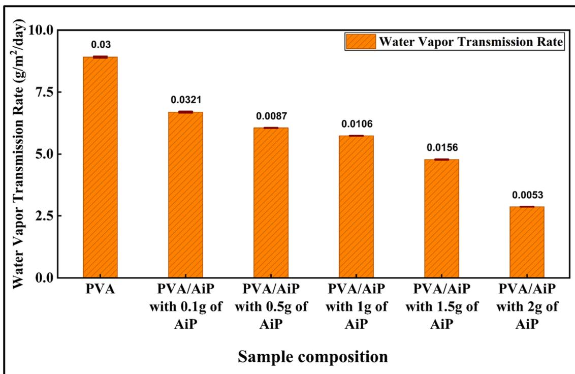
**Fig. 10** Water vapour transmission rate for matrix PVA film and PVA/AiP hybrid films.
