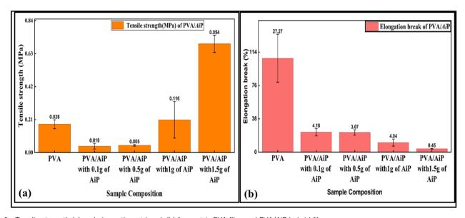
Tensile strength (a) and elongation at break (b) for matrix PVA film and PVA/AiP hybrid films
