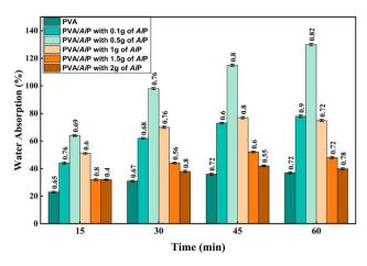
Fig. 7 Results of water absorption of matrix PVA film and PVA/AiP hybrid films.
