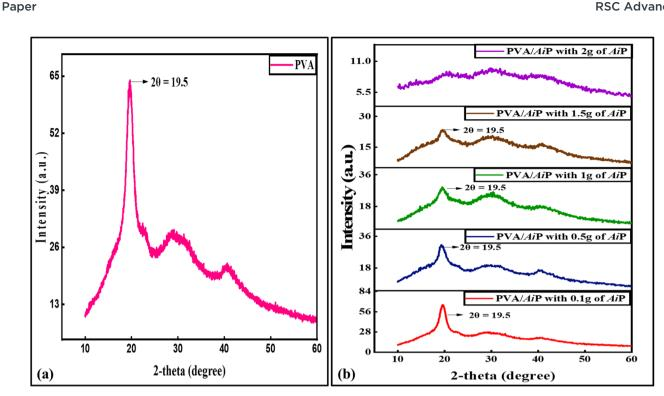
X-ray diffractogram of matrix PVA (a) and PVA/AiP hybrid films (b).
