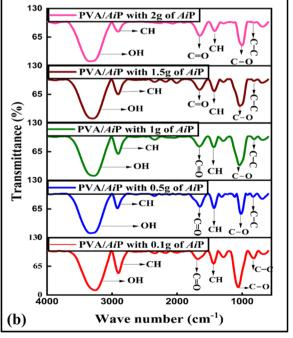
Fig. 2 FTIR spectra of matrix PVA (a) and PVA/AiP hybrid films (b).
