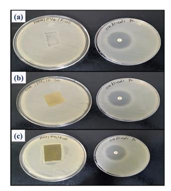
Fig. 12 Antimicrobial activity of PVA film (a), PVA/AiP with 0.1 g of AiP (b), PVA/AiP with 1.5 g of AiP (c) against  $\it E.~coli.$
