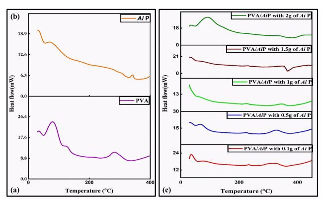
Fig. 6 DSC thermogram of matrix PVA (a) AiP filler (b) and PVA/AiP hybrid films (c).
