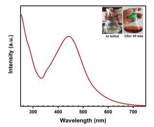
Fig. 1 UV-vis spectrum of a reaction mixture of AgNO<sub>3</sub> (40 mL of 2 mM) and Piper chaba leaf extract (2 mL of 1 g/10 mL) after 60 min of reaction time at 80 °C with (inset) the visual appearance of the reaction mixture at the initial state and after 60 min.
