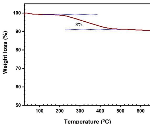
Fig. 5 TGA curve of AgNPs synthesized from 40 mL of 2 mM AgNO<sub>3</sub> and 2 mL of *Piper chaba* leaf extract (1 g/10 mL) at pH 7 and 80 °C for a reaction time of 1 h.
