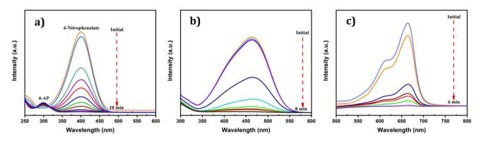
Fig. 13 Time-dependence UV-vis absorption spectra for the catalytic reduction of (a) 4-NP, (b) MO, and (c) MB by NaBH<sub>4</sub> in the presence of AgNPs synthesized using *Piper chaba* leaf extract.
