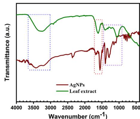
Fig. 4 FTIR spectra of the solid content of *Piper chaba* leaf extract and AgNPs synthesized using 40 mL of 2 mM AgNO<sub>3</sub> and 2 mL of *Piper chaba* leaf extract (1 g/10 mL) at pH 7 and 80 °C for a reaction time of 1 h.
