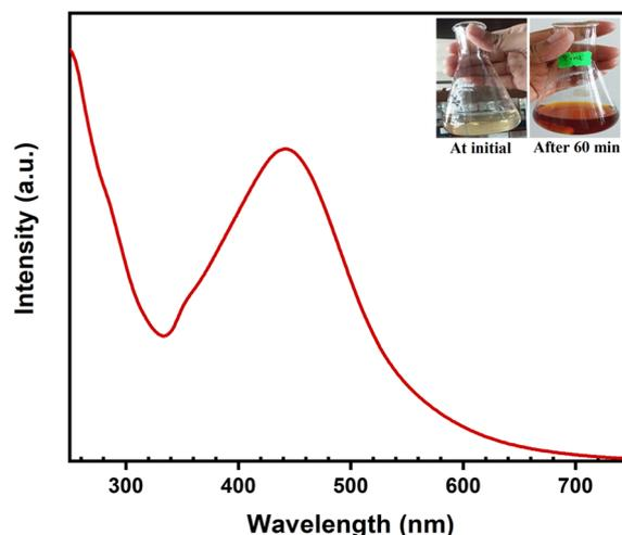
Fig. 1 UV-vis spectrum of a reaction mixture of AgNO<sub>3</sub> (40 mL of 2 mM) and *Piper chaba* leaf extract (2 mL of 1 g/10 mL) after 60 min of reaction time at 80 °C with (inset) the visual appearance of the reaction mixture at the initial state and after 60 min.
