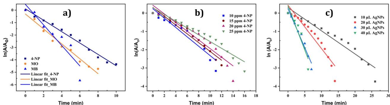
Fig. 14 Plots of ln(*A*/*A*<sub>0</sub>) versus time for the catalytic reduction of (a) 4-NP, MO, and MB; (b) for the catalytic reduction of 4-NP in different concentrations of 4-NP and (c) for the catalytic reduction of 4-NP in different dosages of AgNPs.
