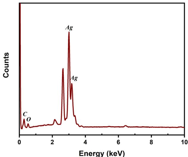
Fig. 7 EDX spectrum of AgNPs synthesized from 40 mL of 2 mM  $\text{AgNO}_3$  and 2 mL of *Piper chaba* leaf extract (1 g/10 mL) at pH 7 and 80 °C for a reaction time of 1 h.
