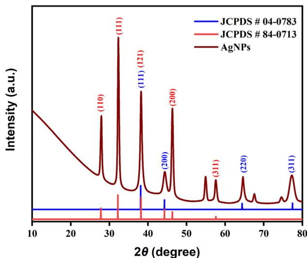
Fig. 3 XRD pattern of AgNPs synthesized using 40 mL of 2 mM AgNO<sub>3</sub> and 2 mL of *Piper chaba* leaf extract (1 g/10 mL) at pH 7 and 80 °C for a reaction time of 1 h.
