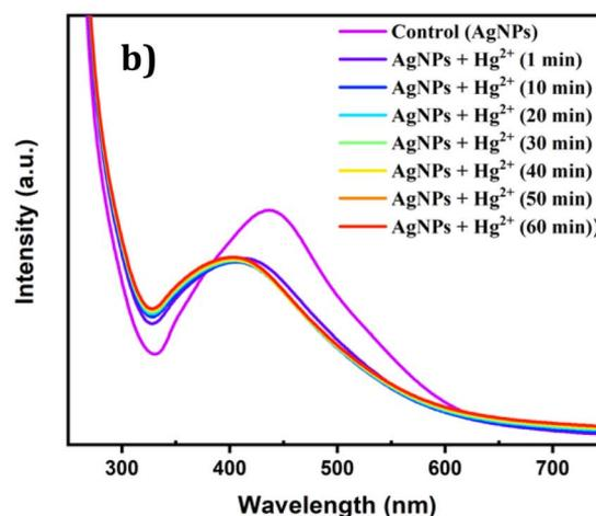
Fig. 12 (a) The regression coefficient between the change in absorbance of AgNPs and the concentration of  $\text{Hg}^{2+}$ . (b) Time-dependent UV-vis spectra of AgNPs dispersion in the presence of  $\text{Hg}^{2+}$  ions (10  $\mu\text{M}$ ).
