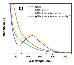
Fig. 10 Absorption spectra of AgNPs when exposed to various metal ions (a)  $Hg^{2+}$  with an individual metal ion and (b)  $Hg^{2+}$  with the mixture of metal ions.
