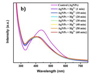
Fig. 12 (a) The regression coefficient between the change in absorbance of AgNPs and the concentration of  $Hg^{2+}$ . (b) Time-dependent UV-vis spectra of AgNPs dispersion in the presence of  $Hg^{2+}$  ions (10  $\mu$ M).
