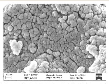
Fig. 6 FE-SEM image of AgNPs synthesized from 40 mL of 2 mM AgNO $_3$  and 2 mL of *Piper chaba* leaf extract (1 g/10 mL) at pH 7 and 80 °C for a reaction time of 1 h.
