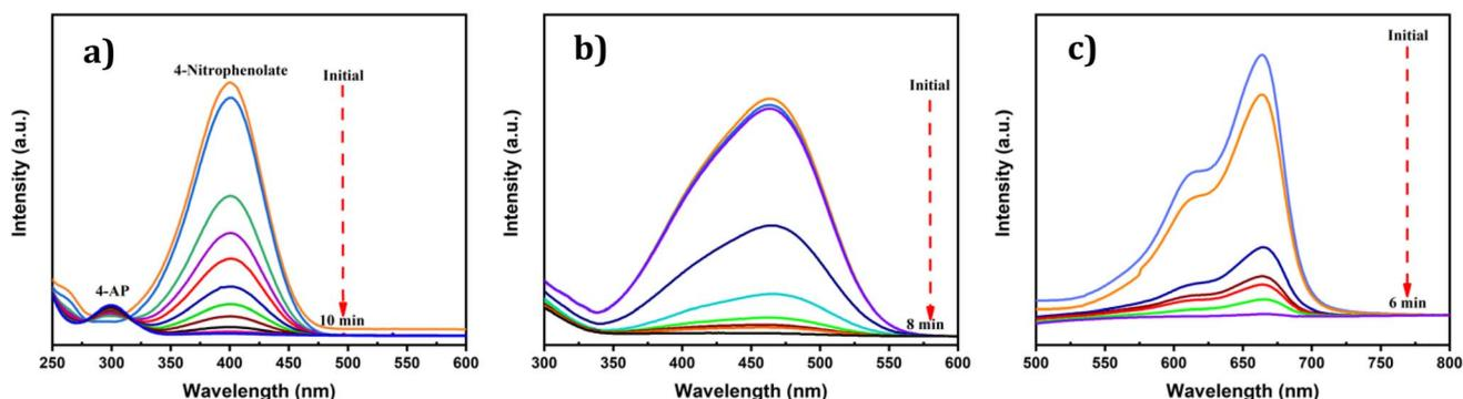
**Fig. 13** Time-dependence UV-vis absorption spectra for the catalytic reduction of (a) 4-NP, (b) MO, and (c) MB by NaBH<sub>4</sub> in the presence of AgNPs synthesized using *Piper chaba* leaf extract.
