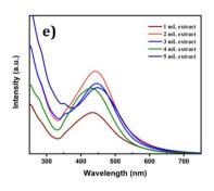
Fig. 2 UV-vis spectra of AgNPs synthesized using *Piper chaba* leaf extract under various conditions: (a) time; (b) temperature; (c) pH; (d) concentration of AgNO<sub>3</sub>; and (e) concentration of leaf extract to optimize the synthetic conditions.
