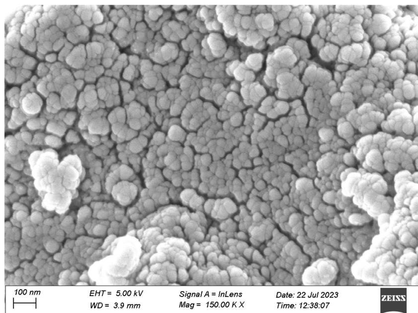
Fig. 6 FE-SEM image of AgNPs synthesized from 40 mL of 2 mM AgNO<sub>3</sub> and 2 mL of *Piper chaba* leaf extract (1 g/10 mL) at pH 7 and 80 °C for a reaction time of 1 h.
