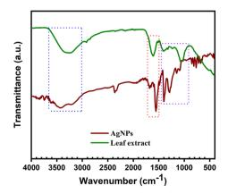
Fig. 4 FTIR spectra of the solid content of *Piper chaba* leaf extract and AgNPs synthesized using 40 mL of 2 mM AgNO $_3$  and 2 mL of *Piper chaba* leaf extract (1 g/10 mL) at pH 7 and 80 °C for a reaction time of 1 h.
