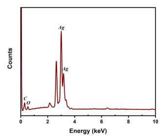
Fig. 7 EDX spectrum of AgNPs synthesized from 40 mL of 2 mM AgNO $_3$  and 2 mL of *Piper chaba* leaf extract (1 g/10 mL) at pH 7 and 80 °C for a reaction time of 1 h.
