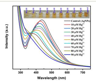
Fig. 11 Visual change and UV-vis absorption spectra of the mixtures of AgNPs and  $Hg^{2+}$  with varied  $Hg^{2+}$  concentrations (10–90  $\mu$ M).
