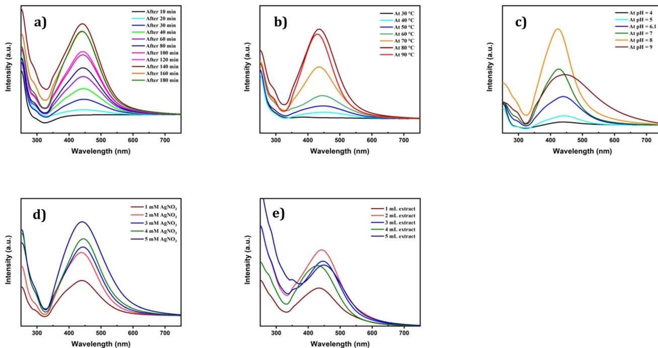
Fig. 2 UV-vis spectra of AgNPs synthesized using *Piper chaba* leaf extract under various conditions: (a) time; (b) temperature; (c) pH; (d) concentration of  $\text{AgNO}_3$ ; and (e) concentration of leaf extract to optimize the synthetic conditions.
