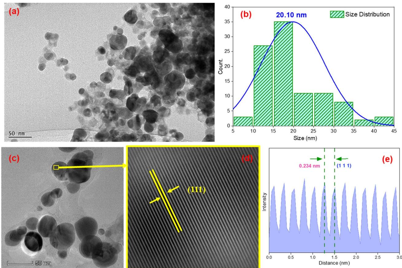
Fig. 8 (a) TEM image of AgNPs synthesized from 40 mL of 2 mM  $\text{AgNO}_3$  and 2 mL of *Piper chaba* leaf extract (1 g/10 mL) at pH 7 and 80 °C for a reaction time of 1 h, the (b) corresponding histogram, (c) TEM at 50 nm scale, (d) FFT graph of the selected area of (c), and the (e) corresponding profile plot.
