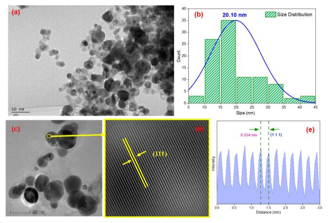
Fig. 8 (a) TEM image of AgNPs synthesized from 40 mL of 2 mM AgNO<sub>3</sub> and 2 mL of *Piper chaba* leaf extract (1 g/10 mL) at pH 7 and 80 °C for a reaction time of 1 h, the (b) corresponding histogram, (c) TEM at 50 nm scale, (d) FFT graph of the selected area of (c), and the (e) corresponding profile plot.
