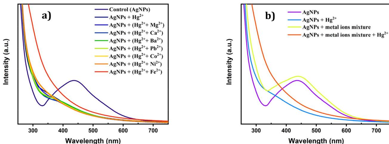
Fig. 10 Absorption spectra of AgNPs when exposed to various metal ions (a) Hg<sup>2+</sup> with an individual metal ion and (b) Hg<sup>2+</sup> with the mixture of metal ions.
