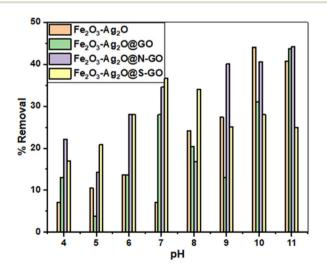
Fig. 6 Photocatalytic activity of Fe $_2$ O $_3$ -Ag $_2$ O, Fe $_2$ O $_3$ -Ag $_2$ O@O, Fe $_2$ O $_3$ -Ag $_2$ O@N-GO and Fe $_2$ O $_3$ -Ag $_2$ O@S-GO NCs at different pH levels.
