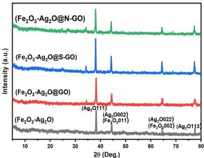
Fig. 1 XRD patterns of Fe<sub>2</sub>O<sub>3</sub>/Ag<sub>2</sub>O, Fe<sub>2</sub>O<sub>3</sub>/Ag<sub>2</sub>O/GO, Fe<sub>2</sub>O<sub>3</sub>/Ag<sub>2</sub>O/S-GO and Fe<sub>2</sub>O<sub>3</sub>/Ag<sub>2</sub>O/N-GO NCs.
