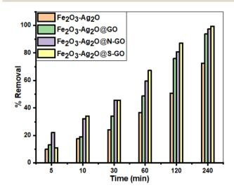
Fig. 7 Photocatalytic activity of  $Fe_2O_3-Ag_2O$ ,  $Fe_2O_3-Ag_2O$ @GO,  $Fe_2O_3-Ag_2O$ @N-GO and  $Fe_2O_3-Ag_2O$ @S-GO NCs at different time intervals.
