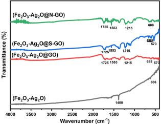
Fig. 2 FTIR spectra of Fe<sub>2</sub>O<sub>3</sub>/Ag<sub>2</sub>O, Fe<sub>2</sub>O<sub>3</sub>/Ag<sub>2</sub>O/GO, Fe<sub>2</sub>O<sub>3</sub>/Ag<sub>2</sub>O/S-GO, Fe<sub>2</sub>O<sub>3</sub>/Aq<sub>2</sub>O/N-GO NCs.
