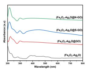
Fig. 3 UV-visible spectra of Fe<sub>2</sub>O<sub>3</sub>–Ag<sub>2</sub>O, Fe<sub>2</sub>O<sub>3</sub>–Ag<sub>2</sub>O@GO, Fe<sub>2</sub>O<sub>3</sub>-Ag<sub>2</sub>O@S-GO and Fe<sub>2</sub>O<sub>3</sub>–Ag<sub>2</sub>O@N-GO NCs.
