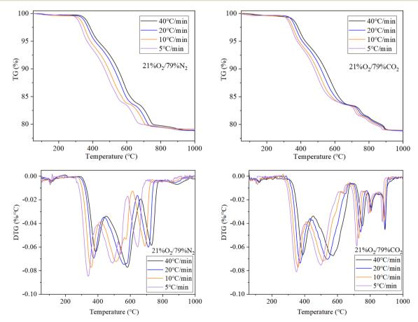
Fig. 2 TG and DTG curves of CJ oil shale combustion in the atmospheres of 21%O<sub>2</sub>/79%CO<sub>2</sub> and 21%O<sub>2</sub>/79%N<sub>2</sub>.
