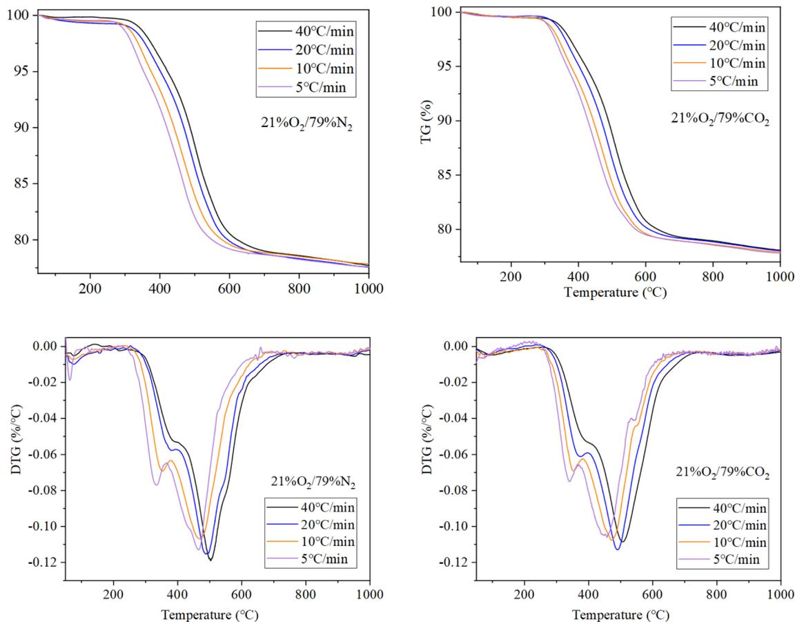
Fig. 3 TG and DTG curves of FS oil shale combustion in the atmospheres of 21%O<sub>2</sub>/79%CO<sub>2</sub> and 21%O<sub>2</sub>/79%N<sub>2</sub>.
