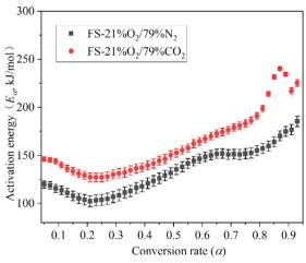
Fig. 7 Composite activation energy for CJ and FS oil shale combustion in the atmospheres of  $21\%O_2/79\%CO_2$  and  $21\%O_2/79\%N_2$ .
