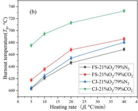
Fig. 5 Ignition temperature  $T_i$  and burnout temperature  $T_b$  for CJ and FS oil shale combustion in the atmospheres of  $21\%O_2/79\%CO_2$  and 21%O<sub>2</sub>/79%N<sub>2</sub>
