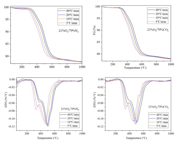
Fig. 3 TG and DTG curves of FS oil shale combustion in the atmospheres of 21%O<sub>2</sub>/79%CO<sub>2</sub> and 21%O<sub>2</sub>/79%N<sub>2</sub>.
