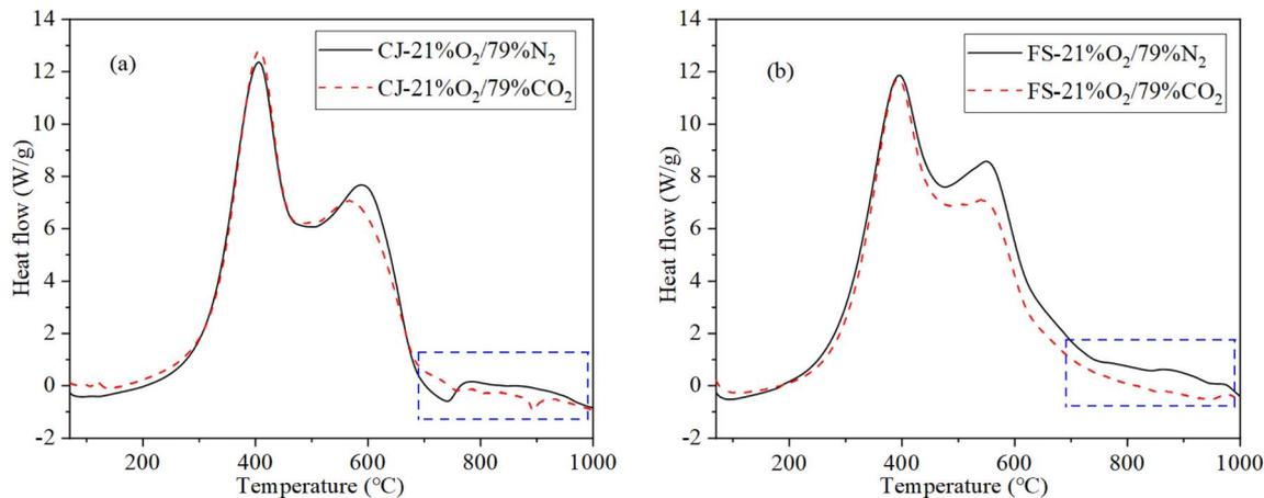
Fig. 4 Heat flow curve for CJ and FS oil shale combustion in the atmospheres of 21%O<sub>2</sub>/79%CO<sub>2</sub> and 21%O<sub>2</sub>/79%N<sub>2</sub> with heating rate of 40 °C min<sup>-1</sup>.
