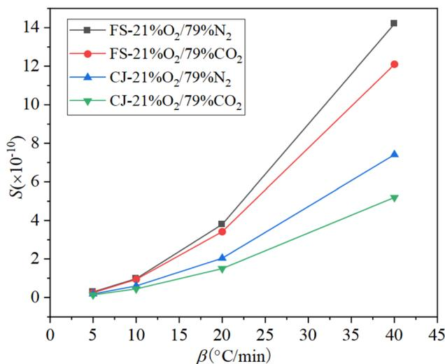
Fig. 6 Comprehensive combustion characteristics index  $S$  for CJ and FS oil shale combustion in the atmospheres of 21%O<sub>2</sub>/79%CO<sub>2</sub> and 21%O<sub>2</sub>/79%N<sub>2</sub>.
