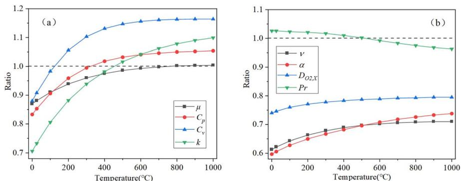
Fig. 1 The relationship between the ratio for physical properties of 21%O<sub>2</sub>/79%CO<sub>2</sub> and 21%O<sub>2</sub>/79%N<sub>2</sub> atmospheres and temperature at 1 atm pressure.
