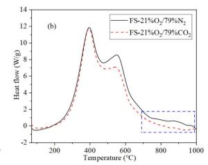
Fig. 4 Heat flow curve for CJ and FS oil shale combustion in the atmospheres of 21%O<sub>2</sub>/79%CO<sub>2</sub> and 21%O<sub>2</sub>/79%N<sub>2</sub> with heating rate of 40 °C min<sup>-1</sup>.
