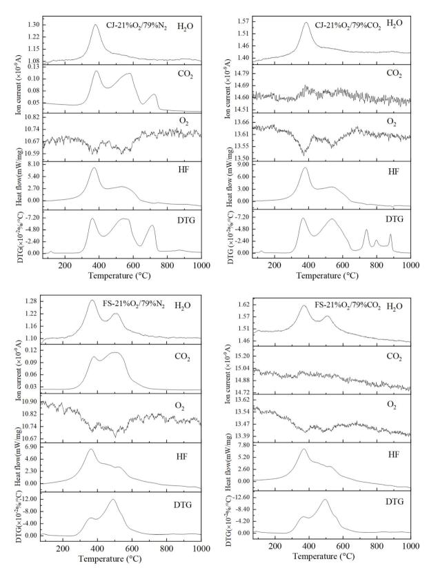
Fig. 8 O<sub>2</sub>, CO<sub>2</sub> and H<sub>2</sub>O evolution profiles followed by MS during CJ and FS oil shale combustion of 21%O<sub>2</sub>/79%CO<sub>2</sub> and 21%O<sub>2</sub>/79%N<sub>2</sub> (m/z 18, H<sub>2</sub>O; m/z 32, O<sub>2</sub>; m/z 44, CO<sub>2</sub>, 20 °C min<sup>-1</sup> heating rate).
