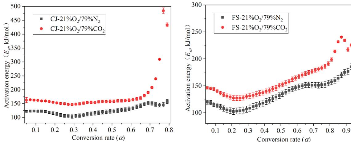
Fig. 7 Composite activation energy for CJ and FS oil shale combustion in the atmospheres of 21%O<sub>2</sub>/79%CO<sub>2</sub> and 21%O<sub>2</sub>/79%N<sub>2</sub>.
