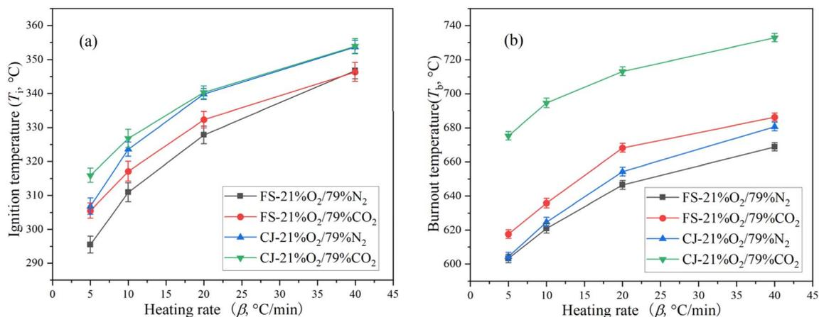
Fig. 5 Ignition temperature  $T_i$  and burnout temperature  $T_b$  for CJ and FS oil shale combustion in the atmospheres of 21%O<sub>2</sub>/79%CO<sub>2</sub> and 21%O<sub>2</sub>/79%N<sub>2</sub>.
