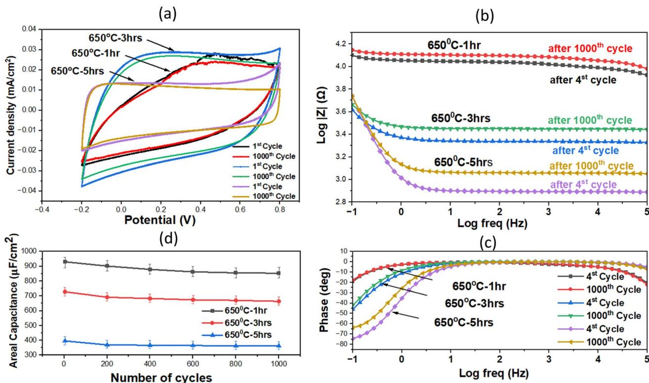
Fig. 8 (a) CV performance of  $\text{TiO}_2\text{@C}$  core-shell NWs *in situ*-annealed at  $650^\circ\text{C}$  for 1, 3, and 5 hours and their corresponding (b) Bode plots and (c) phase plots undergoing 1000 cycles, and (d) areal capacitance values across 1000 cycles.
