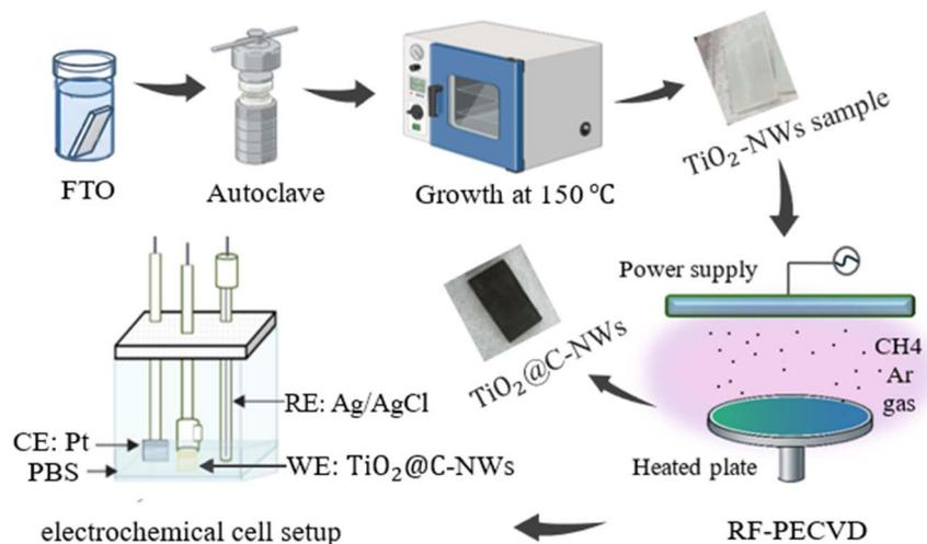
Fig. 1 Schematic illustration of the synthesis process of  $\text{TiO}_2@C$  core-shell NWs, followed by electrochemical characterization using a three-electrode cell setup.
