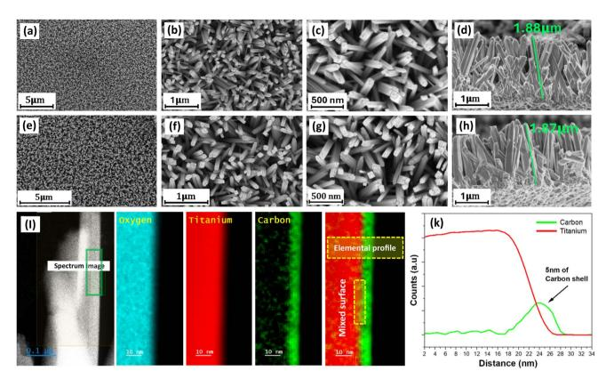
Fig. 2 SEM images of (a–d) pristine  $TiO_2$ -NWs, (e–h)  $TiO_2$ @C core-shell NWs annealed at 650 °C for 3 hours, (i) its STEM image and EELS elemental mapping, and (k) Elemental profile for C and Ti-edge.
