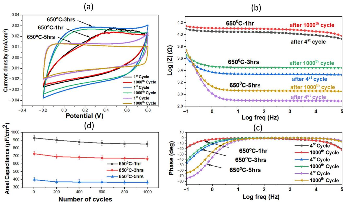
Fig. 8 (a) CV performance of  $\text{TiO}_2\text{@C}$  core-shell NWs *in situ*-annealed at 650 °C for 1, 3, and 5 hours and their corresponding (b) Bode plots and (c) phase plots undergoing 1000 cycles, and (d) areal capacitance values across 1000 cycles.
