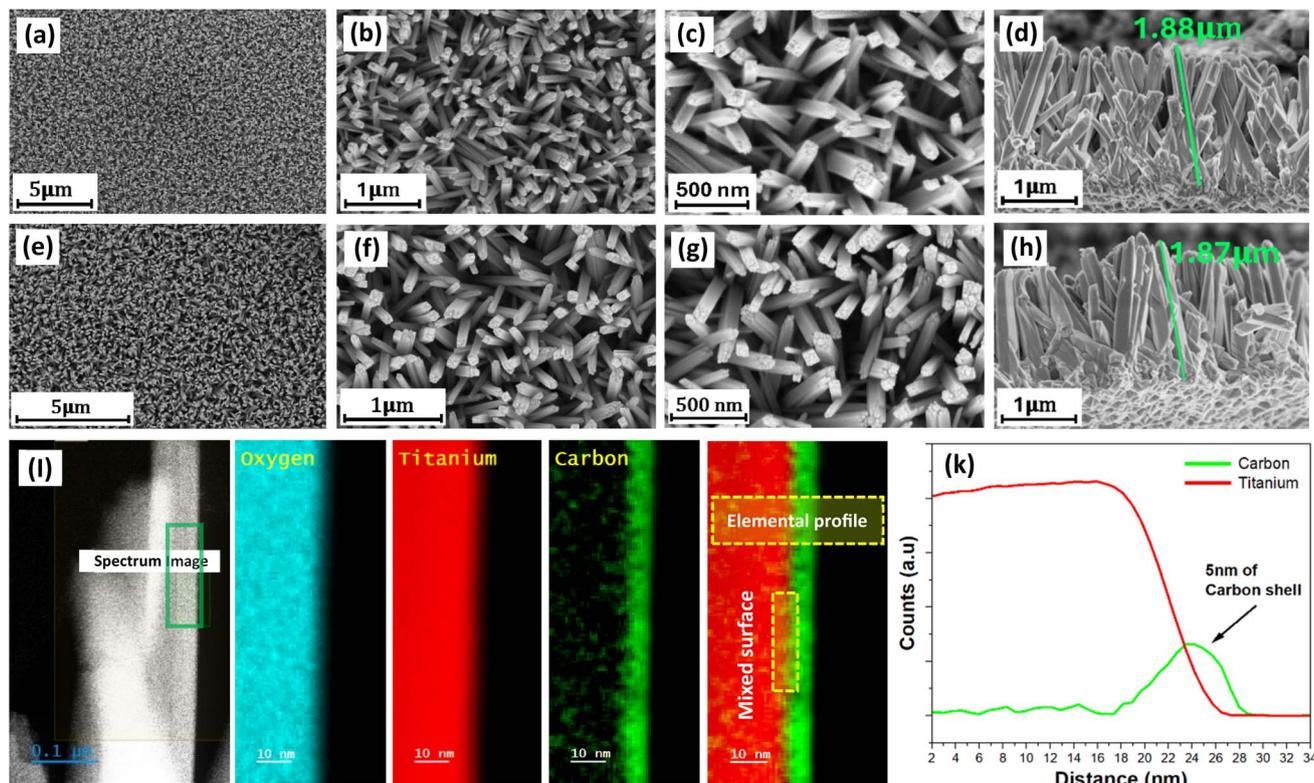
Fig. 2 SEM images of (a–d) pristine  $\text{TiO}_2$ -NWs, (e–h)  $\text{TiO}_2$ @C core-shell NWs annealed at 650 °C for 3 hours, (i) its STEM image and EELS elemental mapping, and (k) Elemental profile for C and Ti-edge.
