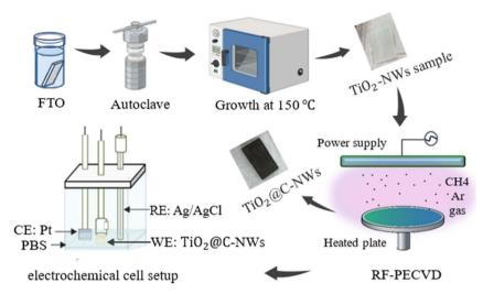
Fig. 1 Schematic illustration of the synthesis process of TiO<sub>2</sub>@C core—shell NWs, followed by electrochemical characterization using a three-electrode cell setup.
