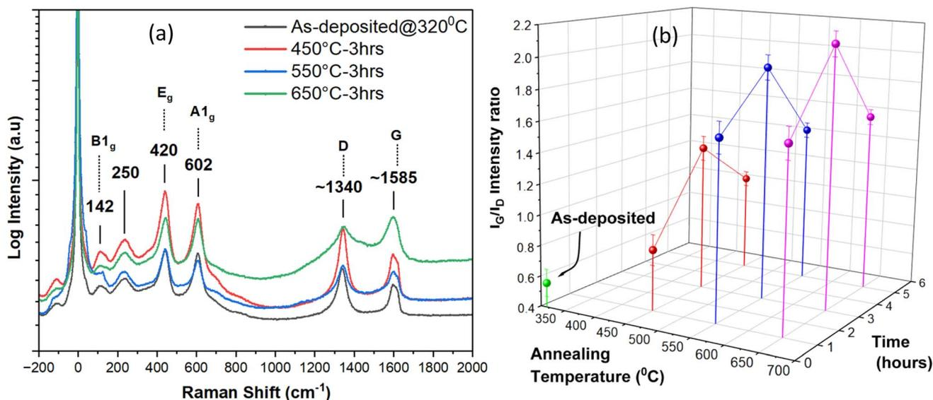
Fig. 4 (a) Raman spectroscopy of as-deposited  $\text{TiO}_2@C$  core-shell NWs and *in situ* annealed at 450 °C, 550 °C, and 650 °C for 3 hours, (b)  $I_G/I_D$  ratio of all treated samples.
