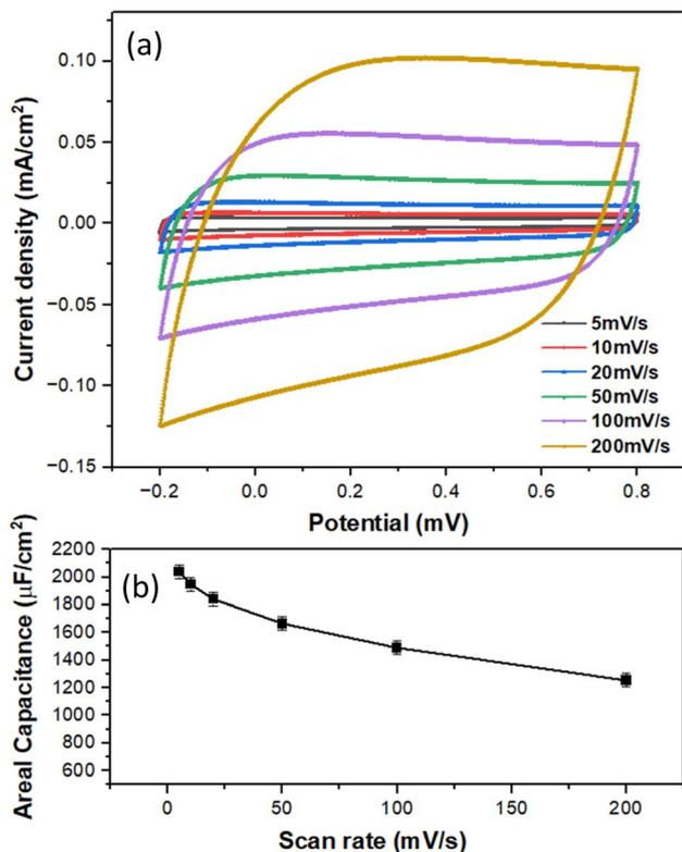
Fig. 9 (a) CV performance of TiO<sub>2</sub>@C core-shell NWs *in situ*-annealed at 650 °C for 3 hours measured at various scan rate, and (b) corresponding plot of areal capacitance vs. scan rate.
