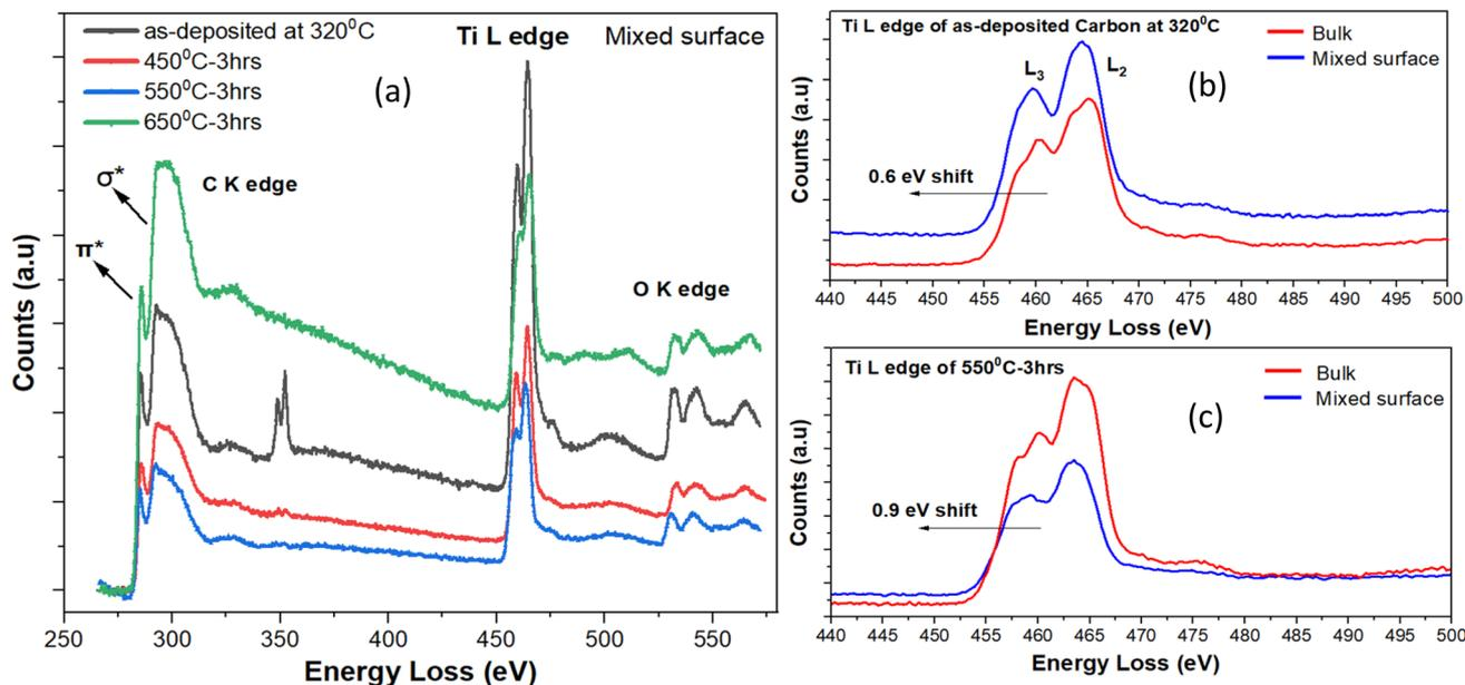
Fig. 3 (a) Overall EELS spectrum (from  $\text{TiO}_2$ -C interface) of as-deposited  $\text{TiO}_2$ @C core-shell NWs and *in situ* annealed at 450 °C, 550 °C, and 650 °C for 3 hours, (b) Ti L-edge of the as-deposited  $\text{TiO}_2$ @C core-shell NW and (c) the *in situ* annealed at 550 °C for 3 hours.
