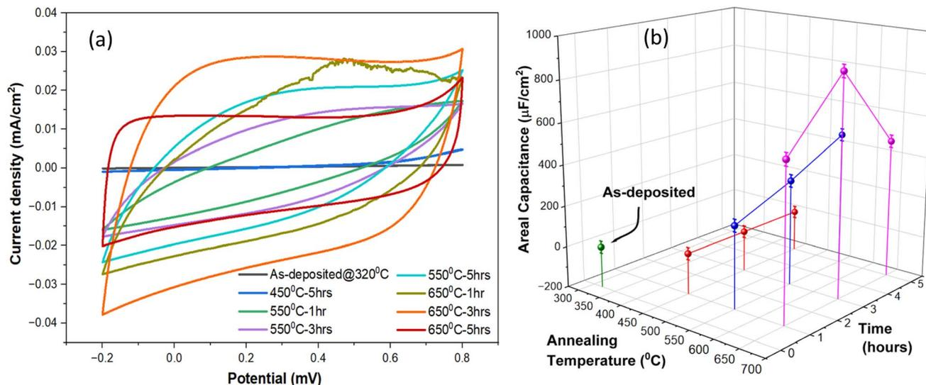
Fig. 6 (a) CV measurements of as-deposited  $\text{TiO}_2$ @C core-shell NWs and *in situ* annealed at 450 °C, 550 °C, and 650 °C for varying duration showing (b) corresponding areal capacitance.
