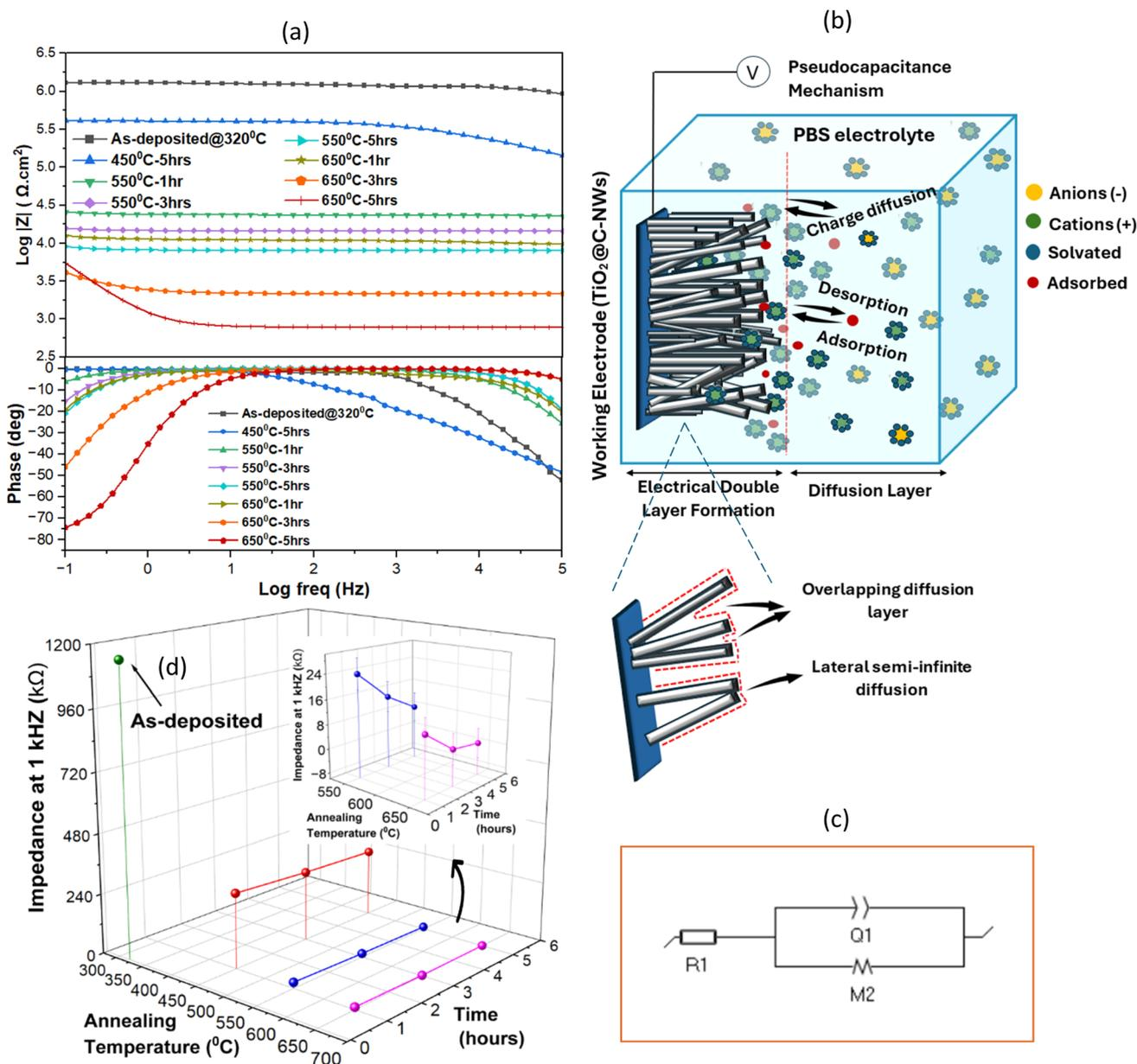
Fig. 7 EIS performance of as-deposited  $\text{TiO}_2$ @C core-shell NWs and *in situ* annealed at 450 °C, 550 °C, and 650 °C for varying duration showing (a) the Bode and phase plots, (b) schematic illustration of electrolyte diffusion mechanism, (c) equivalent circuit of  $\text{TiO}_2$ @C core-shell NWs *in situ* annealed at 650 °C for 3 hours, (d) impedance values of treated samples at 1 kHz.
