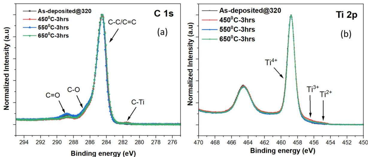
Fig. 5 XPS of as-deposited TiO<sub>2</sub>@C core-shell NWs and *in situ* annealed at 450 °C, 550 °C, and 650 °C for 3 hours, showing (a) C 1s core-level, (b) Ti 2p core-level.
