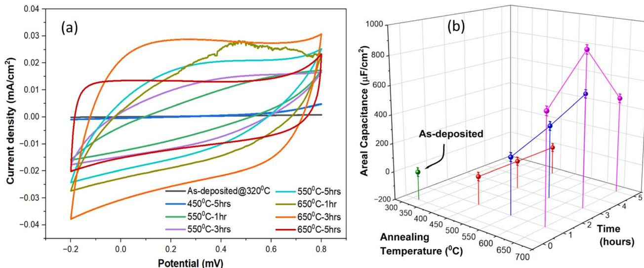
Fig. 6 (a) CV measurements of as-deposited TiO<sub>2</sub>@C core-shell NWs and *in situ* annealed at 450 °C, 550 °C, and 650 °C for varying duration showing (b) corresponding areal capacitance.
