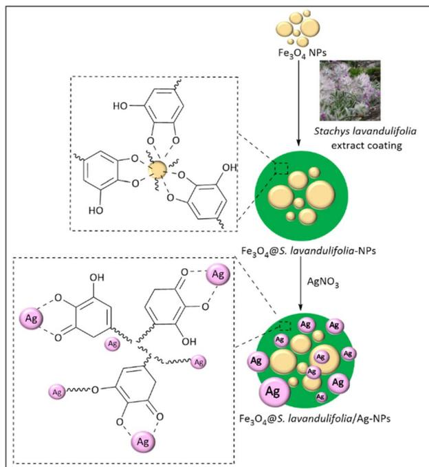
Scheme 5 Synthetic pathway of  $\text{Fe}_3\text{O}_4@S. Lavandulifolia/Ag$  nanocatalyst.
