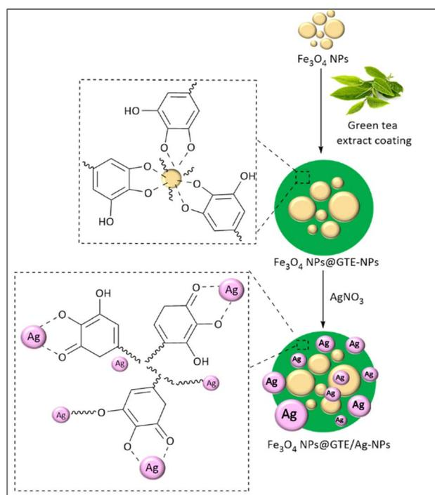
Scheme 13 Preparation process of the Fe<sub>3</sub>O<sub>4</sub>@GTE/Ag-NPs catalyst.
