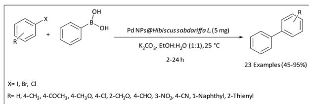
Scheme 28 Suzuki–Miyaura coupling reaction catalysed by Pd NPs@*Hibiscus sabdariffa* L. as catalyst.
