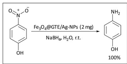
Scheme 14  $\text{Fe}_3\text{O}_4@\text{GTE}/\text{Ag-NPs}$  as the catalyst in the reduction reaction of 4-nitrophenol to 4-aminophenol.
