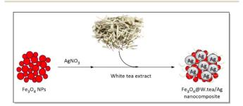
Scheme 56 Green synthesis of the Fe<sub>3</sub>O<sub>4</sub>@W.tea/Ag nanocomposites using white tea extract.
