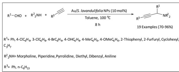
Scheme 51 The A<sup>3</sup>-coupling reaction in the presence of the Au/*S. lavandulifolia* NPs catalyst.
