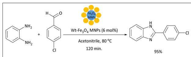
Scheme 33 Synthesis of 2-(4-chlorophenyl)-1H-benzod[imidazole] catalyzed by Wt-Fe<sub>3</sub>O<sub>4</sub> MNPs.
