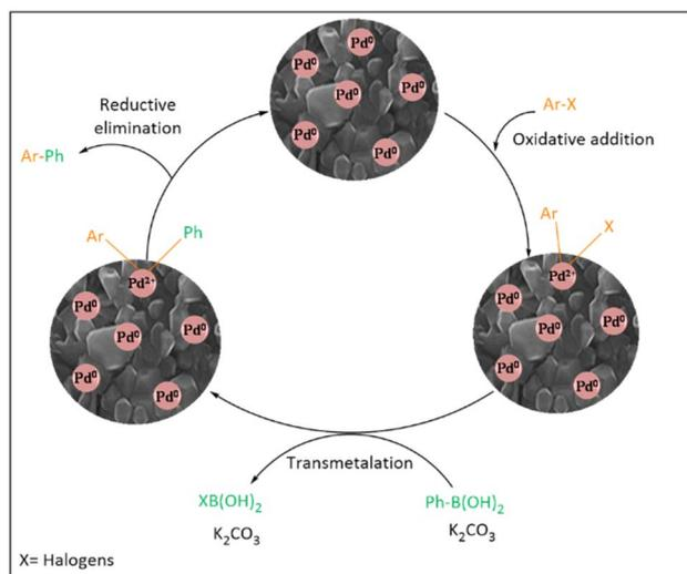
Scheme 20 Possible mechanism of the Suzuki–Miyaura coupling reaction.
