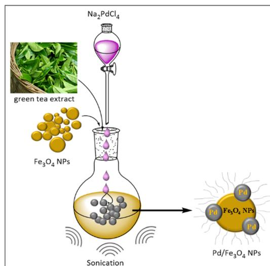
Scheme 24 Preparation of Pd/Fe<sub>3</sub>O<sub>4</sub> NPs assisted by green tea extract under ultrasonic irradiations.
