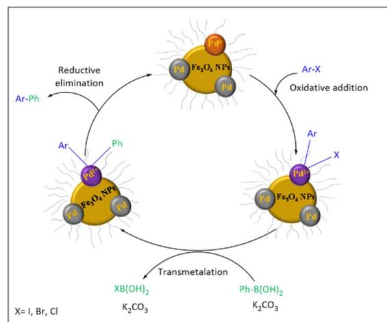
Scheme 26 Possible mechanism of the Suzuki–Miyaura coupling reaction using Pd/Fe<sub>3</sub>O<sub>4</sub> NPs as the catalyst.
