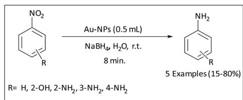
Scheme 15 Au-NPs catalyzed reduction of nitro aromatics by  $\text{NaBH}_4$ .
