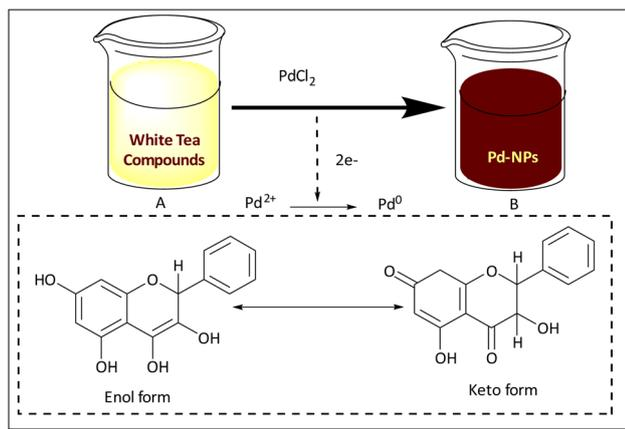
Scheme 37 The aqueous extract of white tea (A) before and (B) after the synthesis of Pd-NPs.
