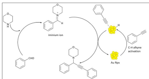
Scheme 52 Probable mechanism for the A<sup>3</sup>-coupling reaction using Au/*S. lavandulifolia* NPs.
