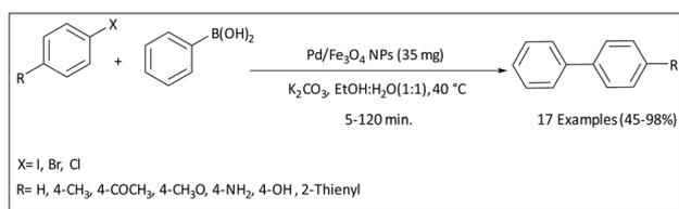
Scheme 25 The Suzuki–Miyaura reaction using Pd/Fe<sub>3</sub>O<sub>4</sub> NPs as the catalyst.
