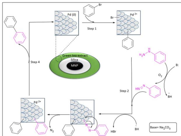
Scheme 49 Proposed mechanism for the denitrogenative bromobenzene and phenylhydrazine coupling by ION-SiO<sub>2</sub>/TE-Pd(0) nanocatalyst.
