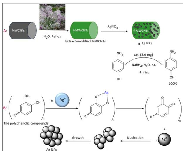
**Scheme 9** (A): Depiction of the eco-friendly functionalization process for MWCNTs, subsequent *in situ* reduction of  $\text{Ag}^+$  ions leading to the formation of Ag-NPs on functionalized MWCNTs (f-MWCNTs) via *Stachys lavandulifolia* extract, producing the Ag NPs/MWCNTs@*S. lavandulifolia* nanocatalyst utilized in 4-nitrophenol reduction; (B): suggested mechanism for Ag-NPs synthesis by *Stachys lavandulifolia* extract.
