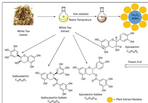
Scheme 32 Synthesis of Wt-Fe<sub>3</sub>O<sub>4</sub> MNPs using white tea extract.
