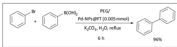
Scheme 22 Suzuki–Miyaura coupling reaction catalyzed by Pd-NPs@FT.
