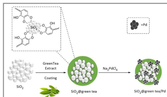
**Scheme 42** Green metric synthesis of the SiO<sub>2</sub>@green tea/Pd nanocomposite and its catalytic use in Buchwald–Hartwig C–N coupling.
