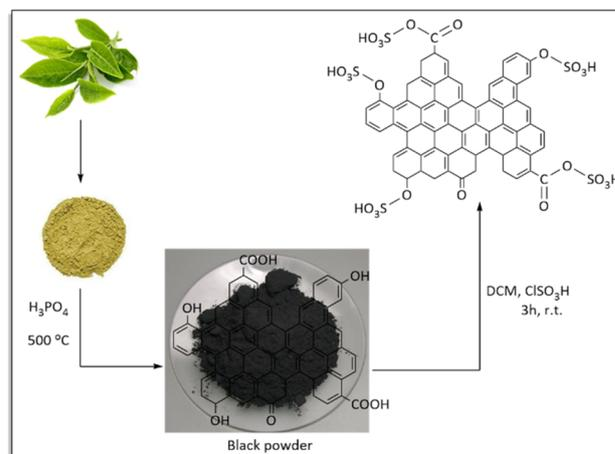
Scheme 35 Schematic of MTLAC-SA synthesis.
