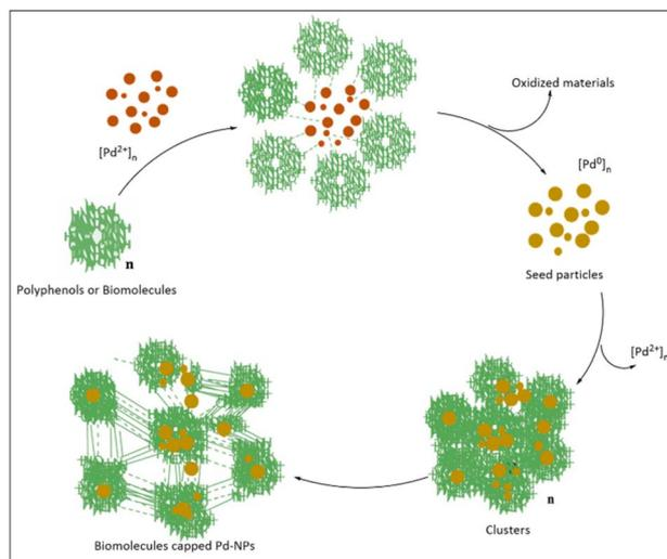
Scheme 16 Proposed reaction pathway for the synthesis of Pd-NPs.
