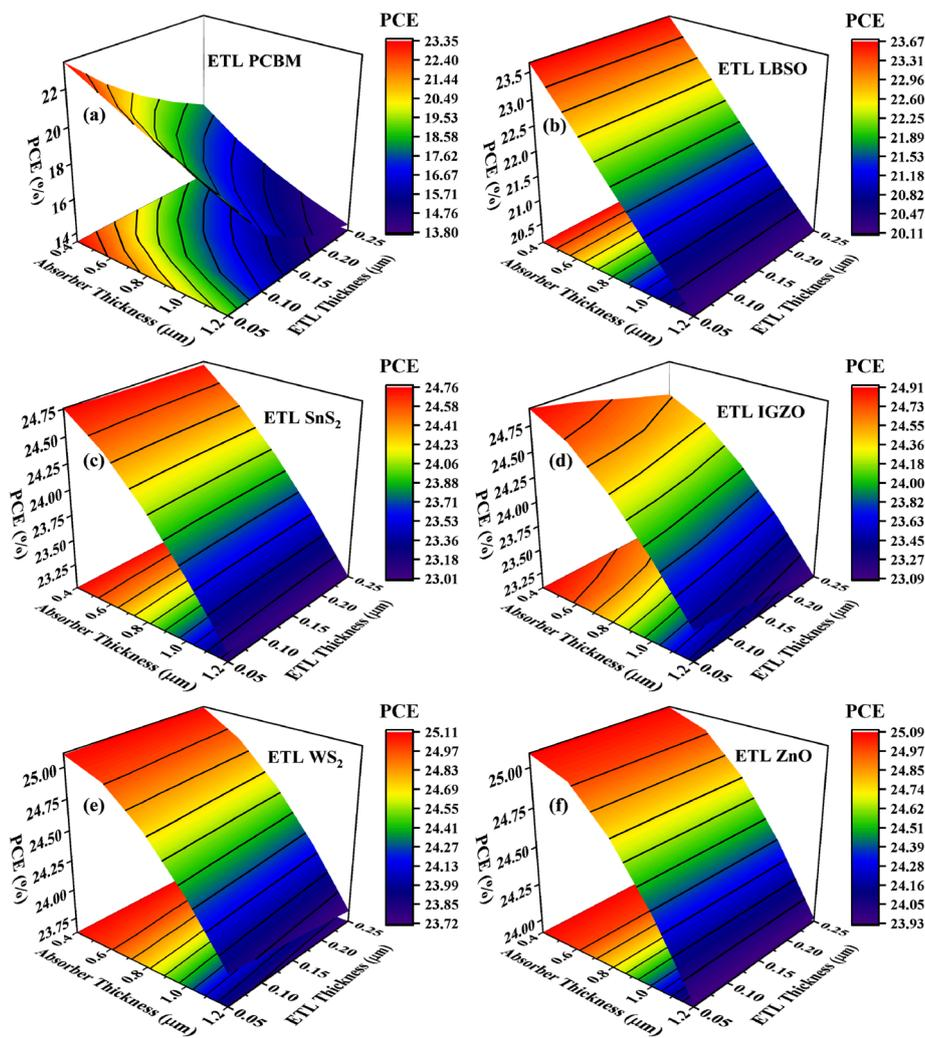
Fig. 9 3D colormap of PCE when ETL is (a) PCBM, (b) LBSO, (c) SnS<sub>2</sub>, (d) IGZO, (e) WS<sub>2</sub>, and (f) ZnO.
