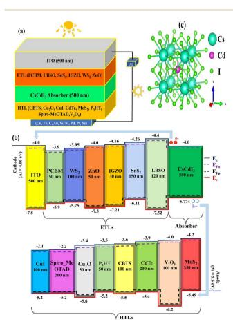
Fig. 2 (a) Schematic device structure, (b) energy band level alignment of the related (a) ITO, ETLs, and absorber  $CsCdl_3$ , and (b) HTLs, and (c) crystal structure.
