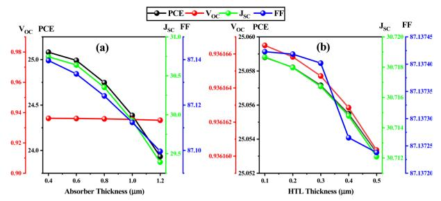
Fig. 14 Influence on PV parameters considering the variation in (a) absorber (CsCdl<sub>3</sub>) thickness, and (b) HTL (MoS<sub>2</sub>) thickness.
