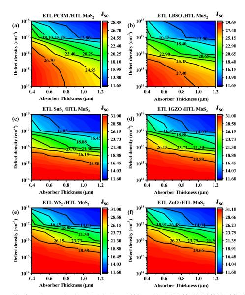
Fig. 11 Contour map of  $J_{SC}$  dependency on absorber defect density and thickness when ETL is (a) PCBM, (b) LBSO, (c) SnS<sub>2</sub>, (d) IGZO, (e) WS<sub>2</sub>, and (f) ZnO.
