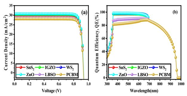
Fig. 19 (a) J-V characteristics and (b) quantum efficiency (QE) curve of CsCdl<sub>3</sub> PSC
