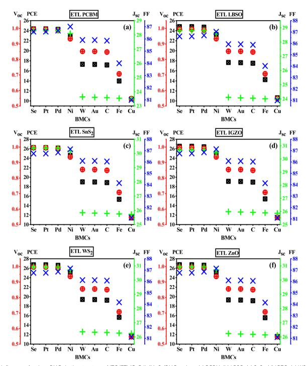
Fig. 3 Influence of various BMCs in the structure of ITO/ETL/CsCdl<sub>3</sub>/MoS<sub>2</sub>/BMCs, where (a) PCBM, (b) LBSO, (c) SnS<sub>2</sub>, (d) IGZO, (e) WS<sub>2</sub>, and (f) ZnO are used as ETL.
