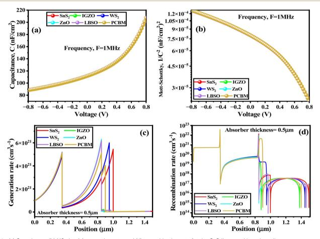
Fig. 18 (a) Capacitance, (b) MS plot, (c) generation rate, and (d) recombination rate for the  $CsCdl_3$  perovskite solar cell.
