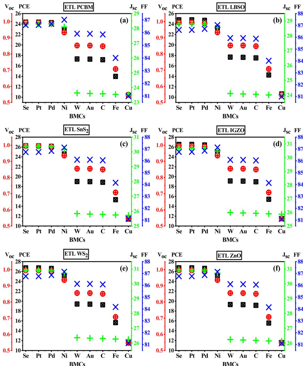
Fig. 3 Influence of various BOCs in the structure of ITO/ETL/CsCdI<sub>3</sub>/MoS<sub>2</sub>/BOCs, where (a) PCBM, (b) LBSO, (c) SnS<sub>2</sub>, (d) IGZO, (e) WS<sub>2</sub>, and (f) ZnO are used as ETL.
