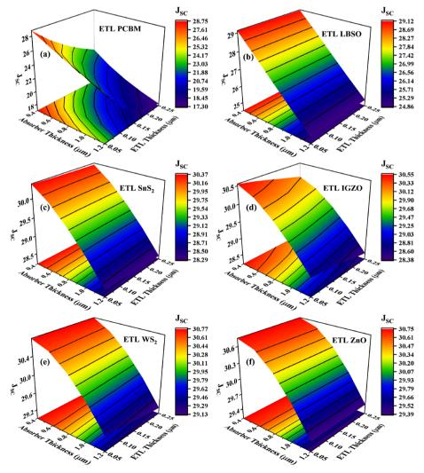
Fig. 7 3D colormap of J<sub>SC</sub> when ETL is (a) PCBM, (b) LBSO, (c) SnS<sub>2</sub>, (d) IGZO, (e) WS<sub>2</sub>, and (f) ZnO.
