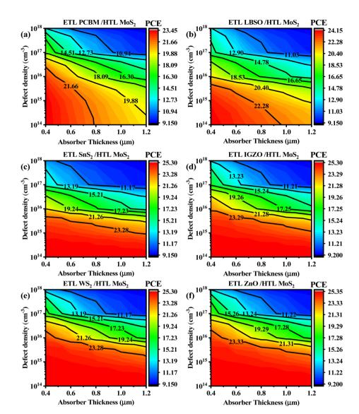
Fig. 13 Contour map of PCE dependency on absorber defect density and thickness when ETL is (a) PCBM, (b) LBSO, (c) SnS<sub>2</sub>, (d) IGZO, (e) WS<sub>2</sub>, and (f) ZnO
