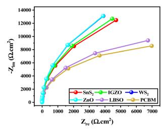
Fig. 20 Nyquist plot of the various ETL materials based on the structure of  $ITO/ETL/CsCdl_3/MoS_2/Ni$ , where PCBM, LBSO, SnS<sub>2</sub>, IGZO, WS<sub>2</sub>, and ZnO are used as ETL.
