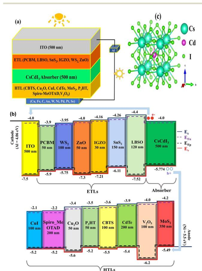
Fig. 2 (a) Schematic device structure, (b) energy band level alignment of the related (a) ITO, ETLs, and absorber CsCdI<sub>3</sub>, and (b) HTLs, and (c) crystal structure.
