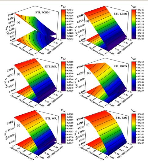
Fig. 6 3D colormap of  $V_{OC}$  when ETL is (a) PCBM, (b) LBSO, (c) SnS<sub>2</sub>, (d) IGZO, (e) WS<sub>2</sub>, and (f) ZnO.
