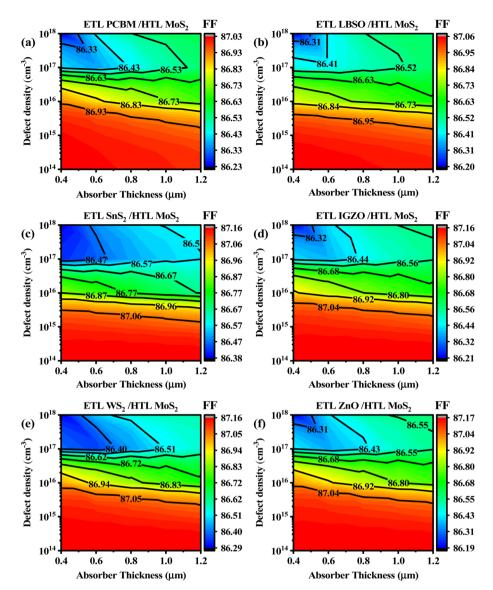
Fig. 12 Contour map of FF dependency on absorber defect density and thickness when ETL is (a) PCBM, (b) LBSO, (c) SnS<sub>2</sub>, (d) IGZO, (e) WS<sub>2</sub>, and (f) ZnO.
