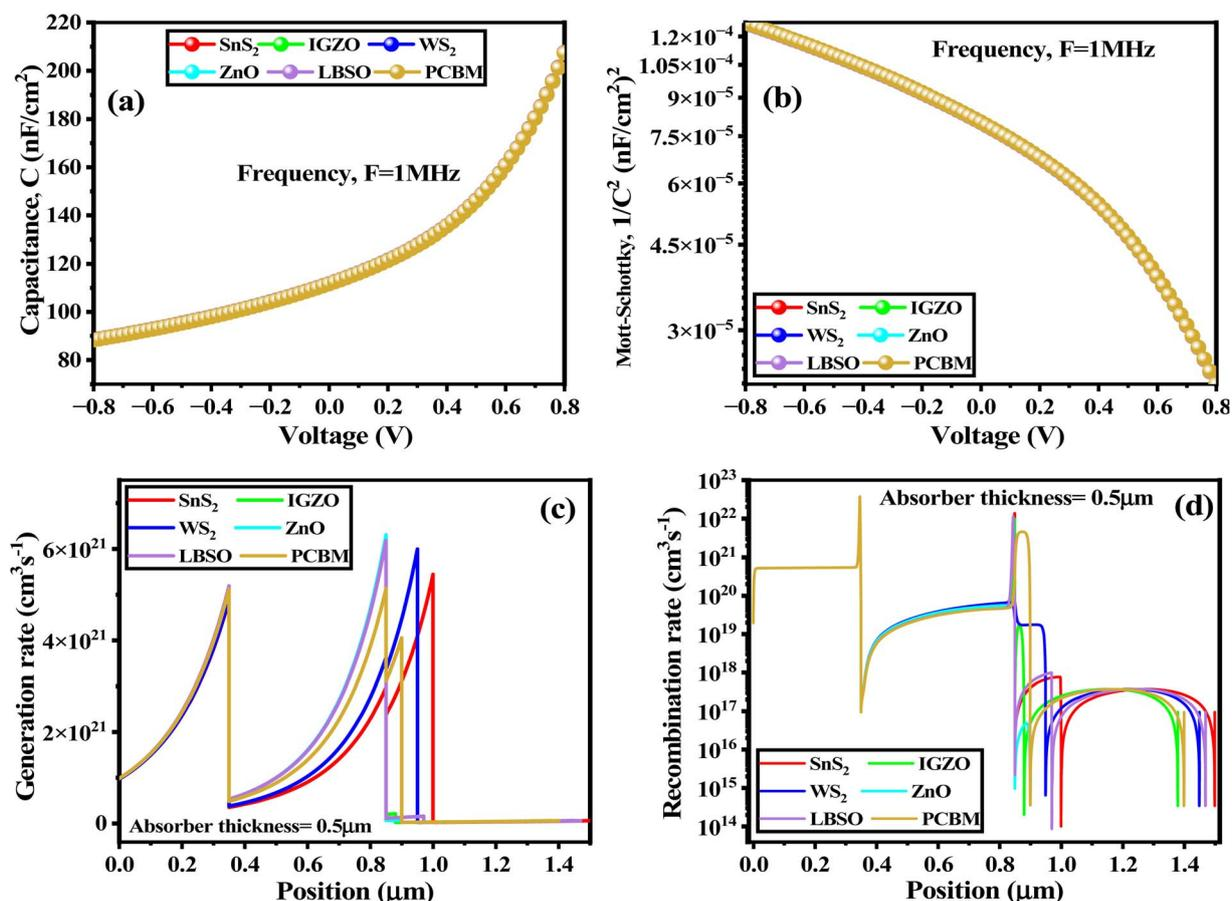
Fig. 18 (a) Capacitance, (b) MS plot, (c) generation rate, and (d) recombination rate for the CsCdI<sub>3</sub> perovskite solar cell.
