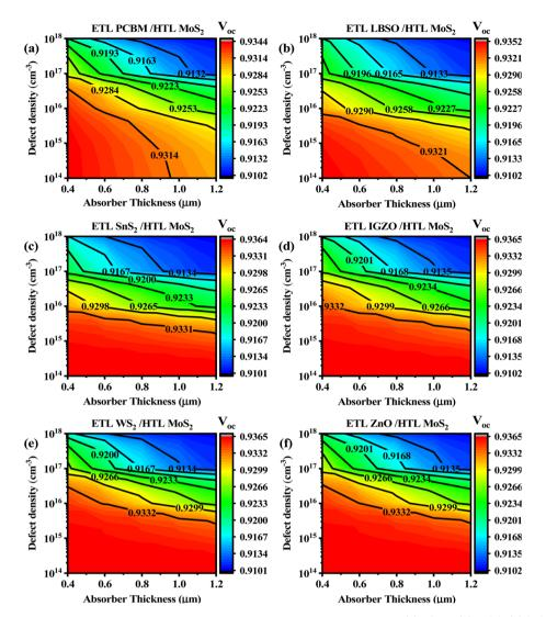
Fig. 10 Contour map of  $V_{\rm OC}$  dependency on absorber defect density and thickness when ETL is (a) PCBM, (b) LBSO, (c) SnS<sub>2</sub>, (d) IGZO, (e) WS<sub>2</sub>, and (f) ZnO.
