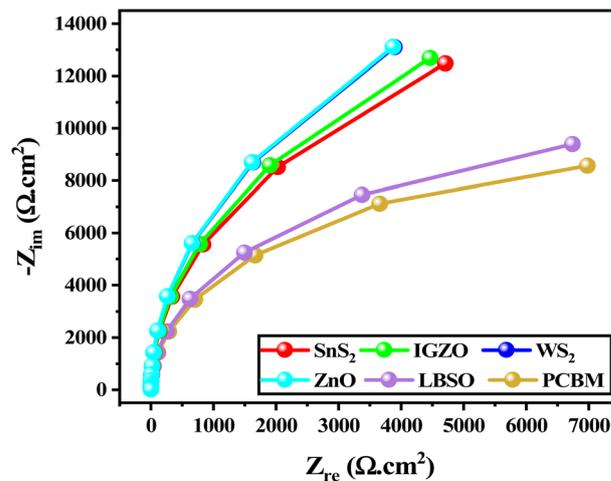
Fig. 20 Nyquist plot of the various ETL materials based on the structure of ITO/ETL/CsCdI<sub>3</sub>/MoS<sub>2</sub>/Ni, where PCBM, LBSO, SnS<sub>2</sub>, IGZO, WS<sub>2</sub>, and ZnO are used as ETL.
