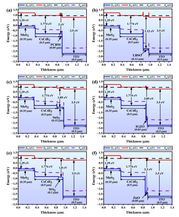
Fig. 5 Band diagrams of the various ETL materials based on the structure of ITO/ETL/CsCdl<sub>3</sub>/MoS<sub>2</sub>/Ni, where (a) PCBM, (b) LBSO, (c) SnS<sub>2</sub>, (d) IGZO, (e) WS<sub>2</sub>, and (f) ZnO are used as ETL.
