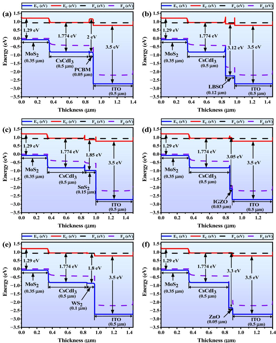
Fig. 5 Band diagrams of the various ETL materials based on the structure of ITO/ETL/CsCdI<sub>3</sub>/MoS<sub>2</sub>/Ni, where (a) PCBM, (b) LBSO, (c) SnS<sub>2</sub>, (d) IGZO, (e) WS<sub>2</sub>, and (f) ZnO are used as ETL.
