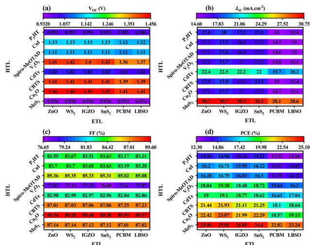
Fig. 4 Impact of various HTL and ETL in PSC while Ni is used as BMC in the structure of ITO/ETLs/CsCdI<sub>3</sub>/HTLs/Ni. (a) V<sub>OC</sub>. (b) J<sub>SC</sub>. (c) FF, and (d) PCE.
