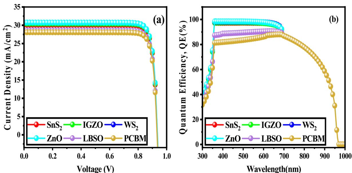
Fig. 19 (a) *J–V* characteristics and (b) quantum efficiency (QE) curve of CsCdI<sub>3</sub> PSC.
