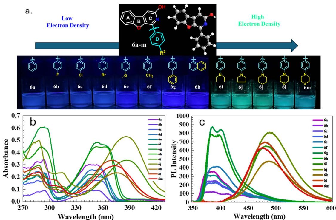
Fig. 5 (a) Photograph of the compounds 6a–m in DMSO under 365 nm UV irradiation (b) UV-visible absorbance (20  $\mu$ M) and (c) emission spectra (10  $\mu$ M) of derivatives of 6, at 20  $^{\circ}$ C; excitation and emission slit width of 5, 5 nm, 600 V except 6g and 6h-570 V.
