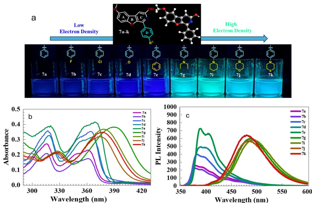
Fig. 6 (a) Photograph of the compounds 7a–k in DMSO under 365 nm UV irradiation, (b) UV-visible absorbance (20  $\mu\text{M}$ ) and (c) emission spectra of derivatives (7a–k), 10  $\mu\text{M}$  at 20 °C; excitation and emission slit width of 5; 5 nm, 600 V.
