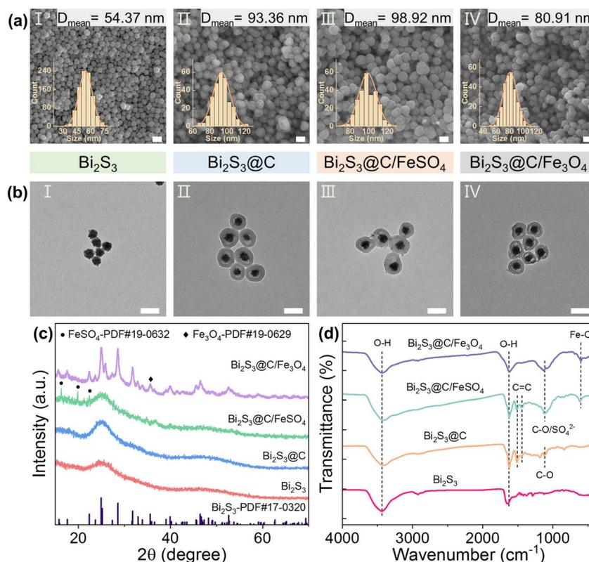
Fig. 1 (a) SEM images (inset: size distributions), (b) TEM images, (c and d) XRD patterns, and FT-IR spectra of  $\text{Bi}_2\text{S}_3$ ,  $\text{Bi}_2\text{S}_3@\text{C}$ ,  $\text{Bi}_2\text{S}_3@\text{C}/\text{FeSO}_4$ , and  $\text{Bi}_2\text{S}_3@\text{C}/\text{Fe}_3\text{O}_4$  NPs, respectively. Scale bar: 100 nm.
