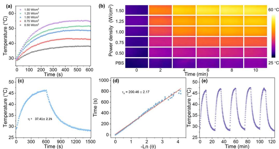
Fig. 3  $\text{Bi}_2\text{S}_3@\text{C}/\text{Fe}_3\text{O}_4$  NPs ( $0.5 \text{ mg mL}^{-1}$ ): (a) temperature-rise curve with variation of power density ( $0.5\text{--}1.5 \text{ W cm}^{-2}$ ). (b) Photothermal diagram at different power densities. (c) Photothermal conversion efficiency test ( $1 \text{ W cm}^{-2}$ ). (d) Relationship between cooling time and  $-\ln \theta$ . (e) Cycle stability ( $1 \text{ W cm}^{-2}$ ).
