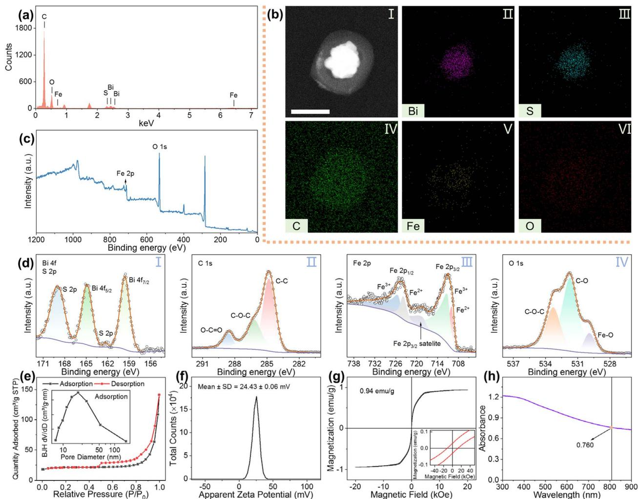
Fig. 2 (a) EDX spectrum, (b) elemental mapping images, (c) and (d) XPS profiles, (e)  $\text{N}_2$  adsorption/desorption isotherms (inset: pore-size distribution curves), (f) zeta potential distributions, (g) magnetization loop (inset: zoom-in M–H hysteresis curve), and (h) UV-vis-NIR absorption spectra of  $\text{Bi}_2\text{S}_3@\text{C}/\text{Fe}_3\text{O}_4$  NPs. Scale bar: 50 nm.
