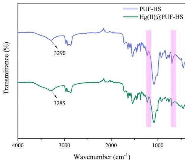
Fig. 14 FTIR analysis of PUF-HS and Hg(II)@PUF-HS.
