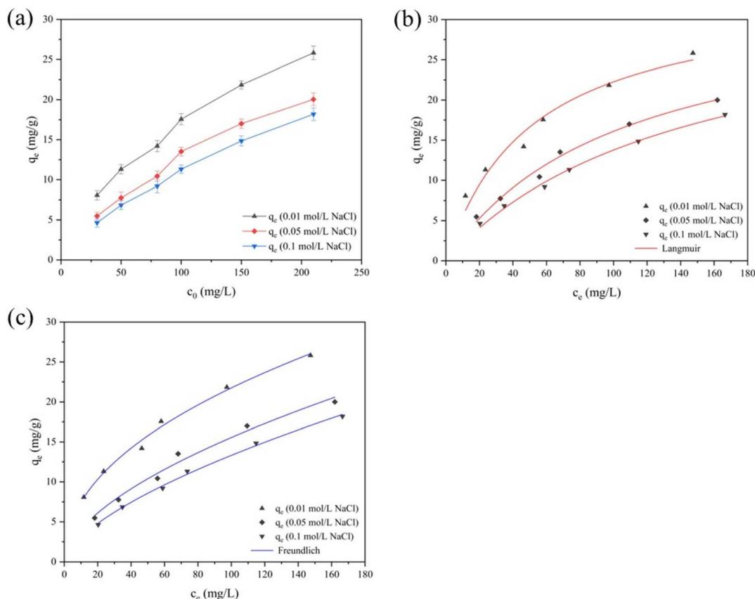
Fig. 12 Effect of ionic strength on Hg(II) adsorption by PUF-HS at 25 °C (a) adsorption isotherm models at different ionic strengths: (b) Langmuir and (c) Freundlich.
