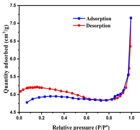
Fig. 3 Nitrogen adsorption–desorption isotherms for (a) NiONPs-BP and (b) CuONPs-BP.
