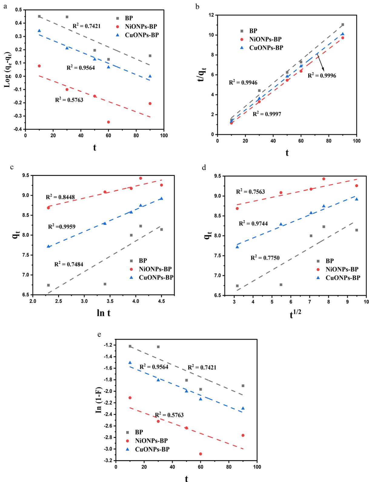
Fig. 7 (a) PFO, (b) PSO, (c) Elovich, (d) IPD and (e) LFD plots for MG uptake onto BP, NiONPs-BP and CuONPs-BP.
