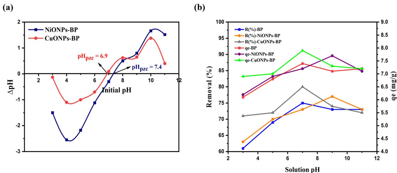
Fig. 4 (a) The pH point of zero charge and (b) effect of pH on adsorption of MG onto BP, NiONPs-BP and CuONPs-BP.
