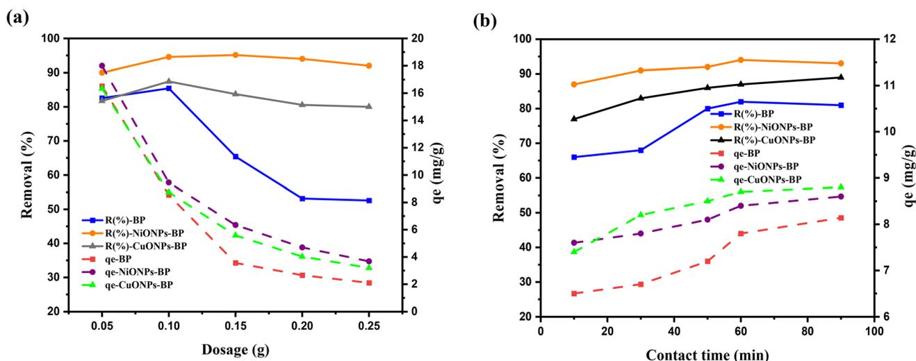
Fig. 5 Effect of (a) dosage and (b) contact time on the adsorption of MG onto BP, NiONPs-BP and CuONPs-BP.
