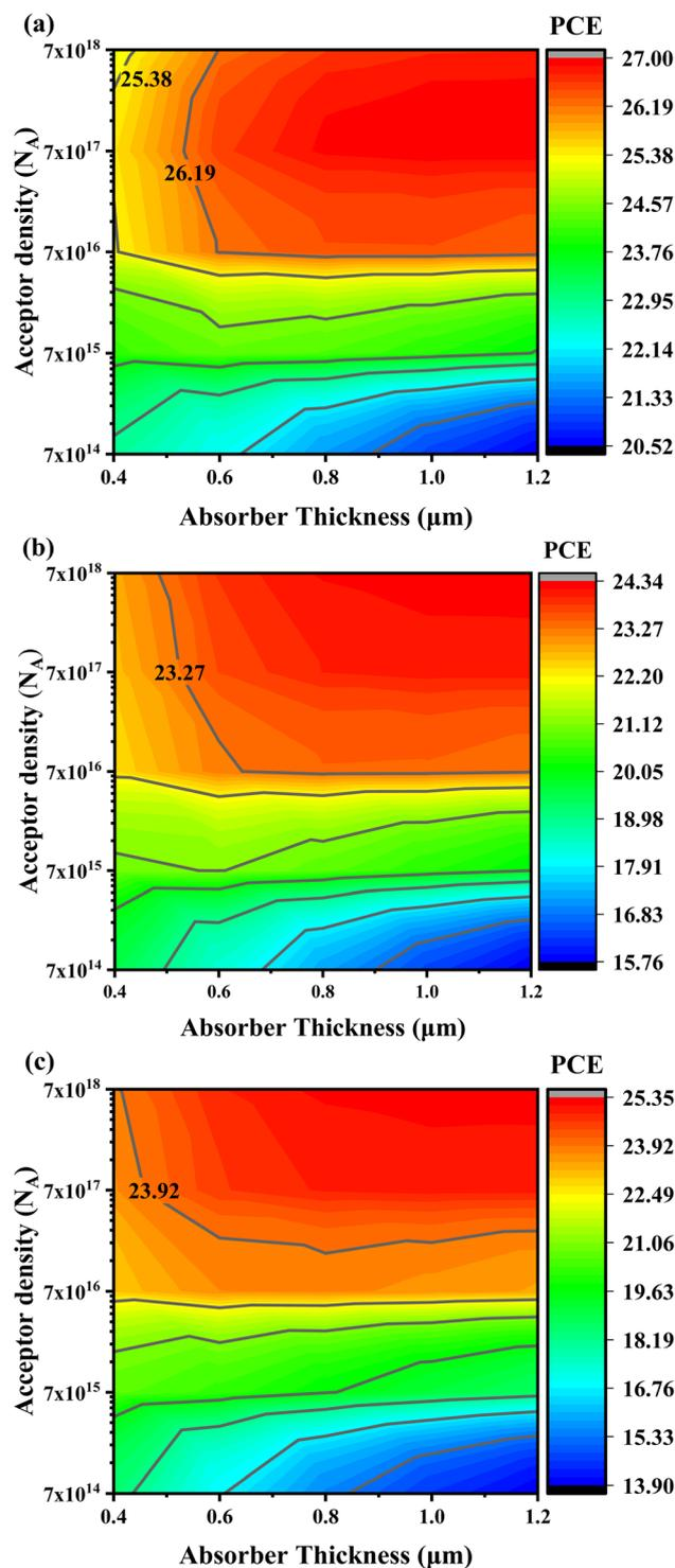
Fig. 11 Contour mapping of PCE showing the effects of varying in absorber thickness and  $N_A$  for ETLs including (a)  $WS_2$ , (b)  $C_{60}$ , and (c) PCBM.
