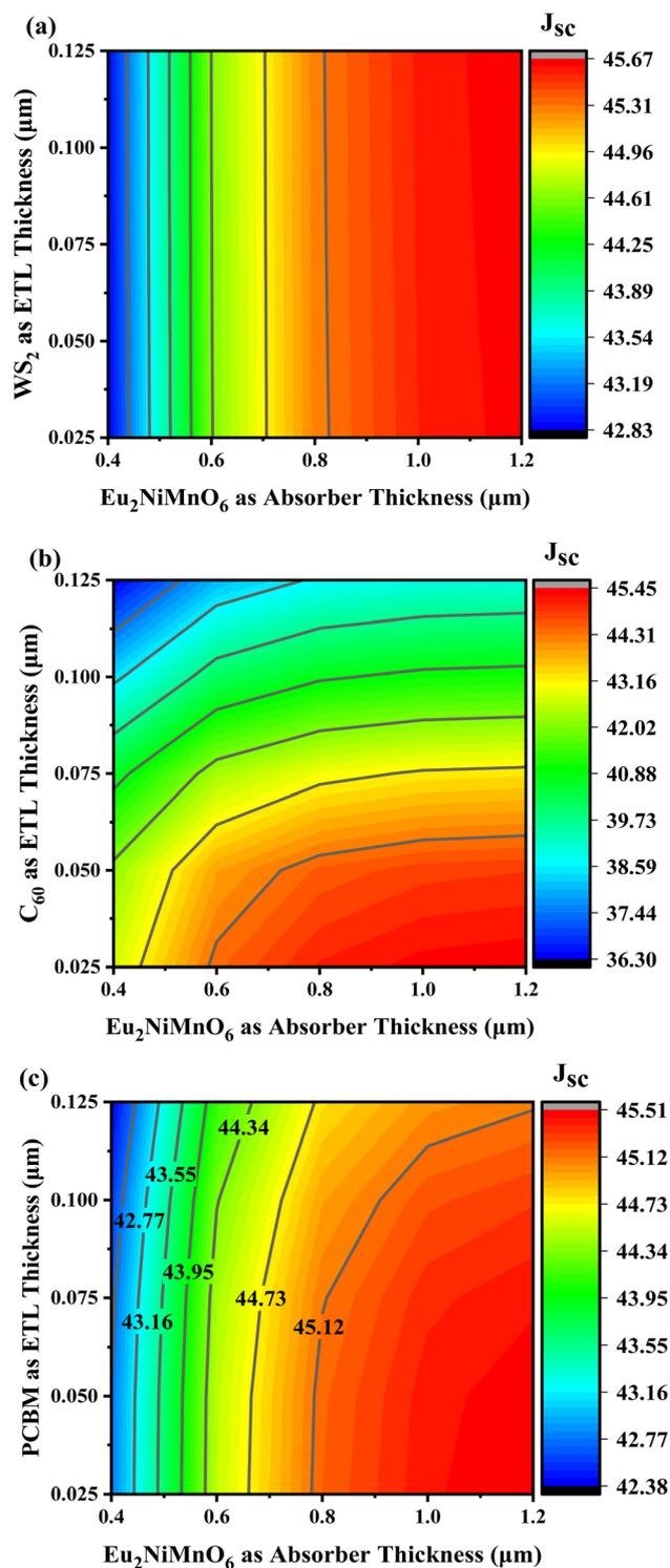
Fig. 5 Contour mapping of J<sub>SC</sub> shows effects of varying ETL and absorber thicknesses for ETLs including (a) WS<sub>2</sub>, (b) C<sub>60</sub>, and (c) PCBM.
