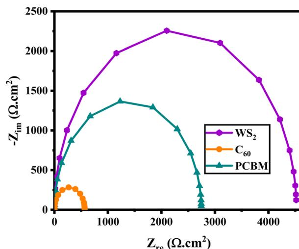
Fig. 18 Comparison of Nyquist plots for  $\text{Eu}_2\text{NiMnO}_6$  absorbers with different ETL materials ( $\text{WS}_2$ ,  $\text{C}_{60}$ ,  $\text{PCBM}$ ).
