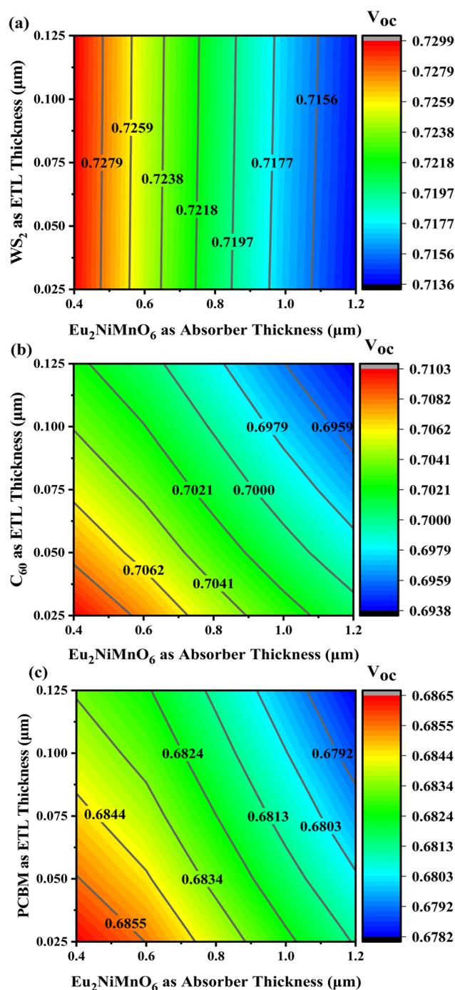
Fig. 4 Contour mapping of V<sub>OC</sub> shows effects of varying ETL and absorber thicknesses for ETLs including (a) WS<sub>2</sub>, (b) C<sub>60</sub>, and (c) PCBM.
