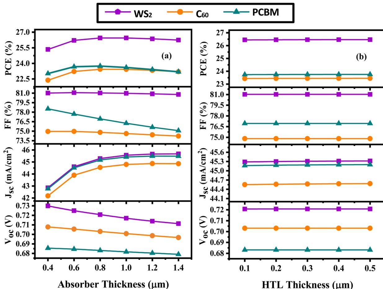
Fig. 12 Impact of varying (a) absorber thickness and (b) HTL thickness on PV parameters.
