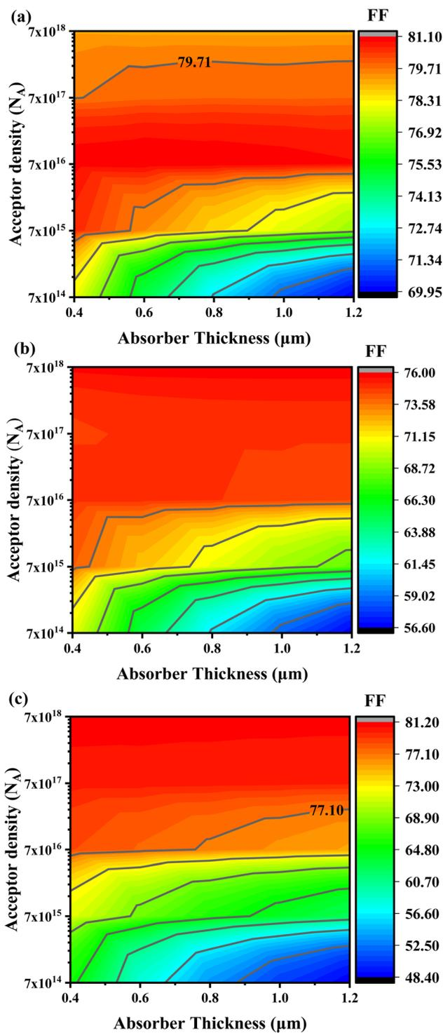
Fig. 10 Contour mapping of FF showing the effects of varying in absorber thickness and  $N_A$  for ETLs including (a)  $WS_2$ , (b)  $C_{60}$ , and (c) PCBM.
