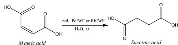
Fig. 7 The reduction reaction of MA to SA.
