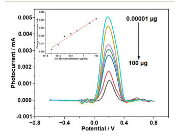
Fig. 3 The DPV voltammograms (in the presence of light) of the fabricated immunosensor incubated with different CA 125 concentrations: 100, 10, 0.1, 0.01, 0.001, 0.0001 and 0.00001  $\mu g$  mL<sup>-1</sup> of CA 125 in 10 mmol L<sup>-1</sup> [Fe(CN)<sub>6</sub>]<sup>3-/4-</sup> solution containing 0.1 M KCl and 0.01 M AA.
