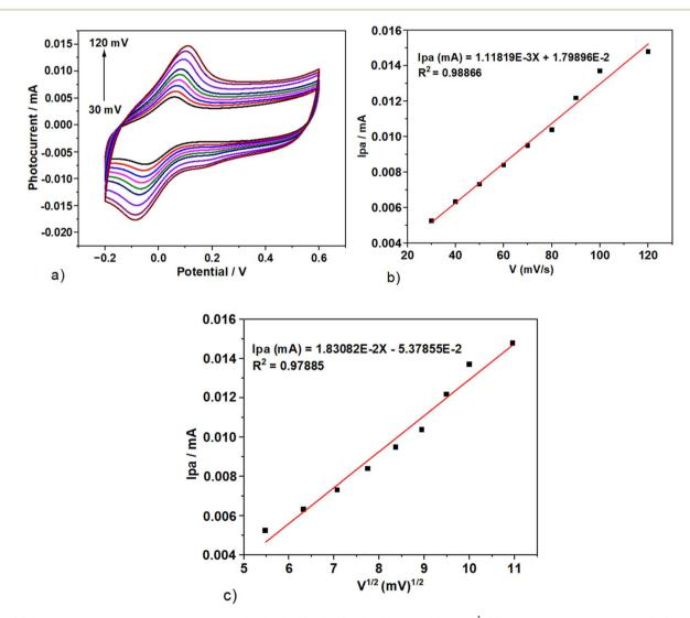
Fig. 2 (a) Cyclic voltammograms at scan rates of 30, 40, 50, 60, 70, 80, 90, 100, and 120 mV s<sup>-1</sup>; (b) plot of anodic peak current ( $I_{pa}$ ) versus the scan rate ( $V_{pa}$ ) versus the square root of the scan rate ( $V_{pa}$ ).
