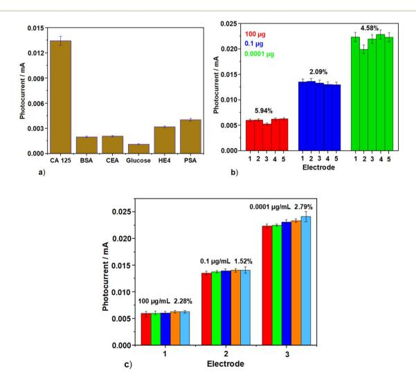
Fig. 4 (a) Selectivity test in the presence of interferents; (b) reproducibility studies; (c) repeatability studies by DPV in the presence of 10 mmol  $L^{-1}$ [Fe(CN)<sub>6</sub>]<sup>3-/4-</sup> solution containing 0.1 M KCl and 0.01 M AA.
