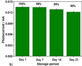
Fig. 5 (a) Stability test under several on/off irradiation cycles of 15 seconds each. (b) Stability test of the CA 125 immunosensor over 21 days for the detection of 0.1  $\mu$ g CA 125 antigen by DPV in the presence of 10 mmol L<sup>-1</sup> [Fe(CN)<sub>6</sub>]<sup>3-/4-</sup> solution containing 0.1 M KCl and 0.01 M ascorbic
