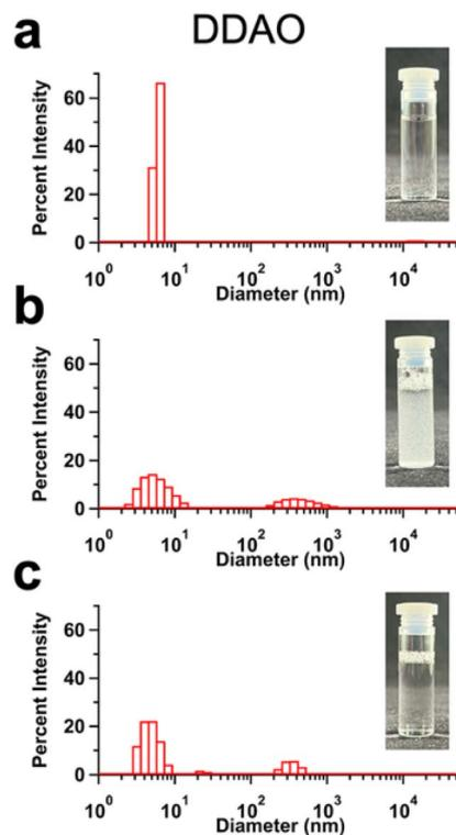
Fig. 7 DLS measurements of 5% (w v<sup>-1</sup>) DDAO with the addition of CEES after (a) 0 min, (b) 24 min, and (c) 60 min. (Insets) Photos of mixtures.
