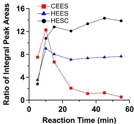
Fig. 6 Ratios of <sup>1</sup>H-NMR integral peak areas of CEES, HEES, and HESC to that of EG in an aqueous mixture of CEES in 5% (w v<sup>-1</sup>) DDAO with 2% (w v<sup>-1</sup>) EG over time.
