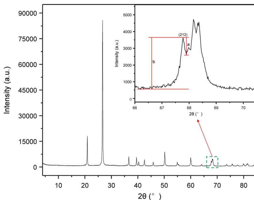
Fig. 2 Powder XRD pattern of sample 2 (200-mesh powder). The inset enlarges the (212) reflection at  $2\theta = 67.75^\circ$ , used to calculate the Crystallinity Index (CI) following Murata and Norman.<sup>21</sup> Peak height ( $a$ ) and total peak height above background ( $b$ ) are indicated; CI values are normalised using scaling factor  $F = 1.12$ .
