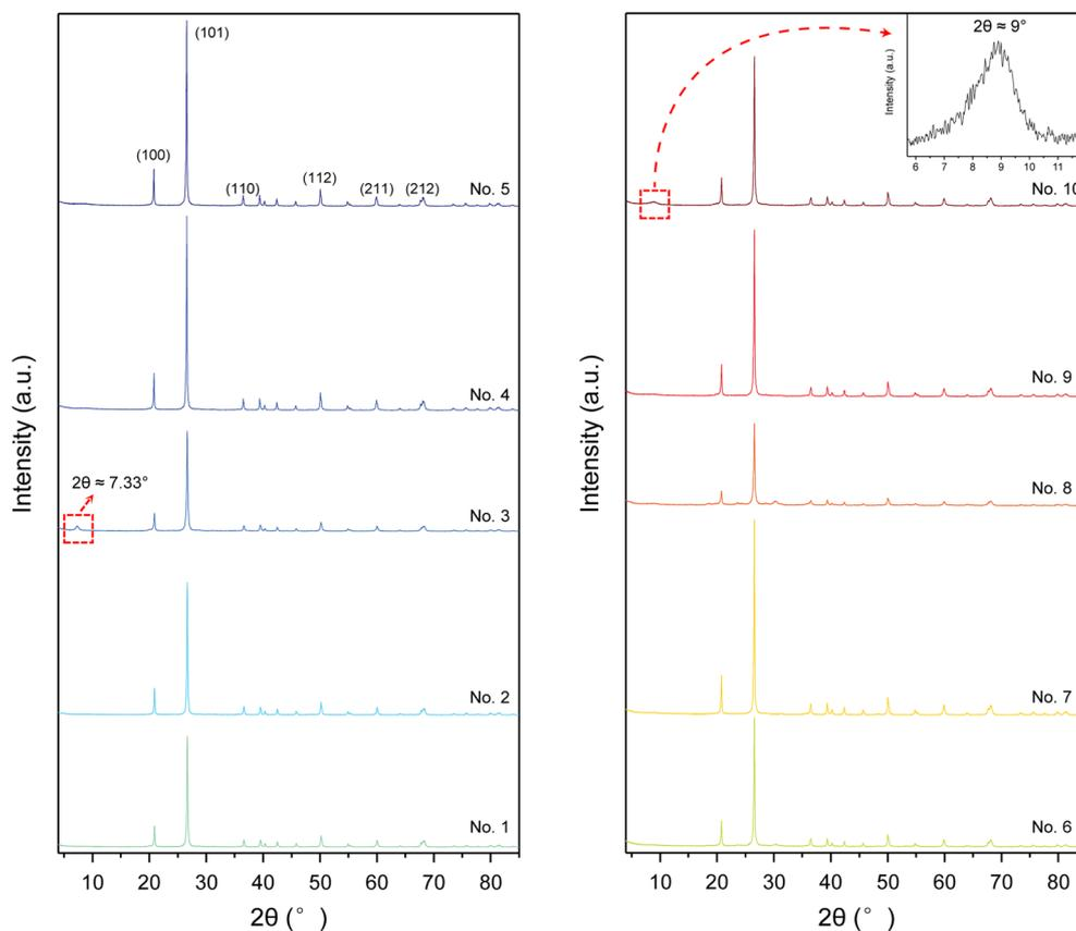
Fig. 3 XRD patterns of ten chrysoprase samples, consistent with the  $\alpha$ -quartz reference (PDF #86-2237). Minor peaks marked by red boxes indicate possible secondary phases or impurities—for example, the sharp  $\sim 7.33^\circ$  peak in sample 3 (assigned to sepiolite) and a broad weak reflection near  $d \approx 10$  Å in sample 10, consistent with poorly crystalline Ni-bearing phyllosilicates.
