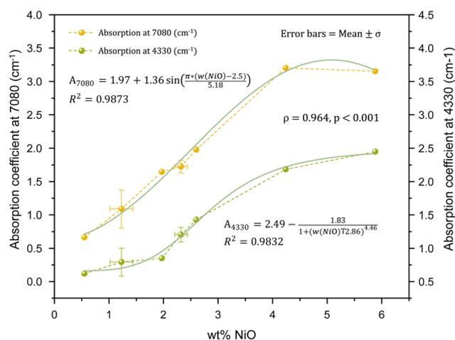
Fig. 7 Correlation between NiO content and NIR absorption coefficients at  $7080\text{ cm}^{-1}$  and  $4330\text{ cm}^{-1}$  in chrysoprase samples. Both bands, attributed to Ni–OH vibrational modes, show very strong positive correlations with Ni content ( $\rho = 0.964$ ,  $p < 0.001$ ). Error bars represent mean  $\pm$  standard deviation.
