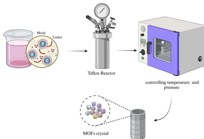
Fig. 1 Schematic of the hydrothermal/solvothermal synthesis of MOFs.
