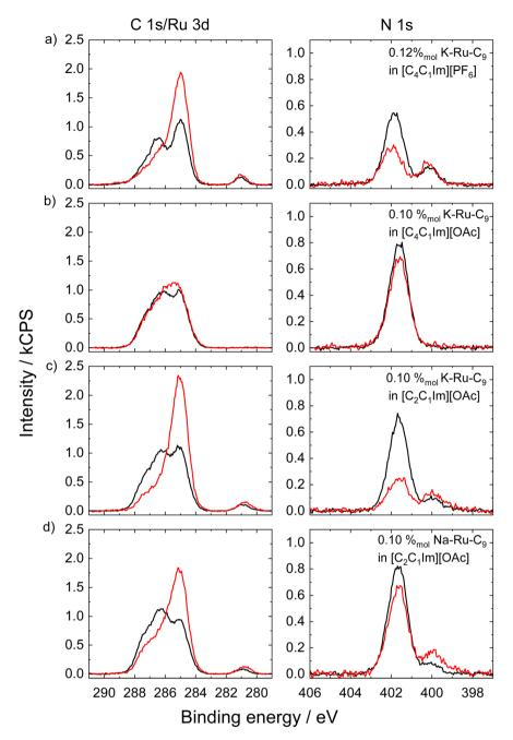
Fig. 4 XP spectra at 0° (black) and 80° (red) for the C 1s/Ru 3d (left) and N 1s (right) regions for (a)  $0.12\%_{mol}$  solution of K-Ru-C<sub>9</sub> complexes in  $[C_4C_1Im][PF_6]$ ,  $0.10\%_{mol}$  solution of (b) K-Ru-C<sub>9</sub> in  $[C_4C_1Im][OAc]$ , (c) K-Ru-C<sub>9</sub> in  $[C_2C_1Im][OAc]$ , and (d) Na-Ru-C<sub>9</sub> in  $[C_2C_1Im][OAc]$  (adapted from ref. 25, with permission).
