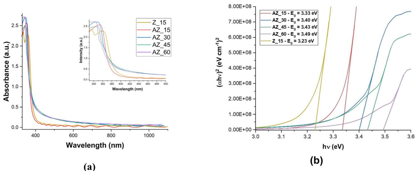
Fig. 3 (a) UV-Vis absorption spectra of ZnO and AZO thin films deposited at different sputtering power. (b) Estimated optical band gap ( $E_g$ ) values of ZnO and AZO films as a function of sputtering power.
