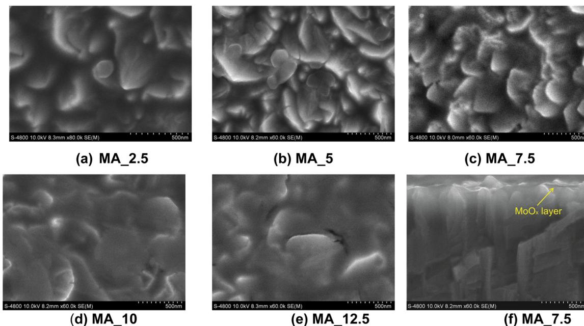
Fig. 9 (a)–(e) SEM images of the MA\_2.5, MA\_5, MA\_7.5, MA\_10, and MA\_12.5 samples. (f) The cross-sectional SEM image of the MA\_7.5 sample.
