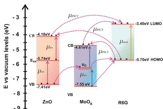
Fig. 15 Schematic diagram of CT between R6G and the MoO<sub>x</sub>/AZO SERS substrate.
