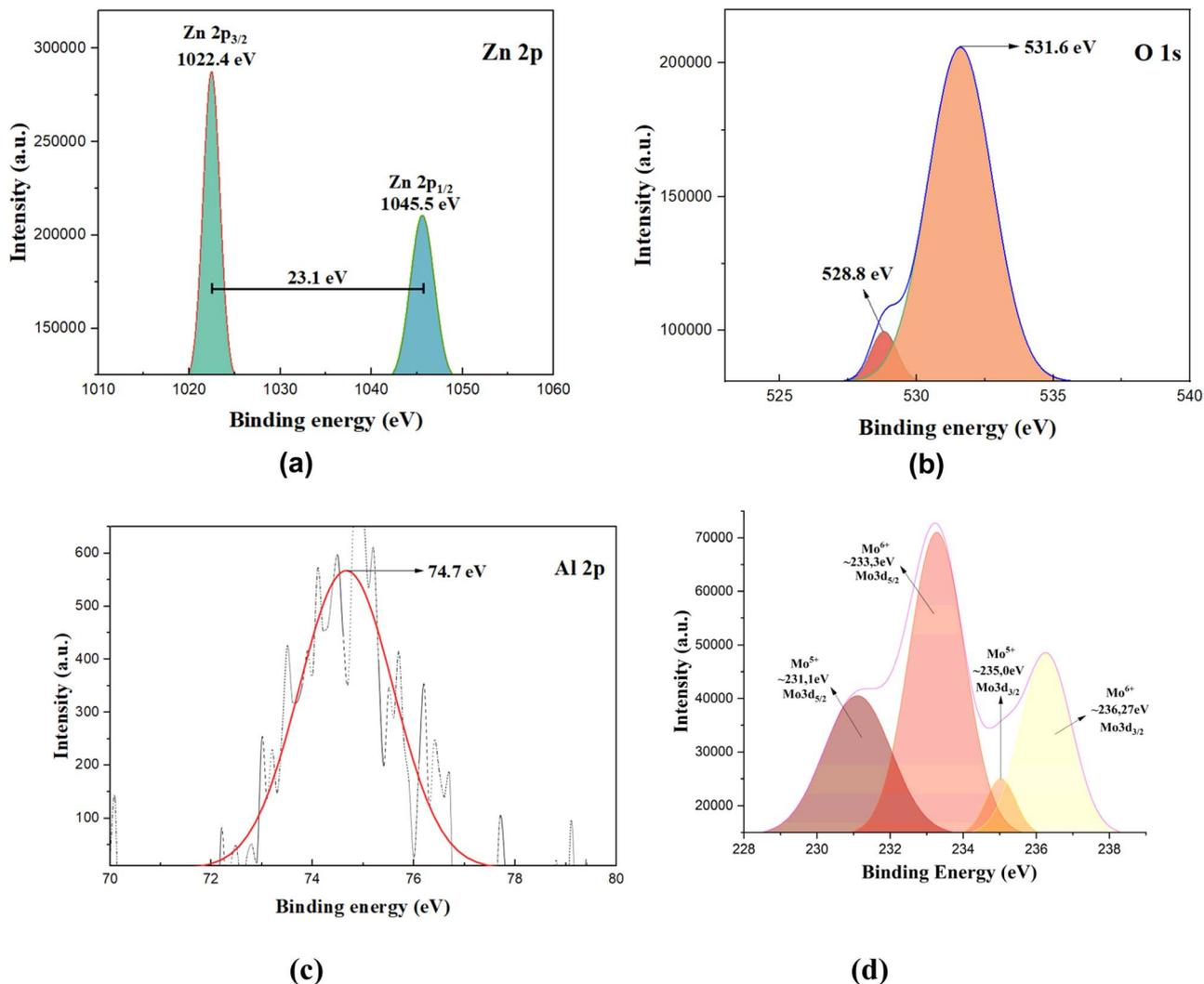
Fig. 12 High-resolution XPS spectra of the MA<sub>7.5</sub> sample: (a) Zn 2p spectrum; (b) O 1s spectrum; (c) Al 2p spectrum; (d) Mo 3d spectrum.
