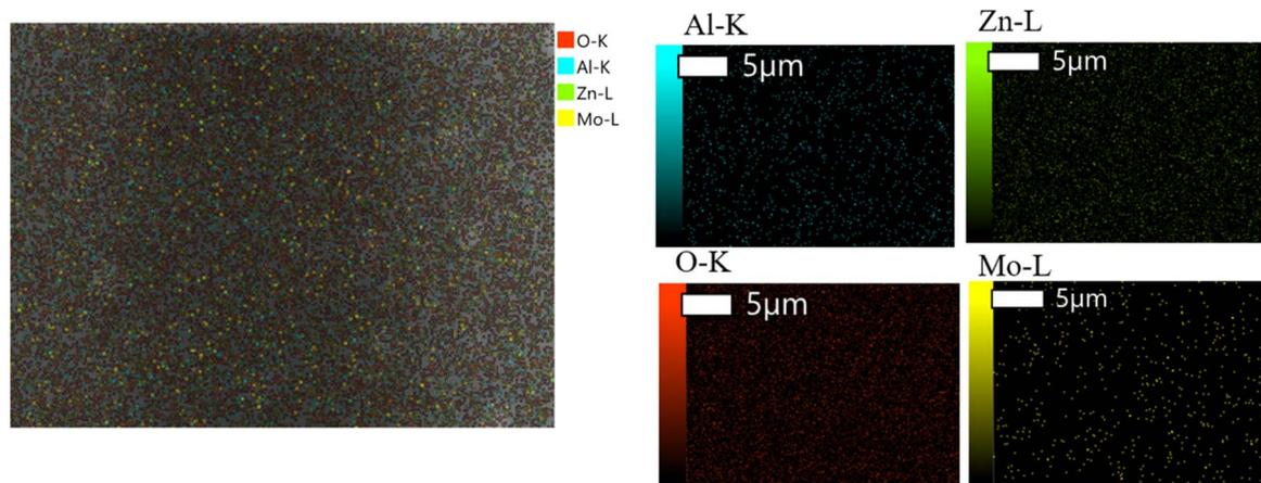
Fig. 10 EDS mapping image and individual elemental EDX analysis of the MA<sub>7.5</sub> sample.
