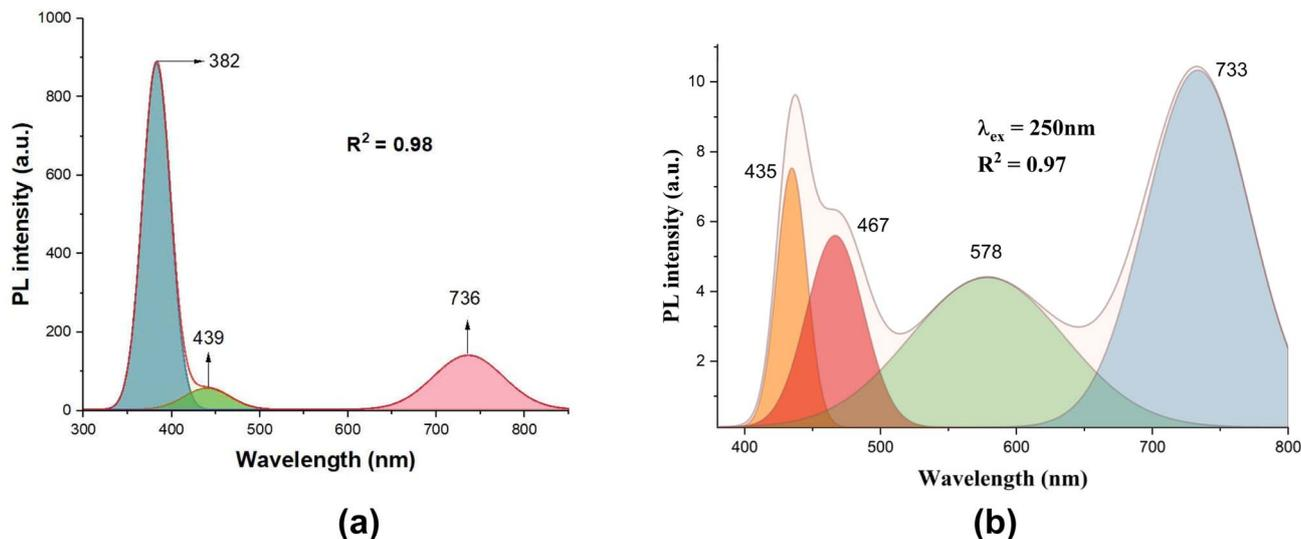
Fig. 11 Gaussian deconvolution PL spectrum of (a) AZ\_45 and (b) MA\_7.5 sample.
