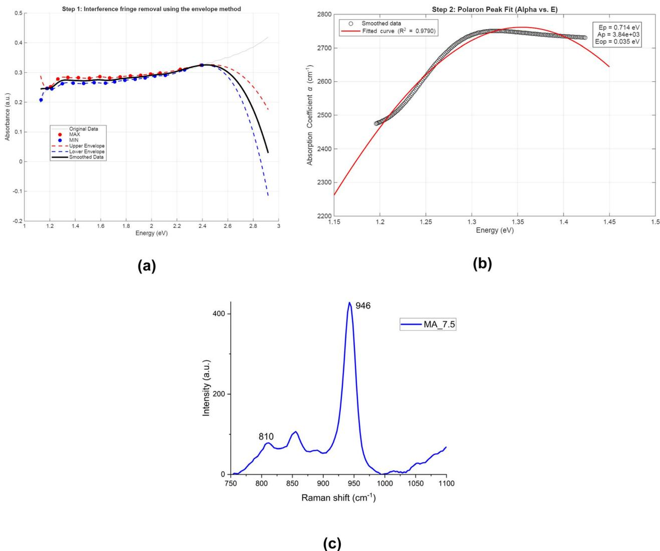
Fig. 14 (a) Interference fringe removal using envelope method. (b) Fit polaron peak using Gaussian according to Holstein model. (c) Raman spectra of MA<sub>7.5</sub> ranging from 750 cm<sup>-1</sup> to 1100 cm<sup>-1</sup>.
