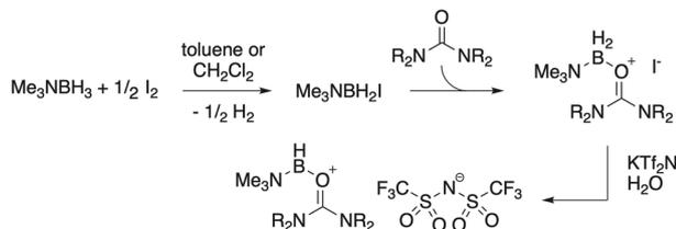
Fig. 3 General synthesis of the new urea-ligated boronium salts.
