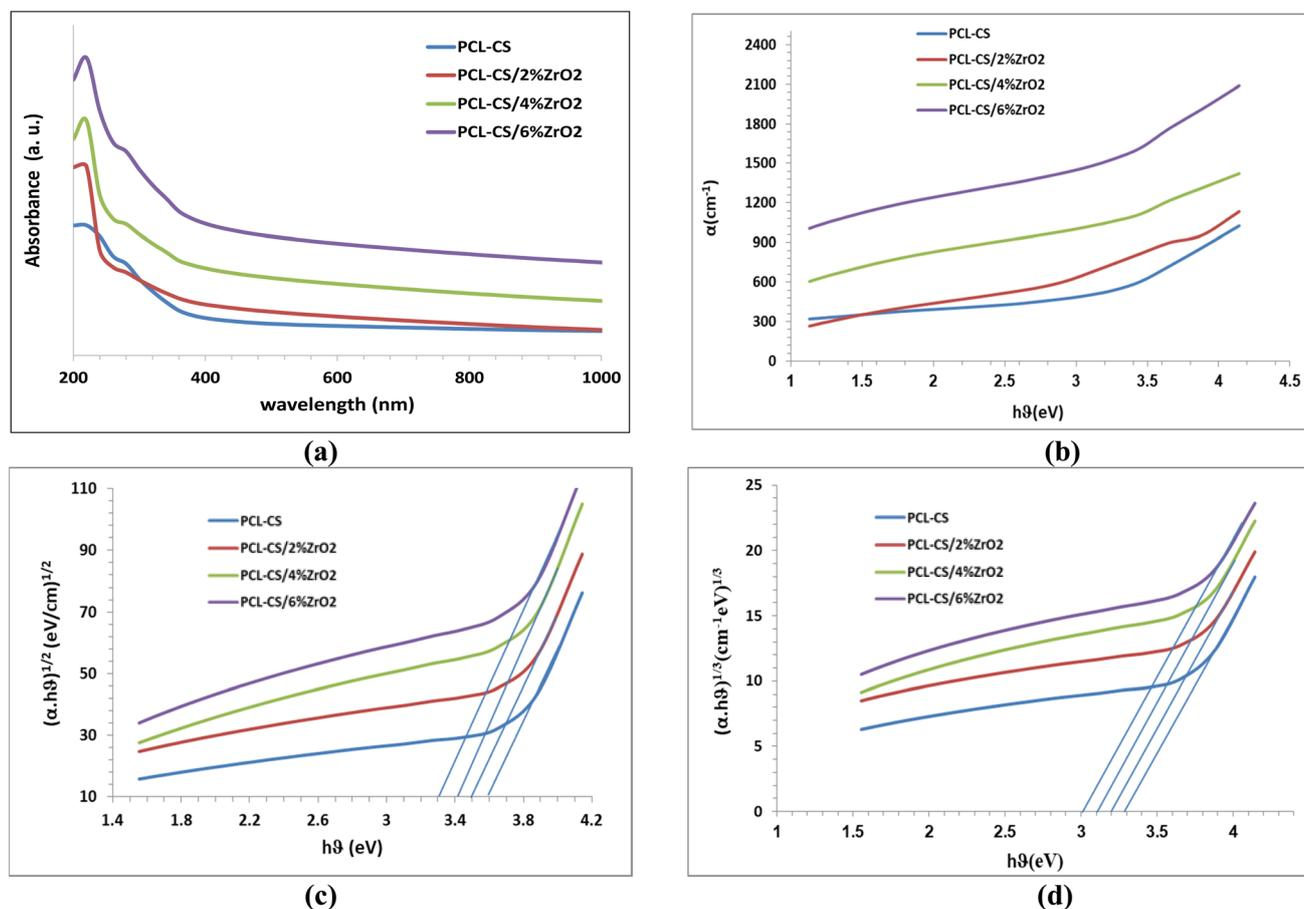
Fig. 7 Optical properties of PCL-CS/ZrO<sub>2</sub> nanocomposites: (a) evolution of absorbance along with wavelength, (b) absorption coefficient ( $\alpha$ ), (c)  $(\alpha h\nu)^{1/2}$ , and (d)  $(\alpha h\nu)^{1/3}$  variation as a function of photon energy ( $h\nu$ ).
