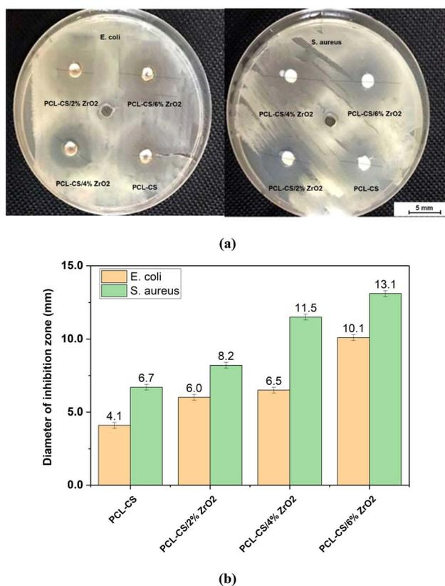
Fig. 9 Antibacterial behavior of CS-PCL/ZrO<sub>2</sub> nanocomposites against the bacteria strains of *E. coli* and *S. aureus*: (a) opticat image of agar plates and (b) diameter inhibition zone for each nanocomposite content.
