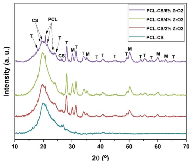
Fig. 1 XRD patterns of PCL-CS/ZrO<sub>2</sub> nanocomposite films with different ZrO<sub>2</sub> concentrations (0%, 2%, 4%, and 6%).
