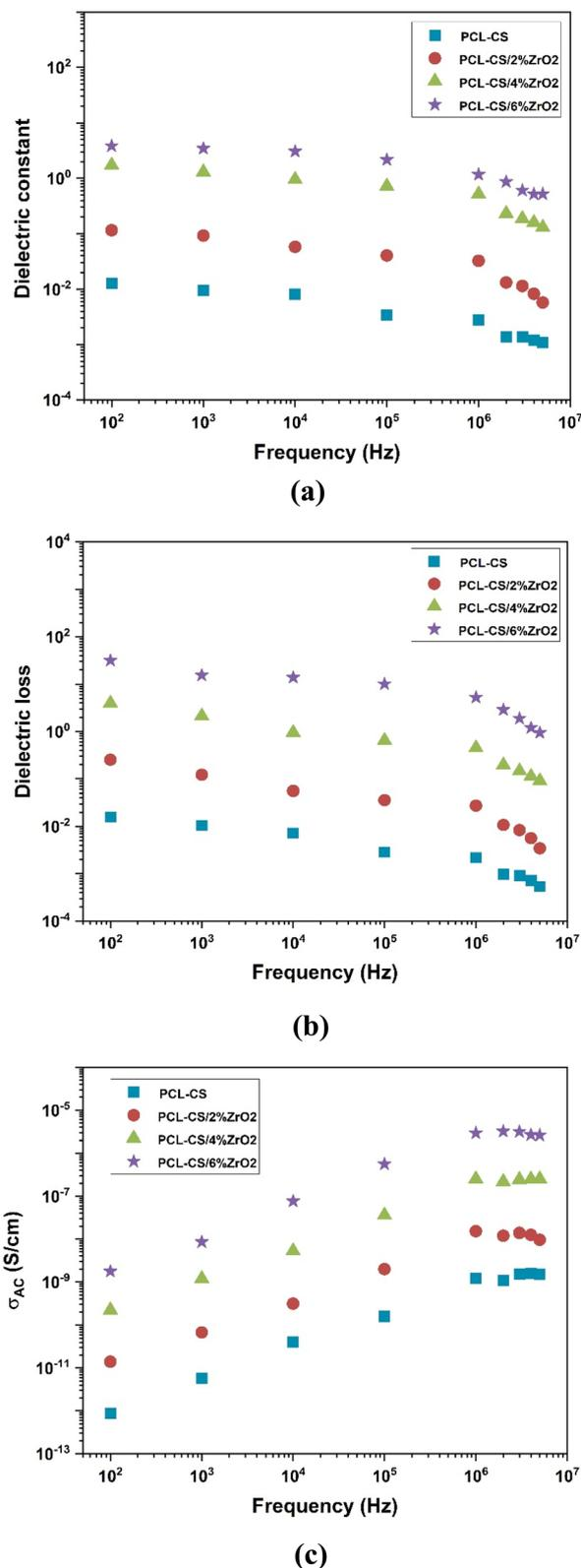
Fig. 6 Dielectric properties for PCL-CS/ZrO<sub>2</sub> nanocomposites: (a) dielectric constant, (b) dielectric loss, and (c) AC electrical conductivity.
