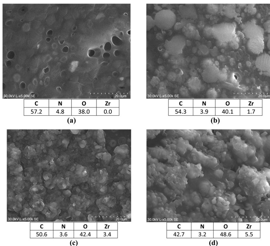
Fig. 3 SEM micrographs and EDS chemical analysis of PCL-CS/ZrO<sub>2</sub> nanocomposite films: (a) 0 wt%, (b) 2 wt%, (c) 4 wt%, and (d) 6 wt%.
