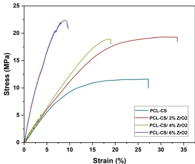
Fig. 4 Stress–strain curves obtained for different PCL-CS/ZrO<sub>2</sub> nanocomposite films.
