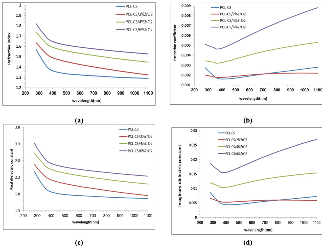
Fig. 8 Optical properties of PCL-CS/ZrO<sub>2</sub> nanocomposites: (a) refractive index, (b) extinction coefficient, (c) real part of dielectric constant, and (d) imaginary part for dielectric constant.
