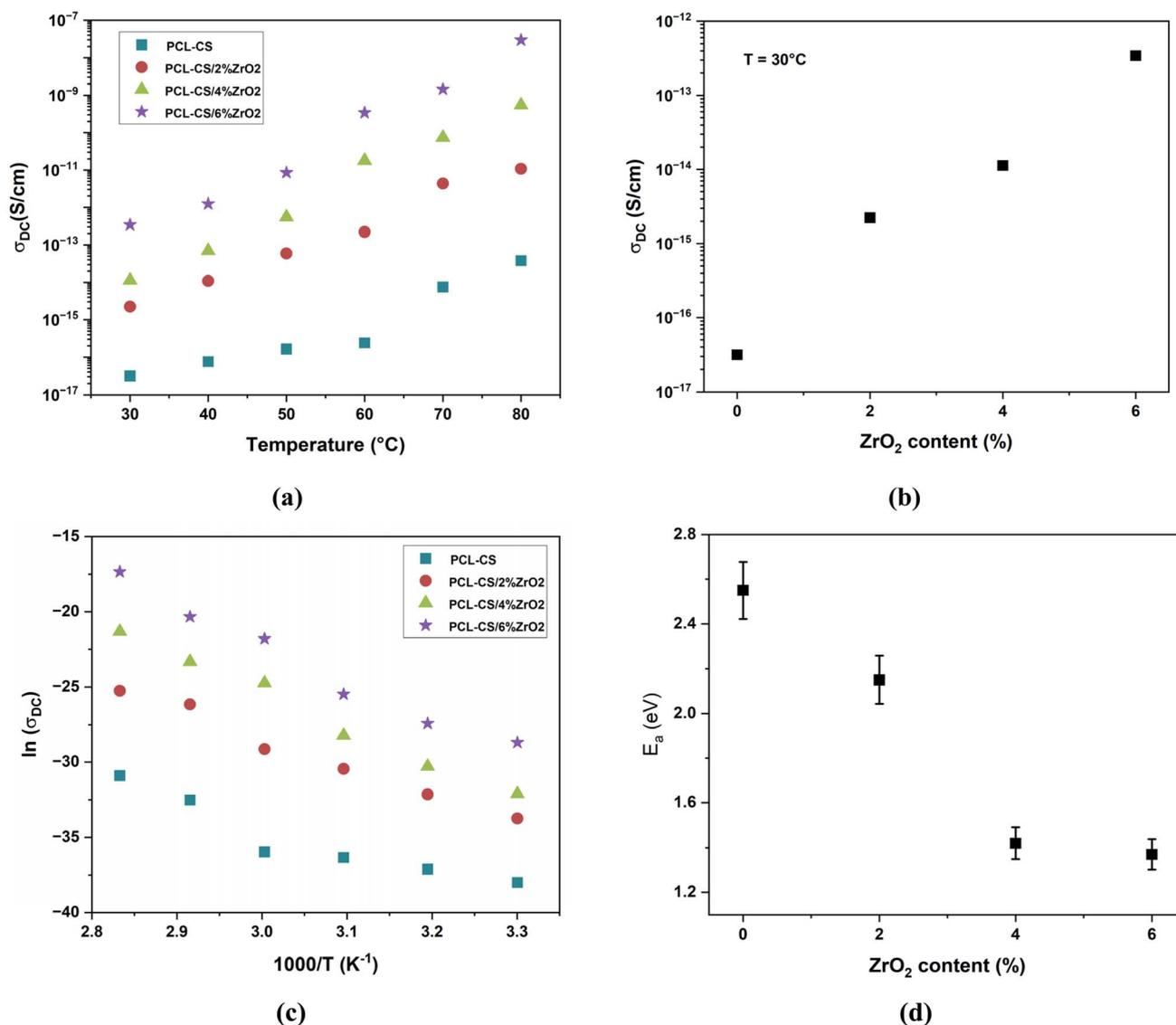
Fig. 5 DC electrical properties of PCL-CS and PCL-CS/ $\text{ZrO}_2$  nanocomposite films: (a) electrical conductivity with temperature, (b) electrical conductivity with  $\text{ZrO}_2$  contents, (c) plot of  $\ln(\sigma_{\text{DC}})$  versus inverted absolute temperature, and (d) thermal activation energy.
