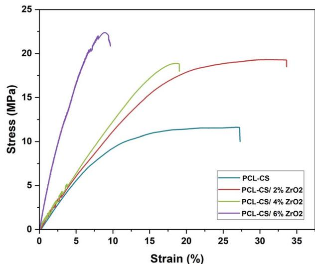
Fig. 4 Stress–strain curves obtained for different PCL-CS/ZrO<sub>2</sub> nanocomposite films.
