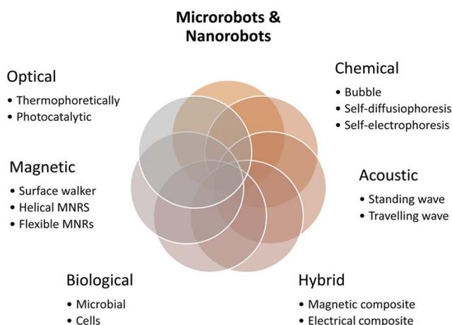
Fig. 5 Different types of Biohybrid nanorobots that can be controlled through proper actuation to accomplish specific tasks, Reprinted from ref. 49 Copyright 2024, RSC.
