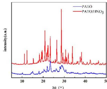
Fig. 3 X-ray diffraction patterns of PATO and PATO-N.
