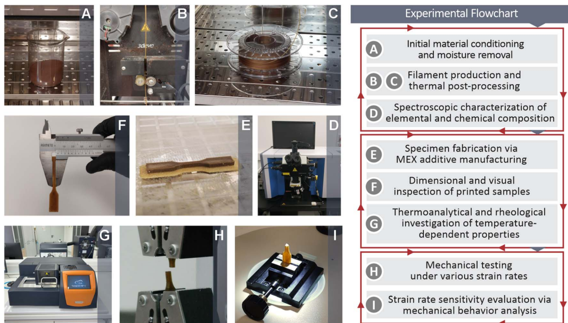
Fig. 1 Pictures revealing the procedures of this research (left side) and the respective experimental flowchart (right side): (A) PI material conditioning and removal of the existing moisture, (B) and (C) filament extrusion and thermal post-processing, (D) elemental and chemical composition through stereoscopic characterization, (E) MEX AM specimen printing, (F) dimension measuring and visual inspection of the specimens, (G) thermo-analytical and rheological investigation of the properties depended from temperature, (H) mechanical performance examination through testing under different strain rates, (I) analysis of the mechanical behavior aiming strain rate sensitivity evaluation.
