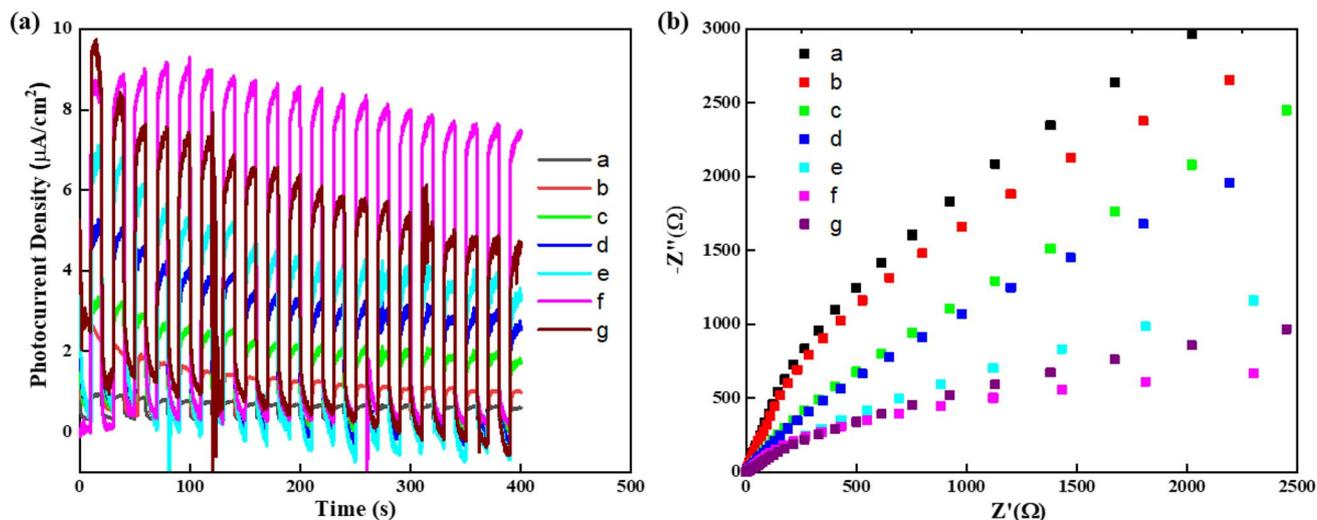
Fig. 4 (a) Transient photocurrent response curves and (b) EIS Nyquist plots of all the samples. (a)  $\gamma$ - $\text{In}_2\text{Se}_3$ ; (b)  $\gamma$ - $\text{In}_2\text{Se}_3/\text{MoS}_2$ ; (c–g)  $\gamma$ - $\text{In}_2\text{Se}_3/\text{MoS}_2/\text{graphene}$  composites with the graphene amount of 1%, 2%, 3%, 4%, and 5%, respectively.)
