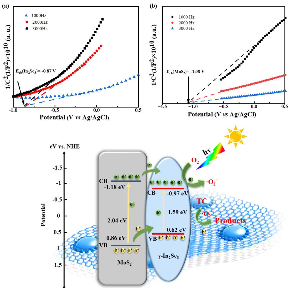
Fig. 7 Mott-Schottky curves of (a)  $\gamma$ -In<sub>2</sub>Se<sub>3</sub> and (b) MoS<sub>2</sub>. (c) Proposed mechanism of charge transfer for the photocatalytic degradation of TC by the  $\gamma$ -In<sub>2</sub>Se<sub>3</sub>/MoS<sub>2</sub>/graphene composite.
