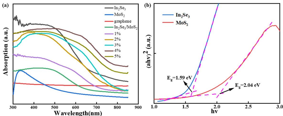
Fig. 3 (a) Absorbance spectra for  $\gamma$ - $\text{In}_2\text{Se}_3$ ,  $\text{MoS}_2$ , and the  $\gamma$ - $\text{In}_2\text{Se}_3/\text{MoS}_2/\text{graphene}$  composites (1%, 2%, 3%, 4%, and 5% represents the amount of graphene in the  $\gamma$ - $\text{In}_2\text{Se}_3/\text{MoS}_2/\text{graphene}$  composites, respectively); (b) bandgap curves of  $\gamma$ - $\text{In}_2\text{Se}_3$  and  $\text{MoS}_2$ .
