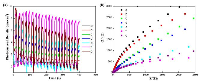
Fig. 4 (a) Transient photocurrent response curves and (b) EIS Nyquist plots of all the samples. (a)  $\gamma - \ln_2 Se_3$ ; (b)  $\gamma - \ln_2 Se_3$ /MoS<sub>2</sub>; (c-g)  $\gamma - \ln_2 Se_3$ /MoS<sub>2</sub>/graphene composites with the graphene amount of 1%, 2%, 3%, 4%, and 5%, respectively.)
