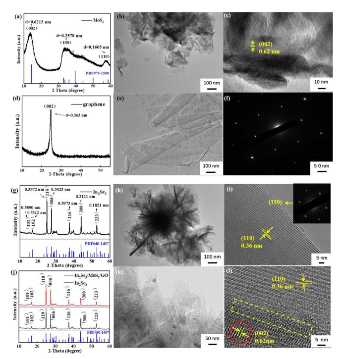
Fig. 1 (a) X-ray diffraction (XRD) pattern, (b) TEM and (c) HRTEM image of MoS<sub>2</sub> nanoplates; (d) XRD pattern, (e) TEM and (f) SEAD image of graphene; (g) XRD pattern of  $\gamma$ -In<sub>2</sub>Se<sub>3</sub>; (h) TEM and (i) HRTEM of  $\gamma$ -In<sub>2</sub>Se<sub>3</sub>, with SEAD pattern inserted in 2 (i); (j) XRD pattern, (k) TEM and (l) HRTEM of  $\gamma$ -In<sub>2</sub>Se<sub>3</sub>/MoS<sub>2</sub>/graphene composite.
