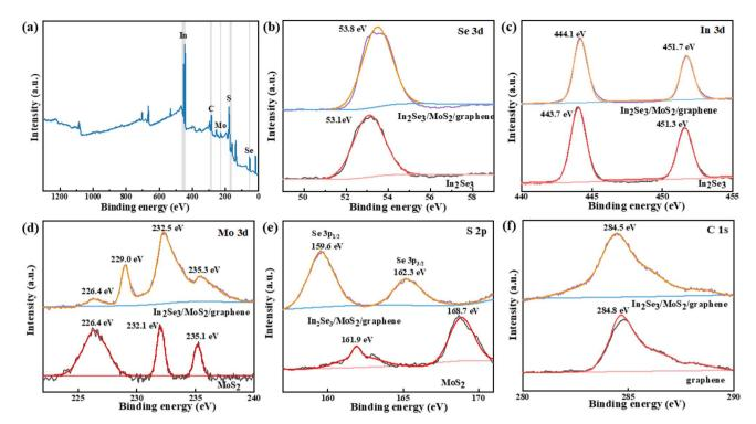
Fig. 2 High-resolution XPS spectra of  $\gamma$ -In<sub>2</sub>Se<sub>3</sub>/MoS<sub>2</sub>/graphene composite: (a) survey spectrum, (b) Se 3d, (c) In 3d, (d) Mo 3d, (e) S 2p and (f) C 1s. Related XPS results of  $\gamma$ -In<sub>2</sub>Se<sub>3</sub>, MoS<sub>2</sub> and graphene are used as references.
