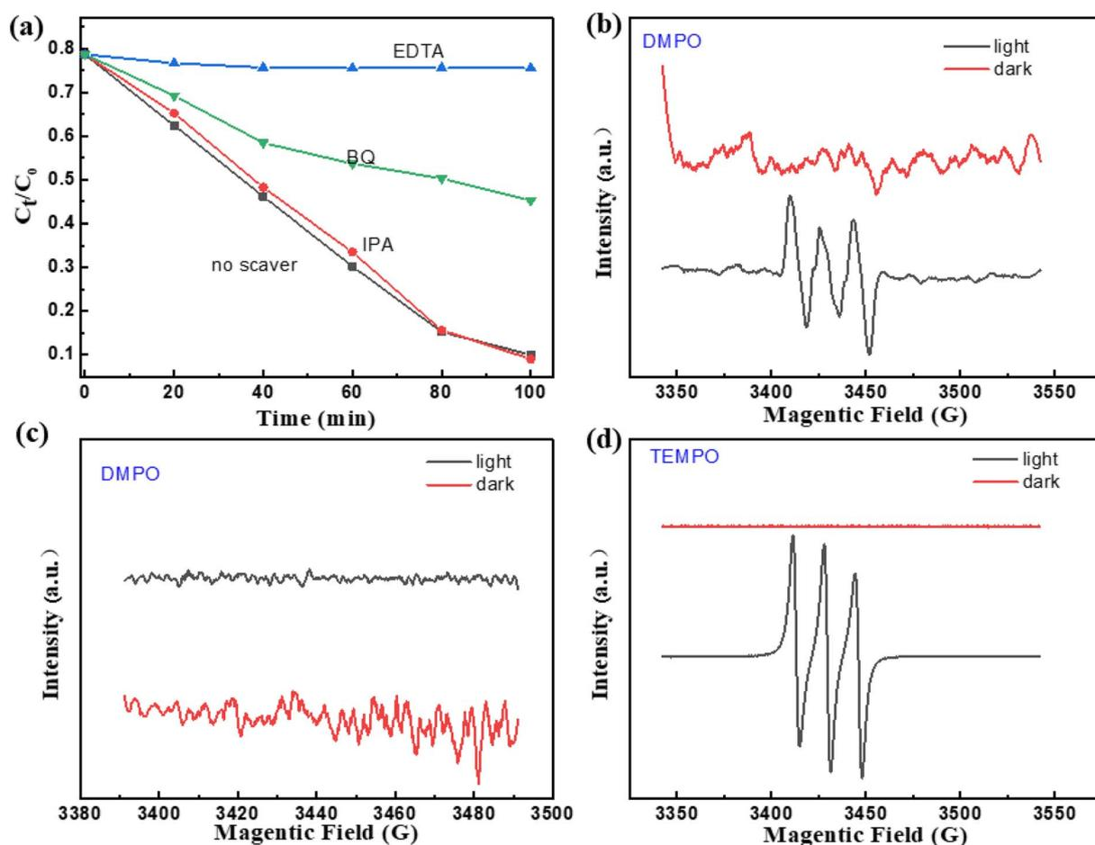
Fig. 6 (a) Effect of quenching reagents on TC degradation; (b) DMPO- $\cdot\text{O}_2^-$  and (c) DMPO- $\cdot\text{OH}$  with irradiation for 30 s in methanol and aqueous dispersion, respectively. (d) TEMPO- $\text{h}^+$  with irradiation for 30 s in methanol.
