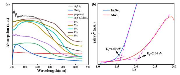
Fig. 3 (a) Absorbance spectra for  $\gamma$ -In<sub>2</sub>Se<sub>3</sub>, MoS<sub>2</sub>, and the  $\gamma$ -In<sub>2</sub>Se<sub>3</sub>/MoS<sub>2</sub>/graphene composites (1%, 2%, 3%, 4%, and 5% represents the amount of graphene in the  $\gamma$ -In<sub>2</sub>Se<sub>3</sub>/MoS<sub>2</sub>/graphene composites, respectively); (b) bandgap curves of  $\gamma$ -In<sub>2</sub>Se<sub>3</sub> and MoS<sub>2</sub>.
