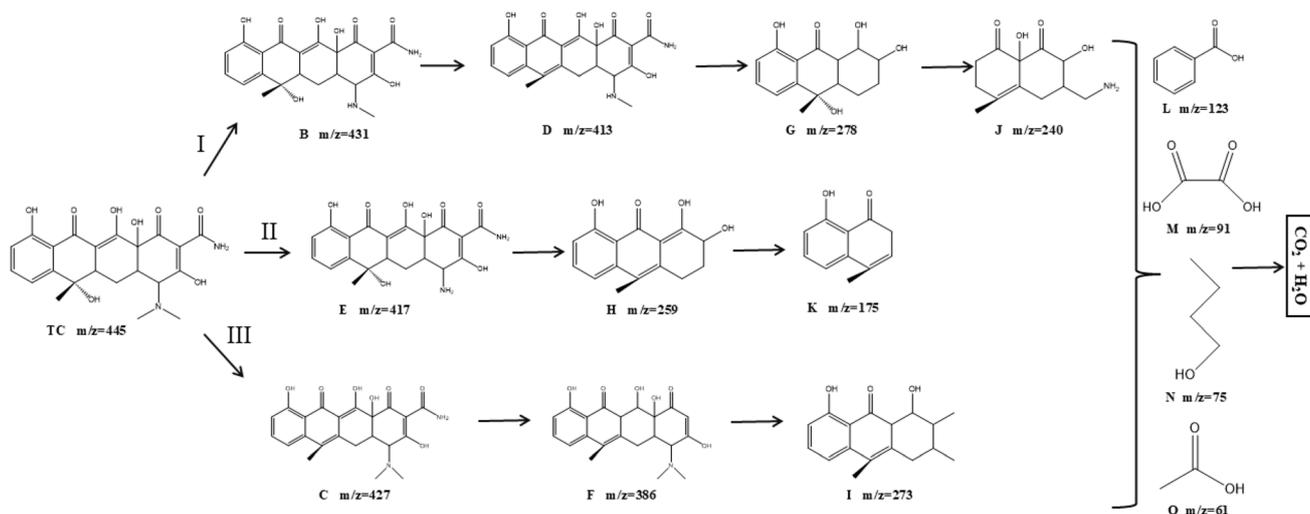
Fig. 8 Proposed TC degradation pathway in the  $\gamma$ -In<sub>2</sub>Se<sub>3</sub>/MoS<sub>2</sub>/graphene composite system.
