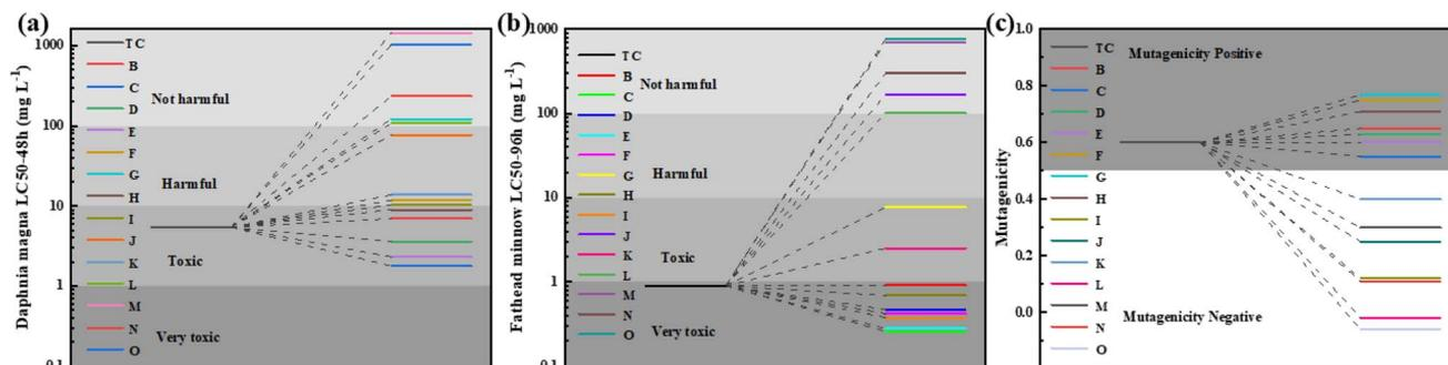
Fig. 9 (a) *Daphnia magna* LC<sub>50</sub>-48h of TC and degradation intermediates; (b) fathead minnow LC<sub>50</sub>-96h of TC and degradation intermediates; (c) mutagenicity of TC and degradation intermediates.
