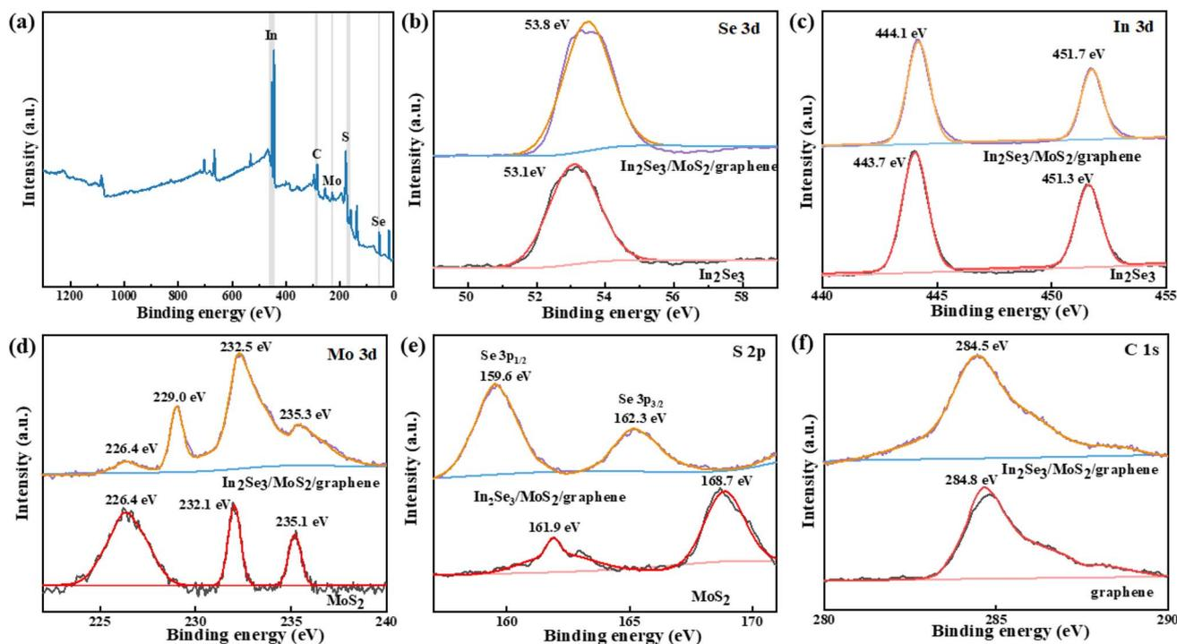
Fig. 2 High-resolution XPS spectra of  $\gamma$ - $\text{In}_2\text{Se}_3/\text{MoS}_2/\text{graphene}$  composite: (a) survey spectrum, (b) Se 3d, (c) In 3d, (d) Mo 3d, (e) S 2p and (f) C 1s. Related XPS results of  $\gamma$ - $\text{In}_2\text{Se}_3$ ,  $\text{MoS}_2$  and graphene are used as references.
