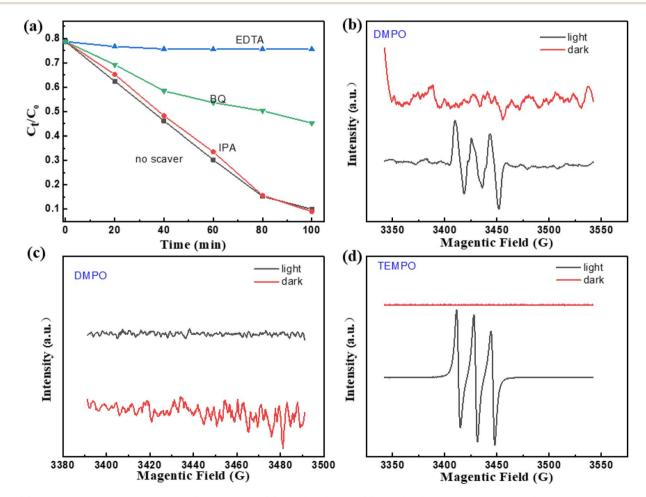
Fig. 6 (a) Effect of quenching reagents on TC degradation; (b) DMPO- $\cdot$ O<sub>2</sub> and (c) DMPO- $\cdot$ OH with irradiation for 30 s in methanol and aqueous dispersion, respectively. (d) TEMPO-h<sup>+</sup> with irradiation for 30 s in methanol.
