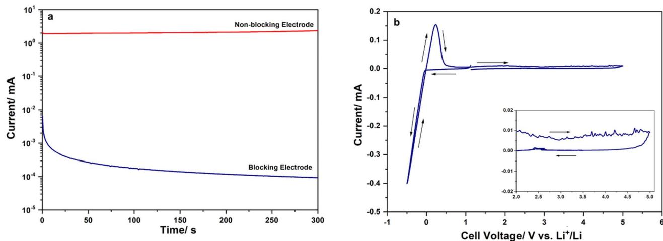
Fig. 6 (a) Change in DC with time when a voltage of 0.5 V (DC) was applied to the S-250 sample; (b) cyclic voltammogram of S-250 obtained at a scan rate of 5 mV s<sup>-1</sup> between 0.5 and 5 V.
