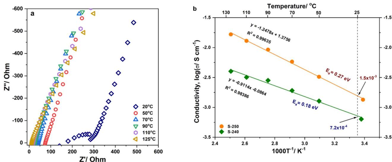
Fig. 5 (a) The impedance spectra of S-250 obtained at various temperatures from around room temperature (20 °C) to 125 °C; (b) temperature dependence of the ionic conductivity of S-240 and S-250.
