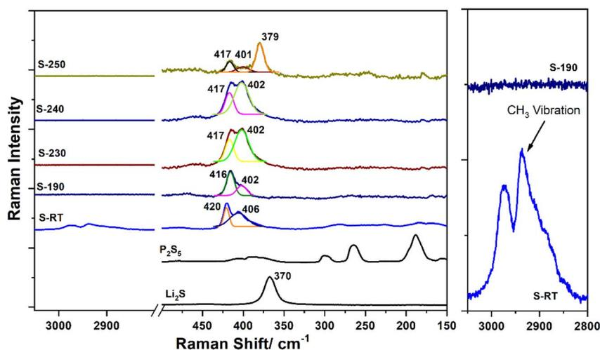
Fig. 3 Raman spectra of  $\text{Li}_2\text{S}$ ,  $\text{P}_2\text{S}_5$ , and the prepared samples S-RT, S-190, S-230, S-240, and S-250. The figure on the right-hand side shows the enlargement in the range of 3050 to  $2800\text{ cm}^{-1}$  of the spectra of S-RT and S-190.
