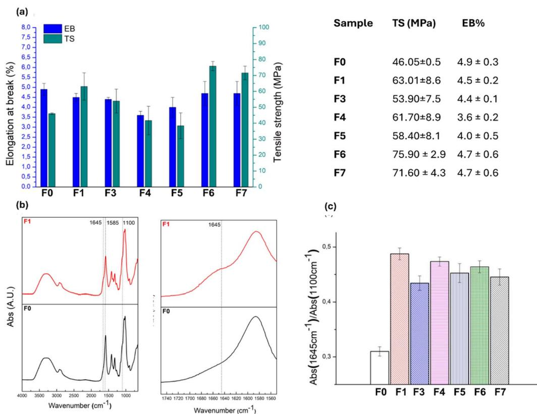
Fig. 4 (a) TS, EB of samples F0, F1, and F3–F7, (b) ATR-FTIR spectra of F1 (red line) and F0 (black line) films, and (c) Abs(1645 cm<sup>-1</sup>)/Abs(1100 cm<sup>-1</sup>) ratios for samples F0, F1, and F3–F7.
