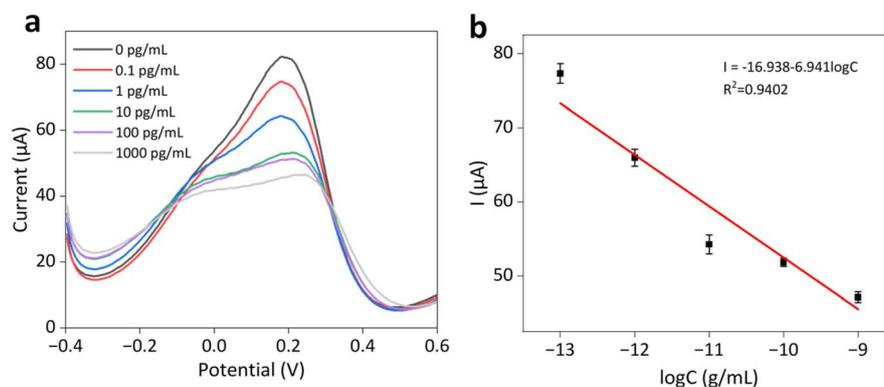
Fig. 7 RPB4 protein sensitivity detection data. (a) DPV curve under different RPB4 protein concentrations. (b) Relationship between the DPV peak current and RPB4 protein concentration after data processing, with the shaded area indicating the error margin.
