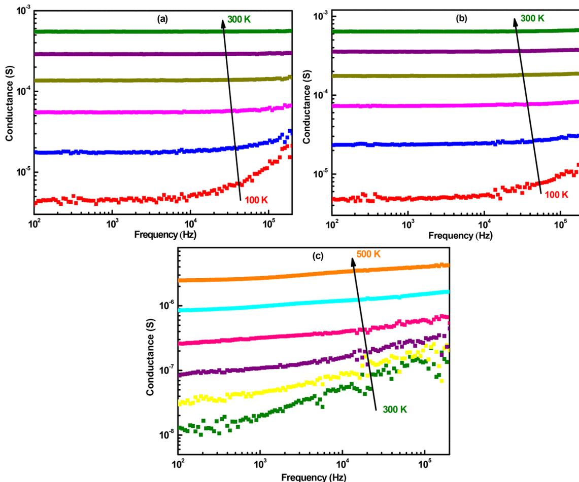
Fig. 9 ac conductance at different measurement temperatures with a step of 40 K for: (a): NPOM, (b): BHyNC and (c): THyNC.
