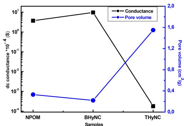
Fig. 10 Inverse variation of dc conductance and pore volume.
