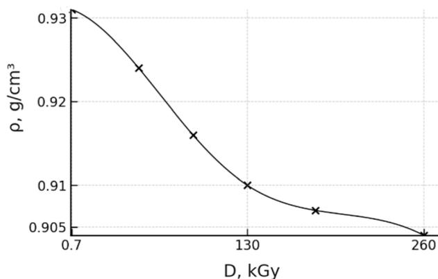
Fig. 7 Variation in density ( $\rho$ ,  $\text{g cm}^{-3}$ ) of immature crude oil from platform 14 as a function of gamma irradiation dose ( $D$ , kGy), indicating progressive transformation of arenes.
