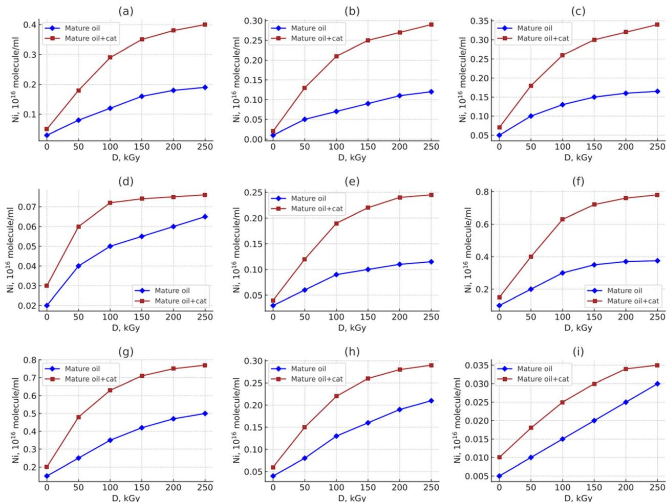
Fig. 3 Effect of irradiation dose ( $D$ , kGy) on the concentration ( $N_i$ ,  $10^{-16}$  molecules  $\text{mL}^{-1}$ ) of hydrocarbon gases formed during  $\gamma$ -radiolysis of mature crude oil samples, with and without Na-bentonite catalyst: (a)  $\text{CH}_4$ , (b)  $\text{C}_2\text{H}_6$ , (c)  $\text{C}_2\text{H}_4$ , (d)  $\sum\text{C}_3$ , (e)  $\sum\text{C}_4$ , (f)  $\sum\text{C}_5$ , (g)  $\sum\text{C}_6$ , (h)  $\sum\text{C}_7$ , (i)  $\sum\text{C}_8$ .
