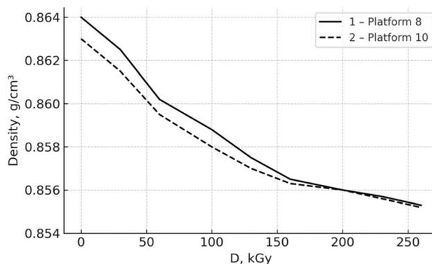
Fig. 11 Variation in density of mature crude oil samples under increasing gamma dose: 1 – platform 8; 2 – platform 10. The density decreases by  $\sim 1\%$ , indicating radiolytic fragmentation of aromatic structures.
