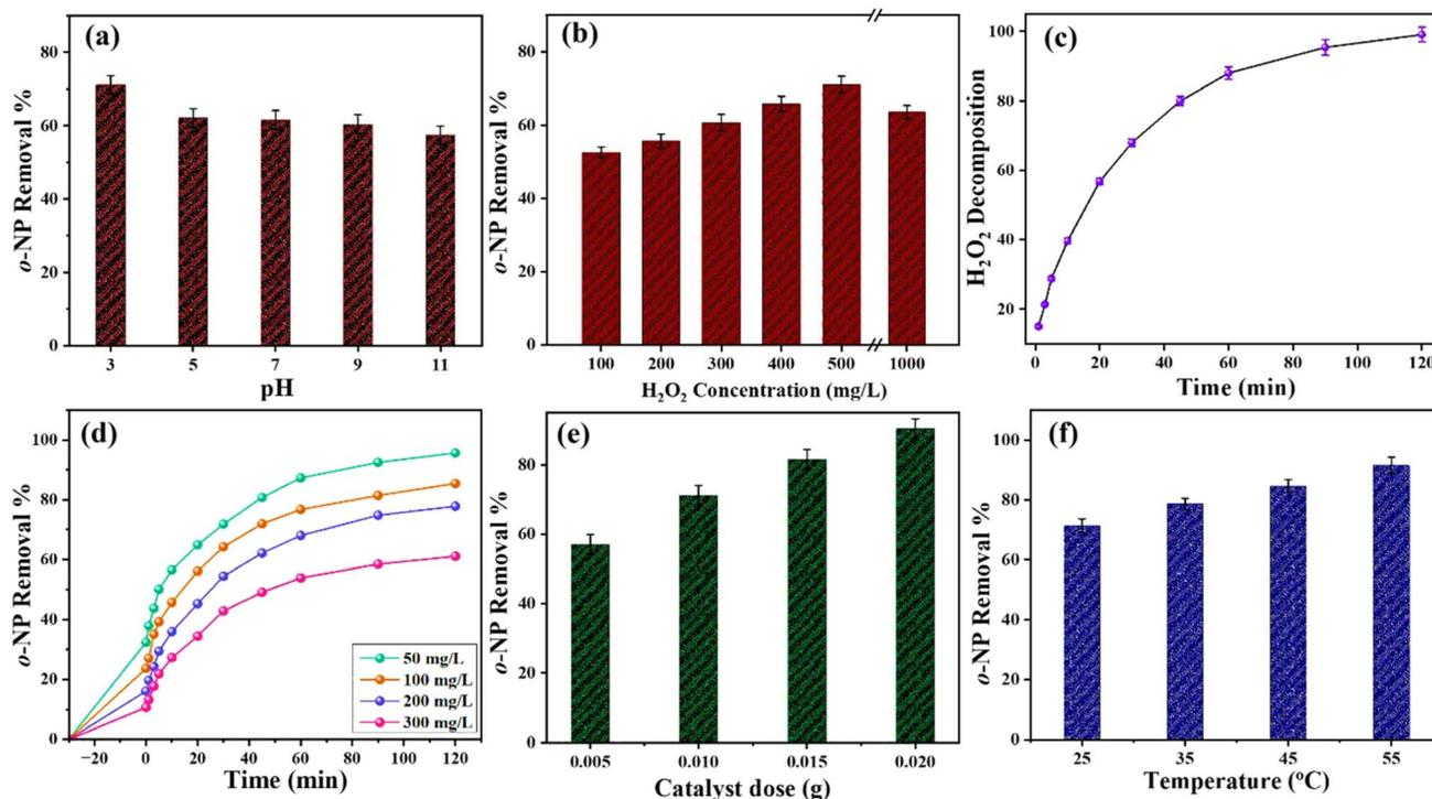
Fig. 4 The experimental findings from the investigation of the catalytic reaction parameters: (a) pH, (b)  $\text{H}_2\text{O}_2$  concentration, (c)  $\text{H}_2\text{O}_2$  degradation rate, (d) *o*-NP concentration, (e)  $\text{Ag}@Z\text{nFe}_2\text{O}_4/\text{BC}$  dosage, and (f) processing temperature.
