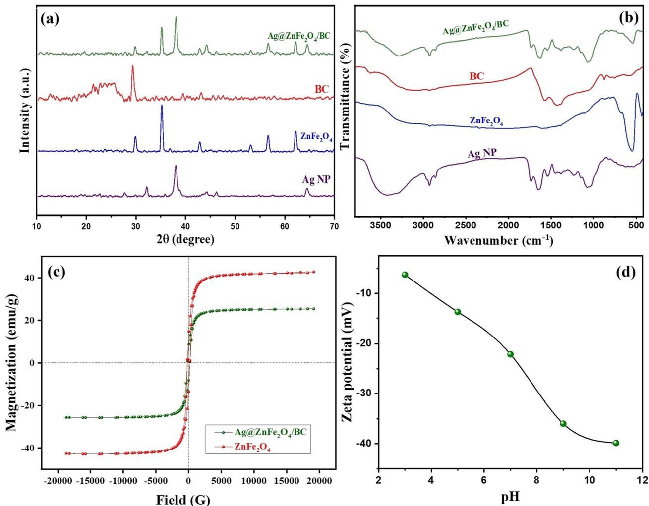
Fig. 1 (a) XRD patterns and (b) FTIR spectra of Ag, ZnFe<sub>2</sub>O<sub>4</sub>, BC, and Ag@ZnFe<sub>2</sub>O<sub>4</sub>/BC. (c) VSM hysteresis loop curves of ZnFe<sub>2</sub>O<sub>4</sub> and Ag@ZnFe<sub>2</sub>O<sub>4</sub>/BC. (d) Zeta potential curve of Ag@ZnFe<sub>2</sub>O<sub>4</sub>/BC.
