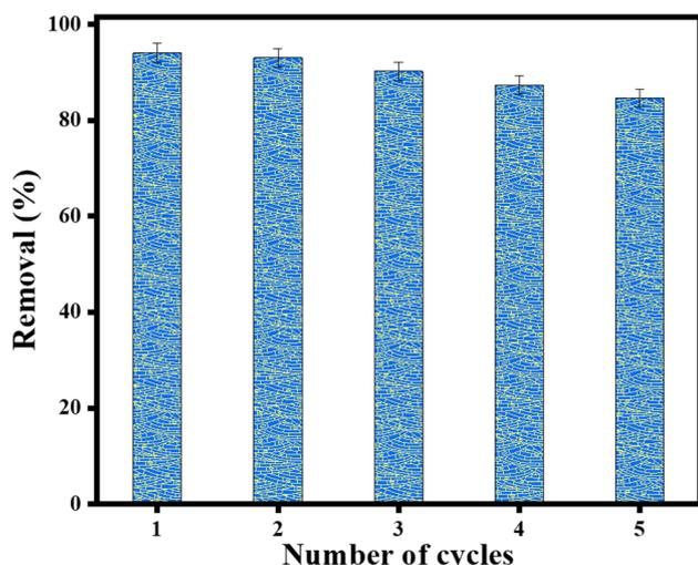
Fig. 8 Recycling study of Ag@ZnFe<sub>2</sub>O<sub>4</sub>/BC for five catalytic degradation runs of *o*-NP.
