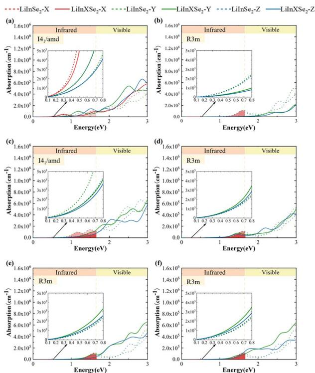
Fig. 5 Optical absorption spectra of all selected structures: (a) 50% Al-doped *I*<sub>41</sub>/*amd* phase; (b) 33% Al-doped *R3m* phase; (c) 50% Ga-doped *I*<sub>41</sub>/*amd* phase; (d) 33% Ga-doped *R3m* phase; (e) 33% Sb-doped *R3m* phase at site 1; (f) 33% Sb-doped *R3m* phase at site 2. The insets show magnified views of the 0.1–0.8 eV range.
