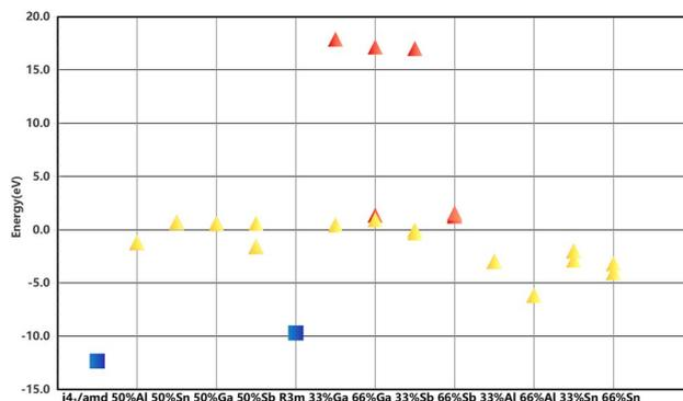
**Fig. 2** Formation energies of all structures are represented by scatter plots. Blue squares denote the two pristine structures, yellow triangles indicate configurations meeting the screening criteria, and red triangles represent those failing the criteria. Structures are grouped by space group ( $I4_1/amd$  and  $R3m$ ).
