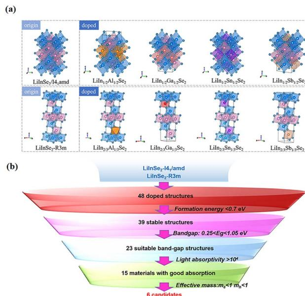
Fig. 1 (a) Structural models of  $\text{LiInSe}_2$  with space groups  $I4_1/amd$  and  $R3m$ , along with the corresponding doped structures incorporating Al/Ga/Sn/Sb elements. The models labeled as origin represent the pristine structures, while those labeled as doped correspond to the four doped configurations. (b) Screening process of the doped structures used in this work.
