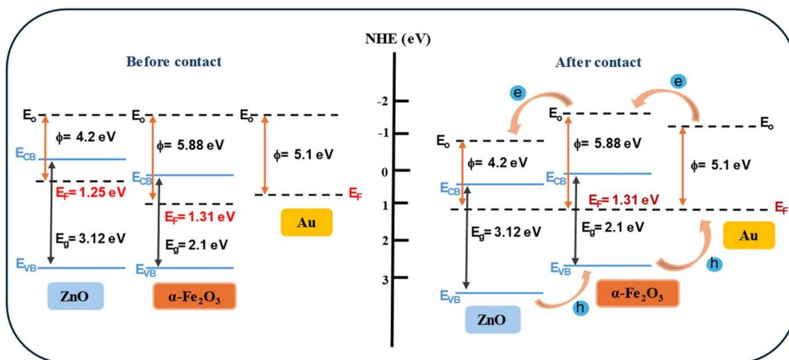
Fig. 9 Equilibrium energy band structure diagrams of the ZnO NRs/ $\alpha$ - $\text{Fe}_2\text{O}_3$  NPs/Au NPs composite before and after contact between the ZnO NRs,  $\alpha$ - $\text{Fe}_2\text{O}_3$  NPs and Au NPs.
