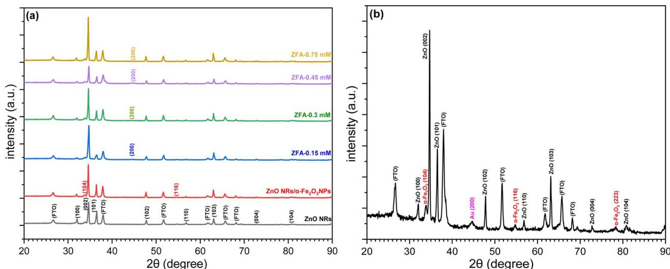
Fig. 4 XRD patterns of (a) ZnO NRs, ZnO NRs/ $\alpha$ -Fe<sub>2</sub>O<sub>3</sub> NPs with different concentrations of Au NPs (b) ZFA-0.45 mM.
