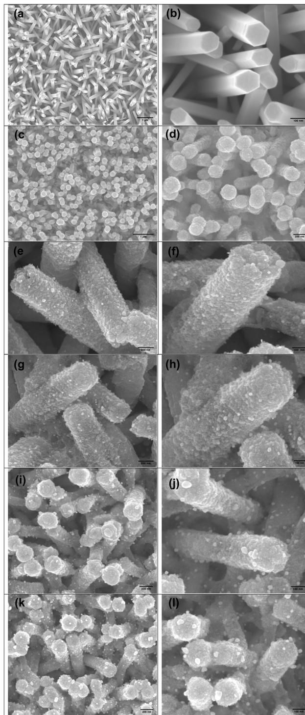
Fig. 2 SEM images of (a and b) ZnO NRs, (c and d) ZnO NRs/ $\alpha\text{-Fe}_2\text{O}_3$  NPs, and ZnO NRs/ $\alpha\text{-Fe}_2\text{O}_3$  NPs/Au NPs with different concentrations of  $\text{HAuCl}_4$ : (e and f) 0.15 mM, (g and h) 0.3 mM, (i and j) 0.45 mM, (k and l) 0.75 mM.
