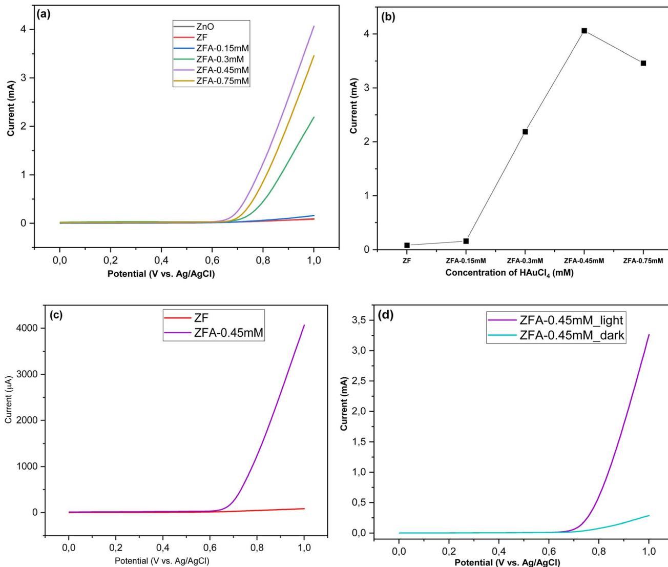
Fig. 6 (a) LSV responses of the ZnO NRs, ZnO NRs/ $\alpha$ -Fe<sub>2</sub>O<sub>3</sub> NPs and different concentrations of the Au NP electrode. (b) The corresponding linear calibration plots of the net current versus the Au NPs precursor. (c) LSV responses of ZF and ZFA-0.45 mM. (d) LSV responses of ZFA-0.45 mM under light and dark conditions.
