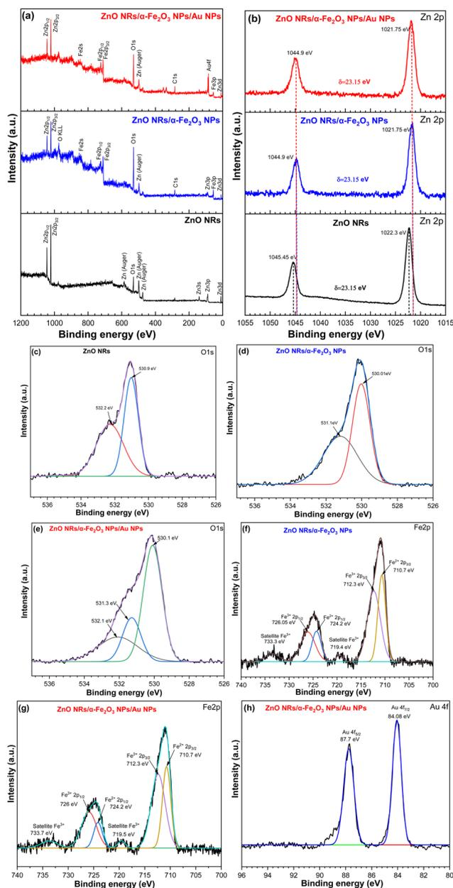
Fig. 5 XPS analysis. (a) The survey scan spectra of ZnONRs, ZnONRs/ $\alpha$ -Fe<sub>2</sub>O<sub>3</sub> NPs and ZnONRs/ $\alpha$ -Fe<sub>2</sub>O<sub>3</sub>NPs/AuNPs. The high-resolution spectra of ZnONRs, ZnONRs/ $\alpha$ -Fe<sub>2</sub>O<sub>3</sub> NPs and ZnONRs/ $\alpha$ -Fe<sub>2</sub>O<sub>3</sub>NPs/AuNPs: (b) Zn 2p, (c–e) O 1s, (f and g) Fe 2p and (h) Au 4f.
