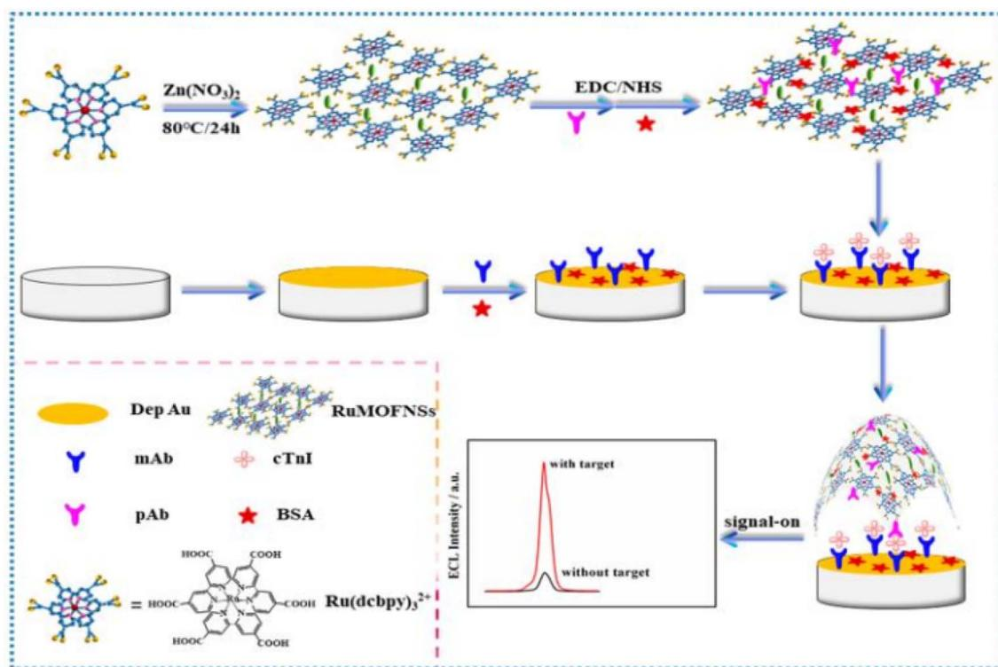
Fig. 11 Schematic fabrication process of the ECL immunosensor.
