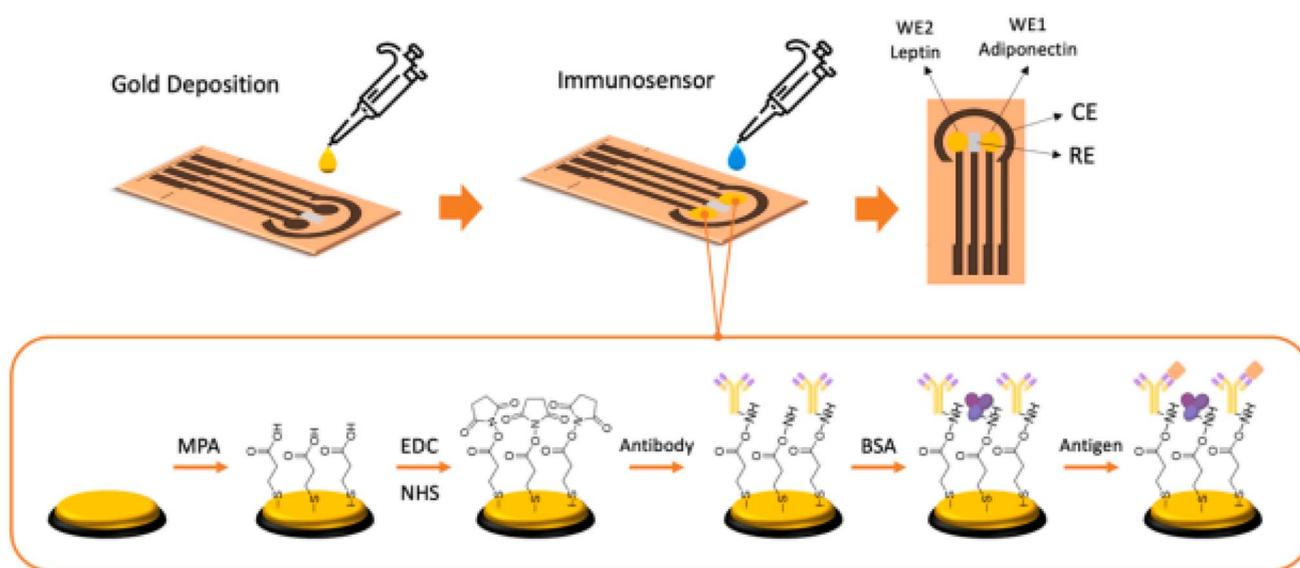
Fig. 8 Schematic illustration of the multiplexed electrochemical immunosensor fabrication process *via* EDC/NHS chemistry, enabling simultaneous detection of adiponectin and leptin biomarkers.
