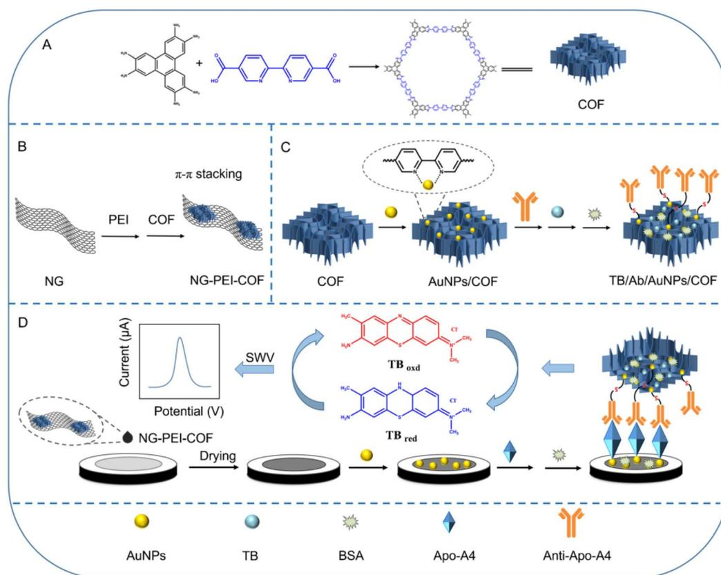
Fig. 10 Schematic diagram of the construction of a multi-signal amplification electrochemical immunosensor for Apo-A4 detection, preparation of COF (A), preparation of NG–PEI–COF composite (B), preparation of tracer probe (C), and detection process of the sensor (D).
