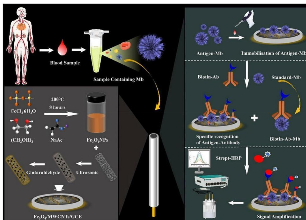
Fig. 4 Diagram of construction of HRP–Strept–Biotin–Ab–Mb/Mb/Fe<sub>3</sub>O<sub>4</sub>–MWCNTs–COOH/GCE electrochemical immunosensor.
