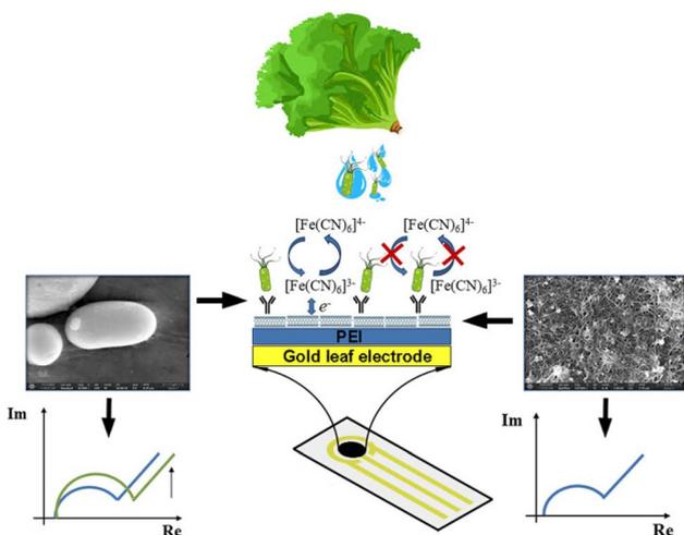
Fig. 2 Schematic layer-by-layer (LbL) procedure and functionalization steps.
