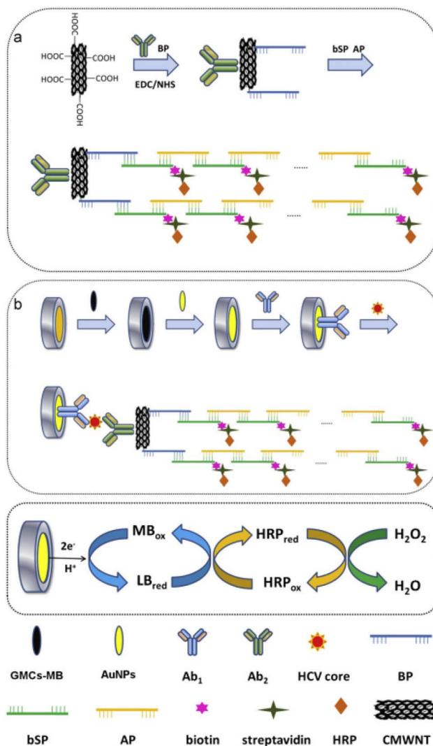
Fig. 3 (a) Preparation of the multi-HRP–DNA–CMWNTs–Ab<sub>2</sub> bi-conjugate, demonstrating the hierarchical assembly of horseradish peroxidase (HRP) enzymes, DNA linkers, carboxylated multi-walled carbon nanotubes (CMWNTs), and secondary antibodies (Ab<sub>2</sub>) for signal amplification and (b) fabrication process of the hepatitis C virus (HCV) immunosensor, highlighting key steps in electrode modification, immunocomplex formation, and electrochemical signal transduction.
