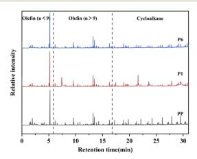
Fig. 8 Py-GCMS spectrum of PP, P1, and P6.
