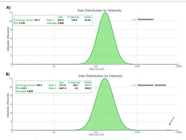
Fig. 3 Dynamic light scattering (DLS) size distribution profiles of nanoemulsion formulations. (A) Size distribution of plain nanoemulsion showing Z-average diameter of 195.7 nm with PDI of 0.342  $\pm$  0.02 and primary population (92.92% by intensity) centered at 205.6 nm. (B) Size distribution of amoxicillin-conjugated nanoemulsion exhibiting hydrodynamic diameter of 199.6 nm with improved PDI of  $0.331 \pm 0.01$ , demonstrating enhanced size uniformity upon drug loading
