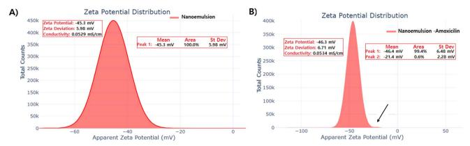
Fig. 2 Zeta potential analysis of nanoemulsion formulations. (A) Zeta potential distribution of plain nanoemulsion showing surface potential of -45.3 ± 5.98 mV with 100% population homogeneity. (B) Zeta potential distribution of amoxicillin-conjugated nanoemulsion demonstrating enhanced surface charge of  $-46.3 \pm 6.71$  mV with 99.4% of particles maintaining the primary peak at -46.4 mV, indicating excellent colloidal stability and electrostatic repulsion
