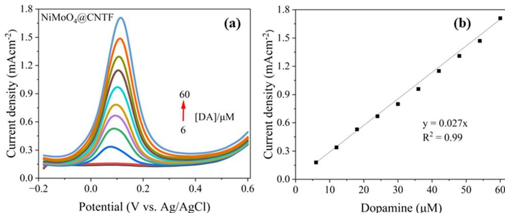
Fig. 10 (a) SWV curve of the NiMoO<sub>4</sub>@CNTF electrode for different concentrations of DA in 0.1 M (KH<sub>2</sub>PO<sub>4</sub>, K<sub>2</sub>HPO<sub>4</sub>, pH 8) and (b) its calibration curve.
