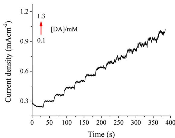
Fig. 11 Staircase chronoamperometry response of the NiMoO<sub>4</sub>@CNTF electrode to DA at various concentrations in the range of 0.1–1.3 mM.
