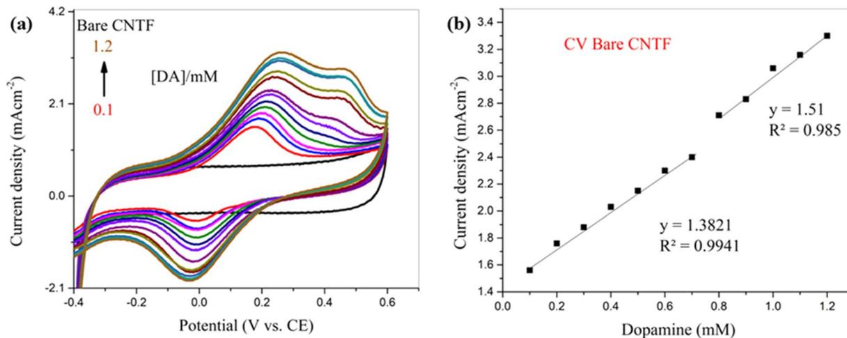
Fig. 6 (a) CV curve of the bare CNT fiber electrode with different concentrations of DA at a fixed scan rate of 0.10 V s<sup>-1</sup> in 0.1 M (KH<sub>2</sub>PO<sub>4</sub>, K<sub>2</sub>HPO<sub>4</sub>, pH 8) and (b) its calibration curve.
