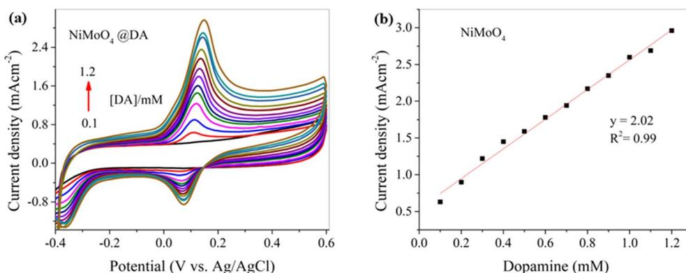
Fig. 5 (a) CV curve of the NiMoO<sub>4</sub>@CNTF electrode for different concentrations of DA at a fixed scan rate of 0.10 V s<sup>-1</sup> in 0.1 M (KH<sub>2</sub>PO<sub>4</sub>, K<sub>2</sub>HPO<sub>4</sub>, pH 8) and (b) its calibration curve.
