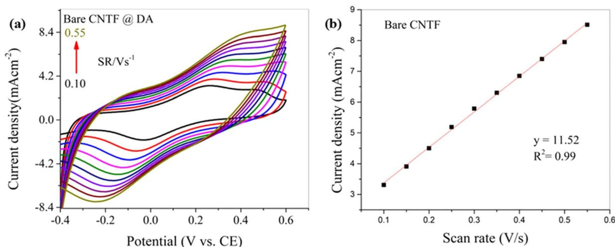
Fig. 9 (a) CV curve for DA detection on the bare CNTF electrode at various scan rates (0.10 to 0.55 V s<sup>-1</sup>) and (b) corresponding calibration curve of current density vs. scan rate.
