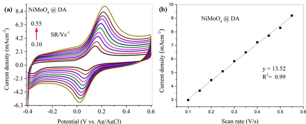
Fig. 8 (a) CV curve for DA detection on the NiMoO<sub>4</sub>@CNTF modified electrode at various scan rates (0.10 to 0.55 V s<sup>-1</sup>) and (b) corresponding calibration curve of current density vs. scan rate.
