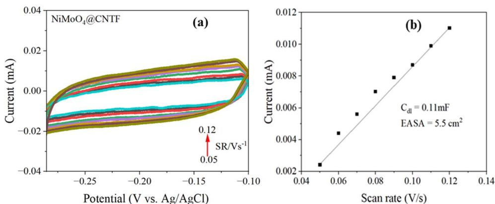
Fig. 7 (a) Non-faradaic CV curves of NiMoO<sub>4</sub>@CNTF at increasing scan rates and (b) corresponding plot of capacitive current density versus scan rate.
