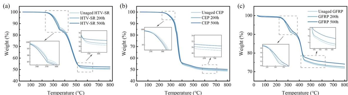
**Fig. 10** TGA curves of three samples before and after corona aging. (a) HTV-SR; (b) CEP; (c) GFRP.
