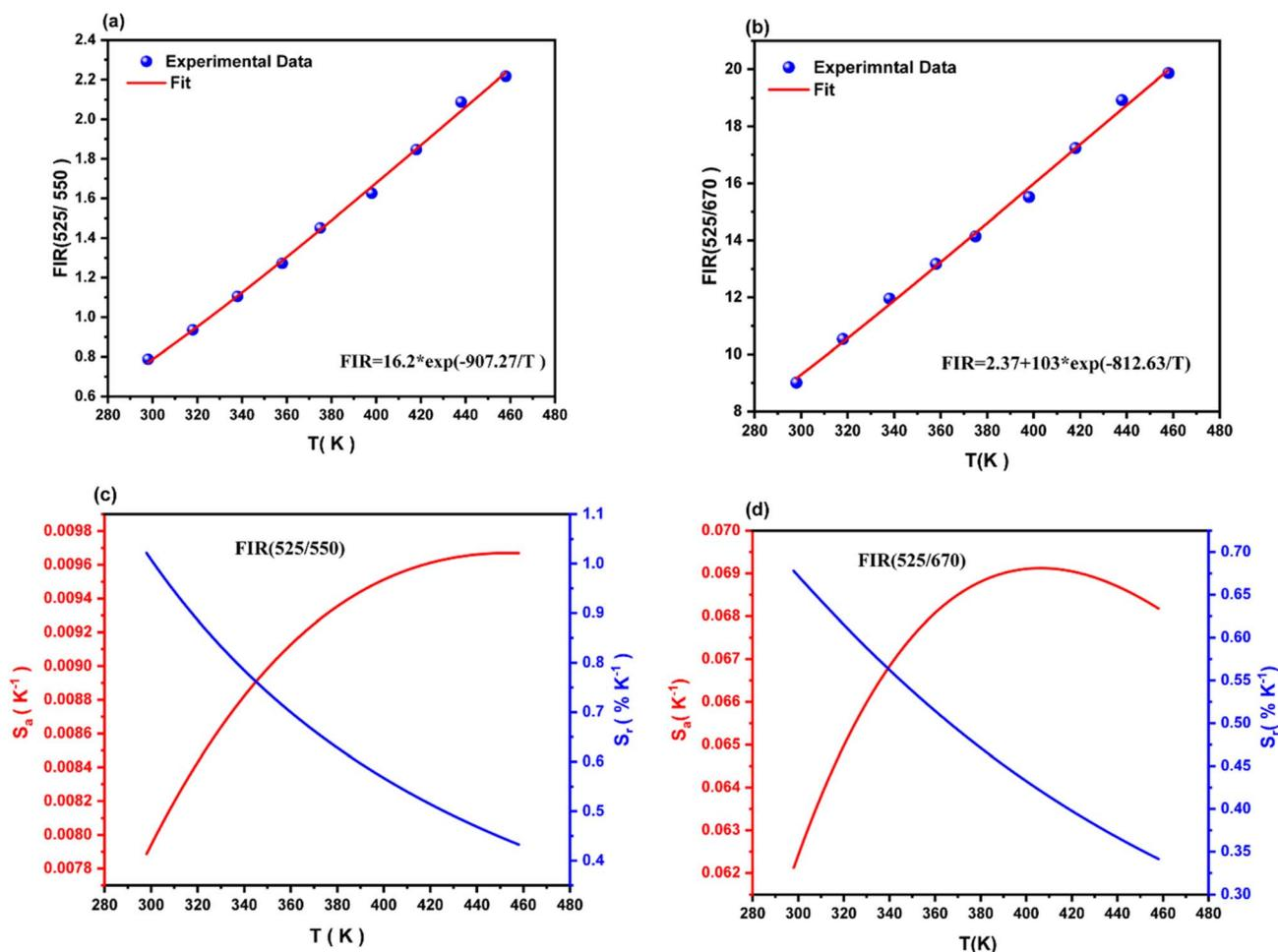
Fig. 8 (a) and (b) FIR variation with temperature. (c) and (d) Absolute sensitivity and relative sensitivity of TCLs ( $I_{525}/I_{550}$ ), NTCLs ( $I_{525}/I_{670}$ ), respectively for  $\text{LCLMO}:0.02 \text{ Er}^{3+}/0.15 \text{ Yb}^{3+}$  under 980 nm excitation.
