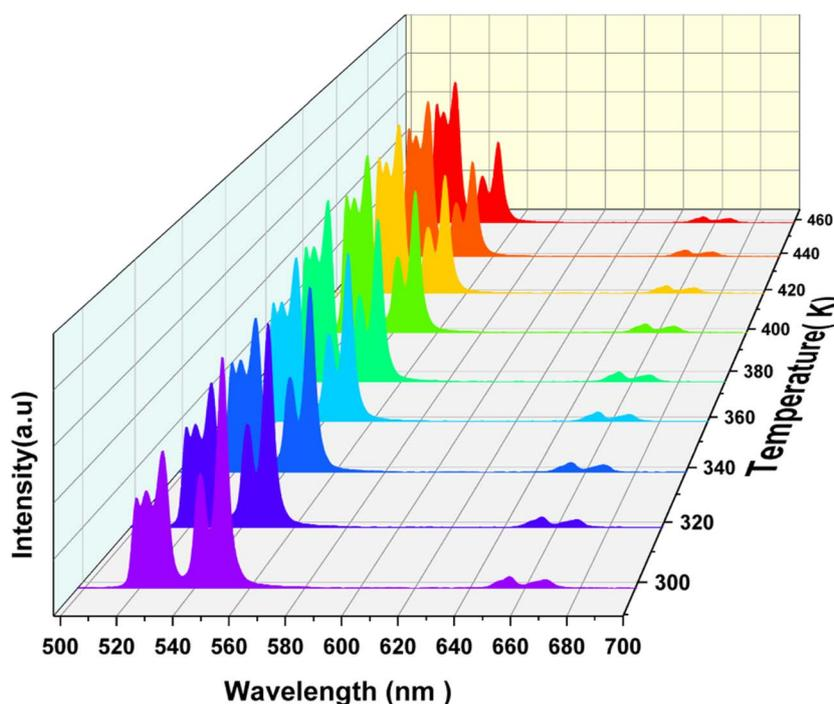
Fig. 7 Temperature dependent UC emission spectra of LCLMO:0.02 Er<sup>3+</sup>/0.15 Yb<sup>3+</sup> under 980 nm excitation.
