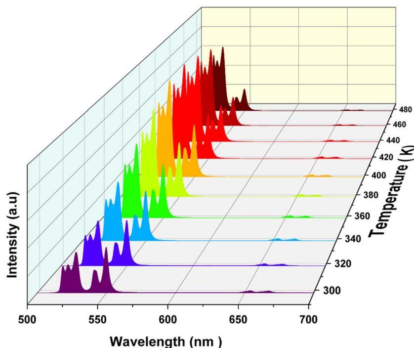
Fig. 4 Temperature dependent down-converted photoluminescence emission spectra of LCLMO:0.02 Er<sup>3+</sup>/0.15 Yb<sup>3+</sup> under 325 nm excitation.
