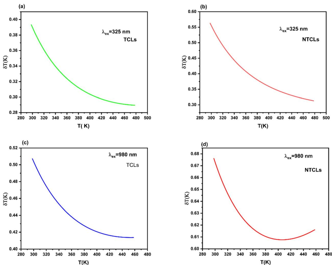
Fig. 9 Temperature uncertainty of LCLMO:Er<sup>3+</sup>/Yb<sup>3+</sup>: (a)  $\delta T$  (525/550) nm (down-conversion), (b)  $\delta T$  (525/670) nm (down-conversion), (c)  $\delta T$  (525/550) nm (UP-conversion), (d)  $\delta T$  (525/670) nm (UP-conversion).
