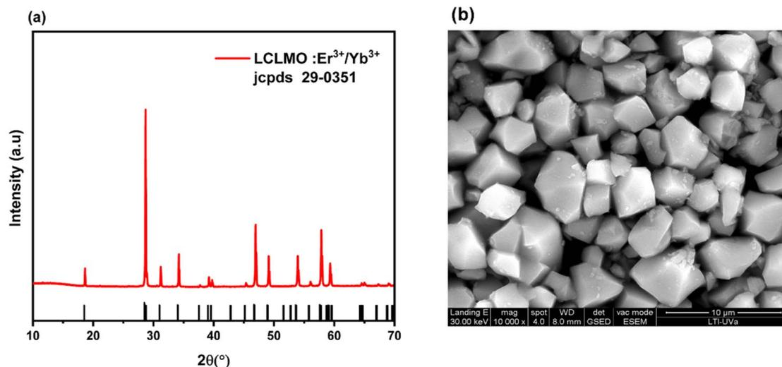
Fig. 1 (a) X-ray powder diffraction patterns, (b) SEM of LCLMO:Er<sup>3+</sup>/Yb<sup>3+</sup>.
