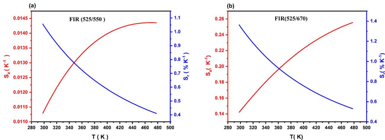
Fig. 6 Absolute sensitivity and relative sensitivity (a) TCL, (b) NTCL for LCLMO:0.02 Er<sup>3+</sup>/0.15 Yb<sup>3+</sup>.
