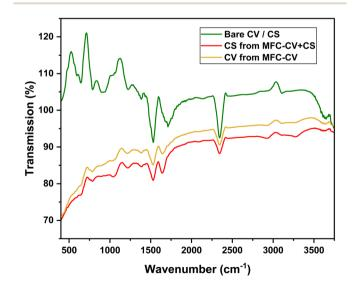
Fig. 9 FTIR spectra of the carbon veil electrode (bare, before experiments) and the electrode after operation in MFC-CV and MFC-CV + CS.
