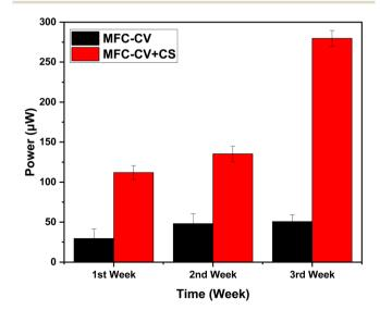
Fig. 4 Power output from triplicate MFC-CV and MFC-CV + CS sets over 3 weeks under non-optimized load.
