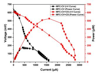
Fig. 6 Polarisation carried out at the 5th week of operation in MFC-CV and MFC-CV + CS.
