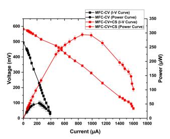
Fig. 5 Polarisation carried out at the 3rd week of operation in MFC-CV and MFC-CV + CS.
