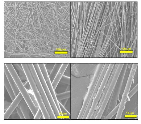
Fig. 2 SEM images of electrodes after operation in MFCs at two different magnifications. Left: carbon veil as a single electrode; right: carbon sleeve in combination with carbon veil.
