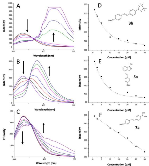
Fig. 2 (A–C) Fluorescence spectra ( $\lambda_{\text{ex}} = 270$  nm) of HSA were recorded in the presence of the compounds at concentrations ranging from 1 to 30  $\mu\text{M}$ , prepared in a solution of 10% v/v DMSO in water and Tris–HCl buffer (pH = 7.4). (D–F) The fluorescence decay pattern of HSA at 330 nm was analysed as a function of increasing compound concentrations.
