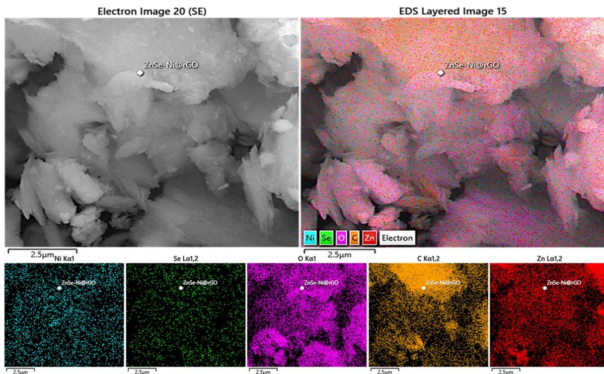
Fig. 5 Elemental mapping of Zn<sub>0.90</sub>Ni<sub>0.10</sub>Se/rGO.
