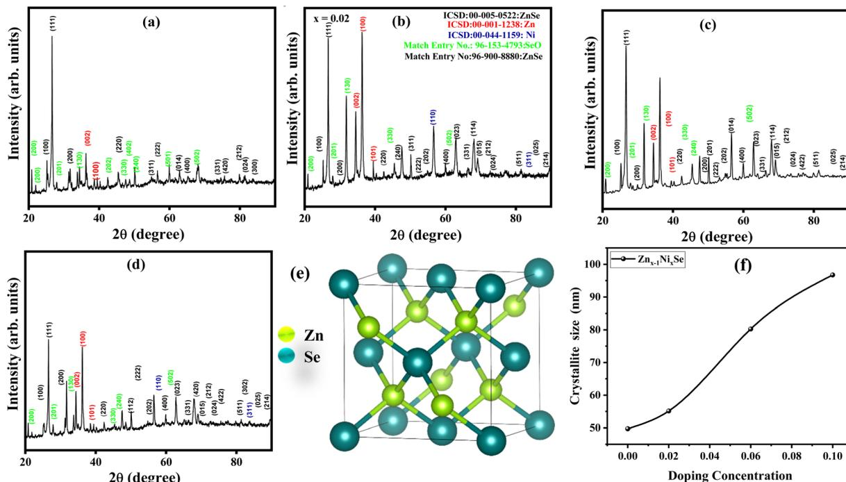
Fig. 2 (a) XRD patterns of ZnSe, (b) Zn<sub>0.90</sub>Ni<sub>0.10</sub>Se, (c) ZnSe/rGO, and (d) Zn<sub>0.90</sub>Ni<sub>0.10</sub>Se/rGO. (e) Crystal structure of ZnSe. (f) Crystallite size vs. different doping percentages.
