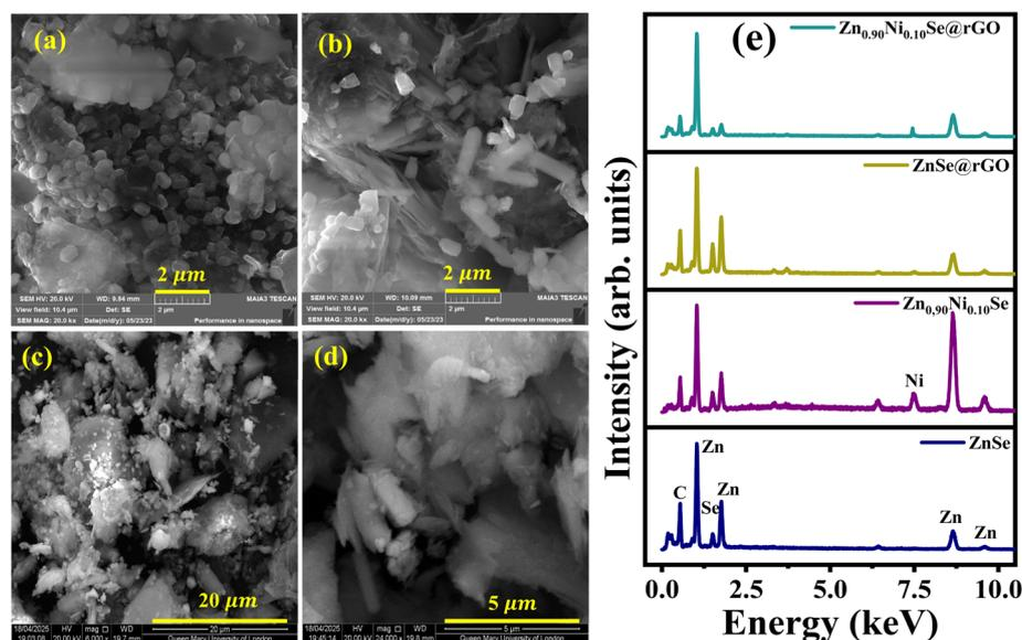
Fig. 3 (a–d) SEM images of ZnSe, Zn<sub>0.90</sub>Ni<sub>0.10</sub>Se, ZnSe/rGO, and Zn<sub>0.90</sub>Ni<sub>0.10</sub>Se/rGO. (e) EDX spectra of all samples.
