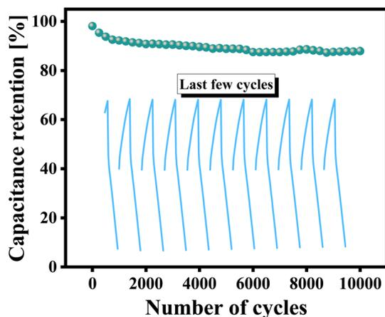
Fig. 10 Cyclic stability test of Zn<sub>0.90</sub>Ni<sub>0.10</sub>Se/rGO.
