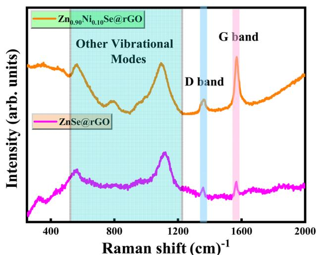
Fig. 6 Raman analysis of ZnSe/rGO and  $\text{Zn}_{0.90}\text{Ni}_{0.10}\text{Se}/\text{rGO}$ .
