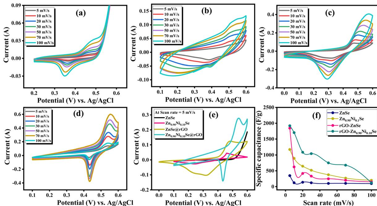
Fig. 7 CV curves at different scan rates for (a) ZnSe, (b)  $\text{Zn}_{0.90}\text{Ni}_{0.10}\text{Se}$ , (c) ZnSe/rGO, and (d)  $\text{Zn}_{0.90}\text{Ni}_{0.10}\text{Se}/\text{rGO}$ . (e) Combined CV curves at  $5 \text{ mV s}^{-1}$ , and (f) scan rate vs. specific capacitance.
